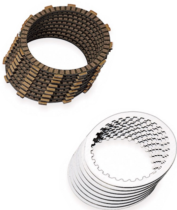
F. SCREAMIN' EAGLE PERFORMANCE CLUTCH FRICTION DISC KIT
