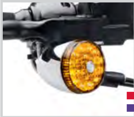
C. LED BULLET TURN SIGNAL KIT – AMBER LENS
