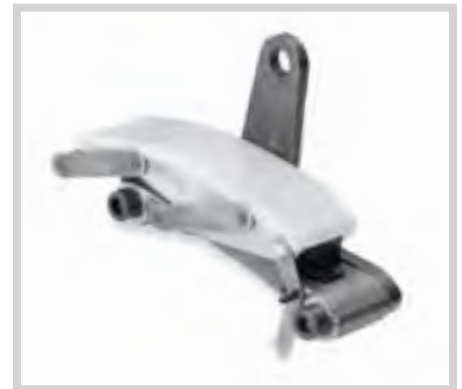
C. AUTOMATIC PRIMARY CHAIN TENSION ADJUSTER
