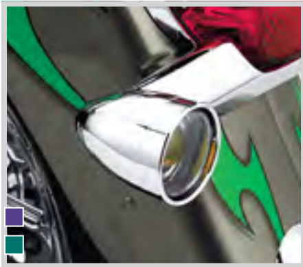
B. BULLET STYLE TURN SIGNAL KIT – REAR SMOKED LENS
