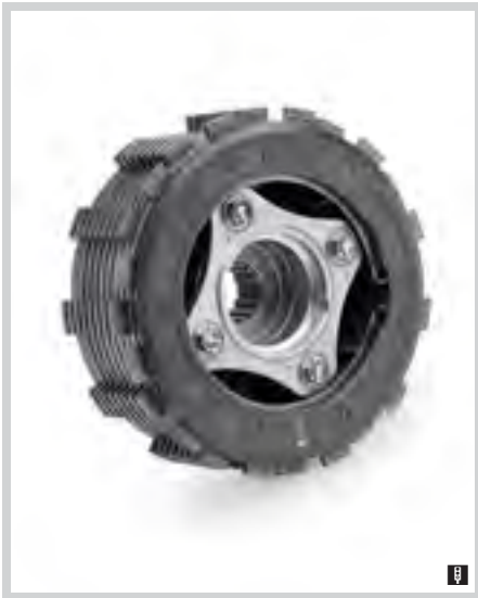
H. SCREAMIN' EAGLE PERFORMANCE SLIPPER CLUTCH FOR VRSC MODELS
