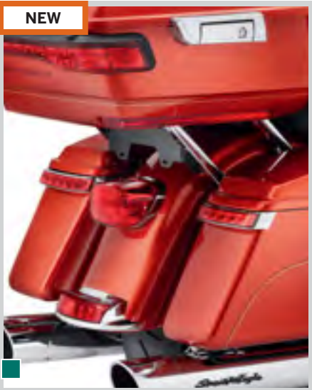
A. ELECTRA GLO LED SADDLEBAG RUN/BRAKE/TURN LAMP – RED LENS
