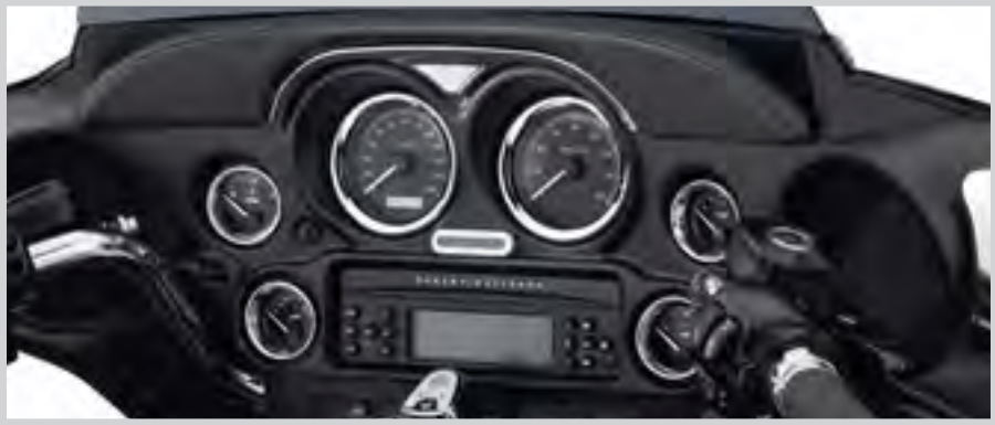
D. CHROME INSTRUMENT BEZELS (SHOWN WITH FAIRING DASH PAD)
