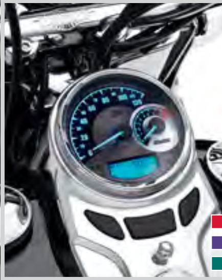
A. COMBINATION ANALOG SPEEDOMETER/TACHOMETER – 5" SPUN ALUMINUM DIAL
