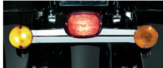
Turn Signal Flashes Amber. Taillight Remains Illuminated
