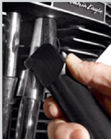
F. SCREAMIN' EAGLE PUSHROD TUBE INSTALLATION AND REMOVAL TOOL
