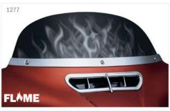
AIRMASTER® GRAPHIC WINDSHIELDS FOR BATWING FAIRING Airmaster® graphic windshields are 7" tall and manufactured from premium hard-coated polycarbonate that will not crack or shatter upon impact, unlike acrylic. Graphics are screen printed behind a light smoke material with proprietary inks, making the images unbelievably sharp and durable.
