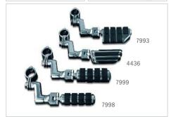
**TOUR-TECH™ CRUISE MOUNTS** FOR 1-1/4" ENGINE GUARDS Short Arm Mounts place the peg 4" back from the bar for taller riders, while the Long Arms are 6" back for shorter riders. The arm and footpeg may be further adjusted along a vertical or horizontal arc. A unique clevis permits angle adjustment of the footpeg. The heavy-duty Quick Clamp and sturdy offset arm ensures that the footpegs will clear fairing lowers and will stay where you put them.
