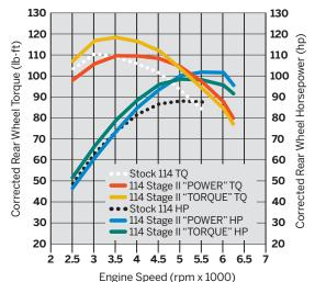
\*\* FLHXSE 114 Stage II "POWER" with Ventilator A/C & Street Cannon Mufflers
