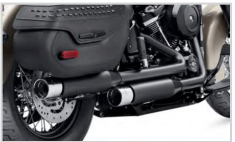
C. SATIN BLACK MUFFLER SHIELDS – SHORT (SHOWN ON FLHC MODEL WITH SATIN BLACK EXHAUST SHIELDS)
