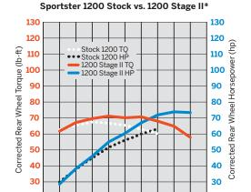
Engine Speed (rpm x 1000) \*14-later XL1200 Stage II with Heavy Breather A/C & Street Cannon Mufflers
