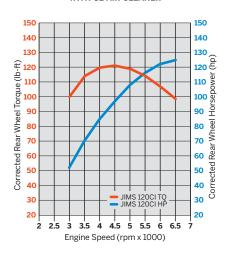
Corrected torque and horsepower measured at the rear wheel on a chassis dynamometer. Your results may vary.
