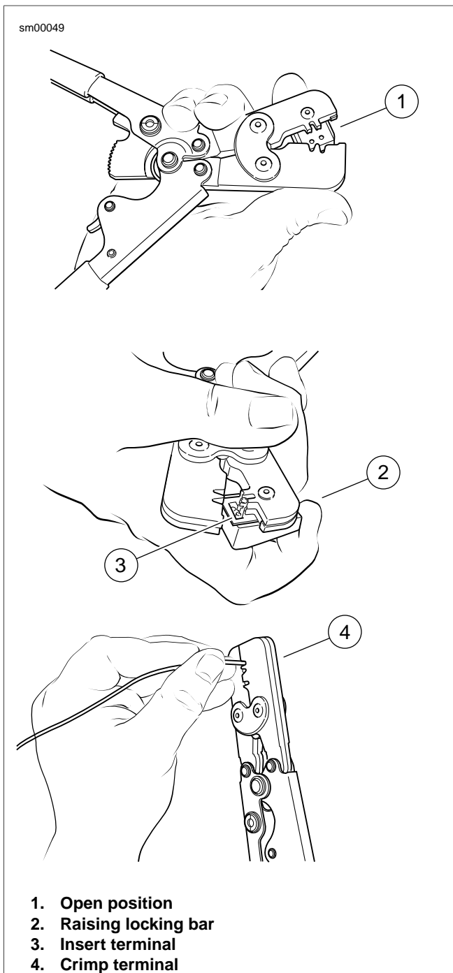
Figure A-22. Delphi Micro-64 Sealed Connector: Terminal in Crimper
