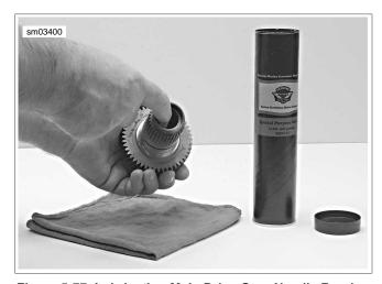
Figure 5-77. Lubricating Main Drive Gear Needle Bearing
