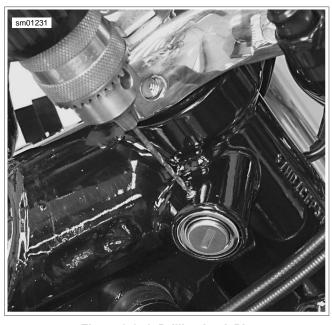
Figure 2-241. Drilling Lock Pin
