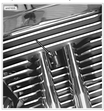
Figure 4-26. ET Sensor Location
