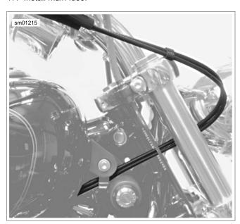
Figure 2-177. Throttle Control Cable Routing: XL Models
