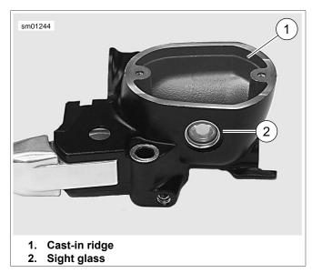
Figure 2-74. Filling Front Master Cylinder Reservoir
