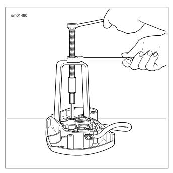
Figure 3-115. Removing Cam Bushing from Gearcase Cover
