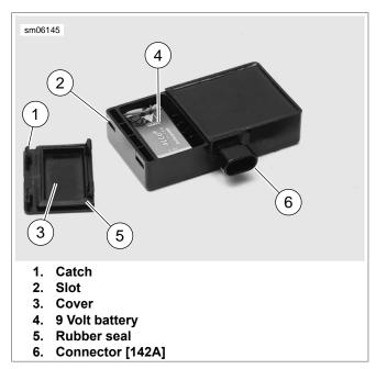
Figure 6-130. Siren Battery Compartment
