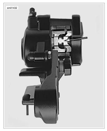
Figure 2-108. Rear Caliper Pad Spring
