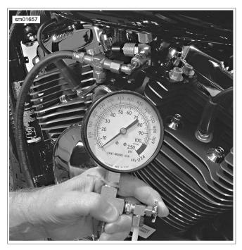
Figure 4-83. Fuel Pressure Gauge Installed: All Models
