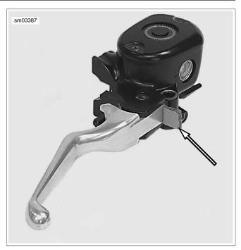
Figure 6-138. Install Cardboard Insert
