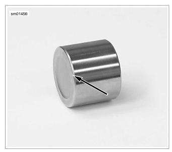
Figure 2-107. Piston Nose Radius
