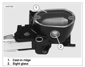
Figure 1-58. Filling Front Master Cylinder Reservoir (typical)
