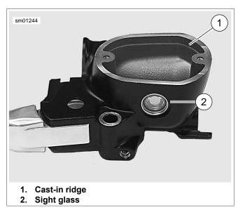
Figure 2-60. Filling Front Master Cylinder Reservoir
