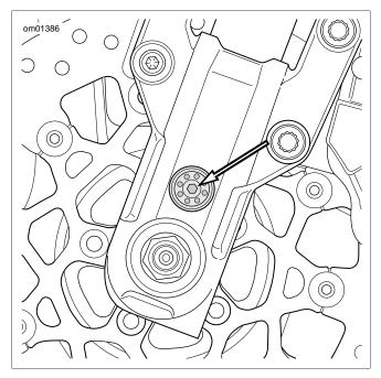
Figure 1-79. Spring Preload Adjuster: XR 1200X
