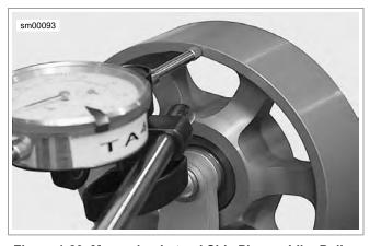
Figure 1-29. Measuring Lateral Side Play on Idler Pulley
