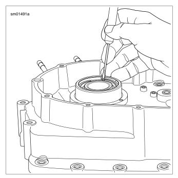
Figure 3-122. Removing Left Main Oil Seal Retaining Ring
