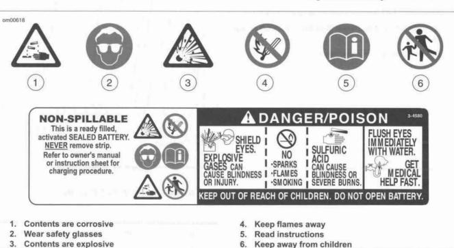
Figure 1-42. Battery Warning Label
