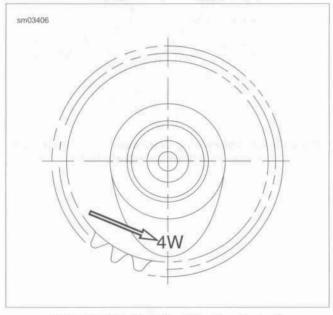
Figure 3-121. Cam Identification (typical)
