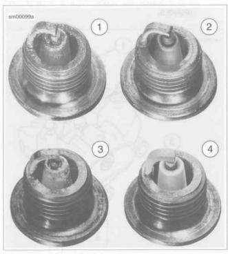
Figure 1-36. Spark Plug Deposits
