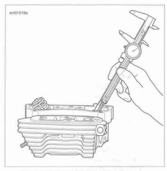
Figure 3-32. Measuring Valve Stem Protrusion
