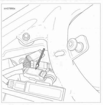
Figure 6-48. License Plate Lamp Connector [40]
