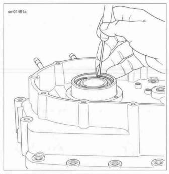
Figure 3-93. Removing Left Main Oil Seal Retaining Ring
