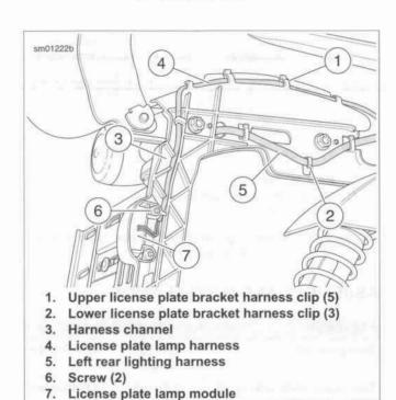
Figure 2-168. Removing/Installing License Plate Lamp Module (U.S.)
