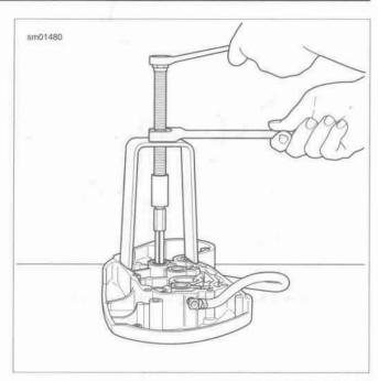
Figure 3-86. Removing Cam Bushing from Gearcase Cover
