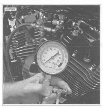
Figure 4-48. Fuel Pressure Gauge Installed: All Models
