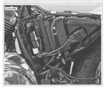
Figure 6-105. Under Seat Routing
