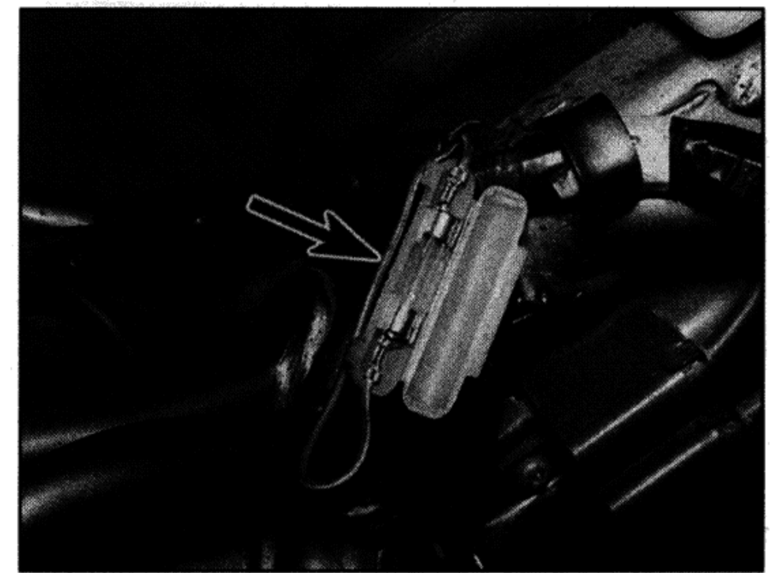
5.1c Cooling fan fuse – XTZ models
