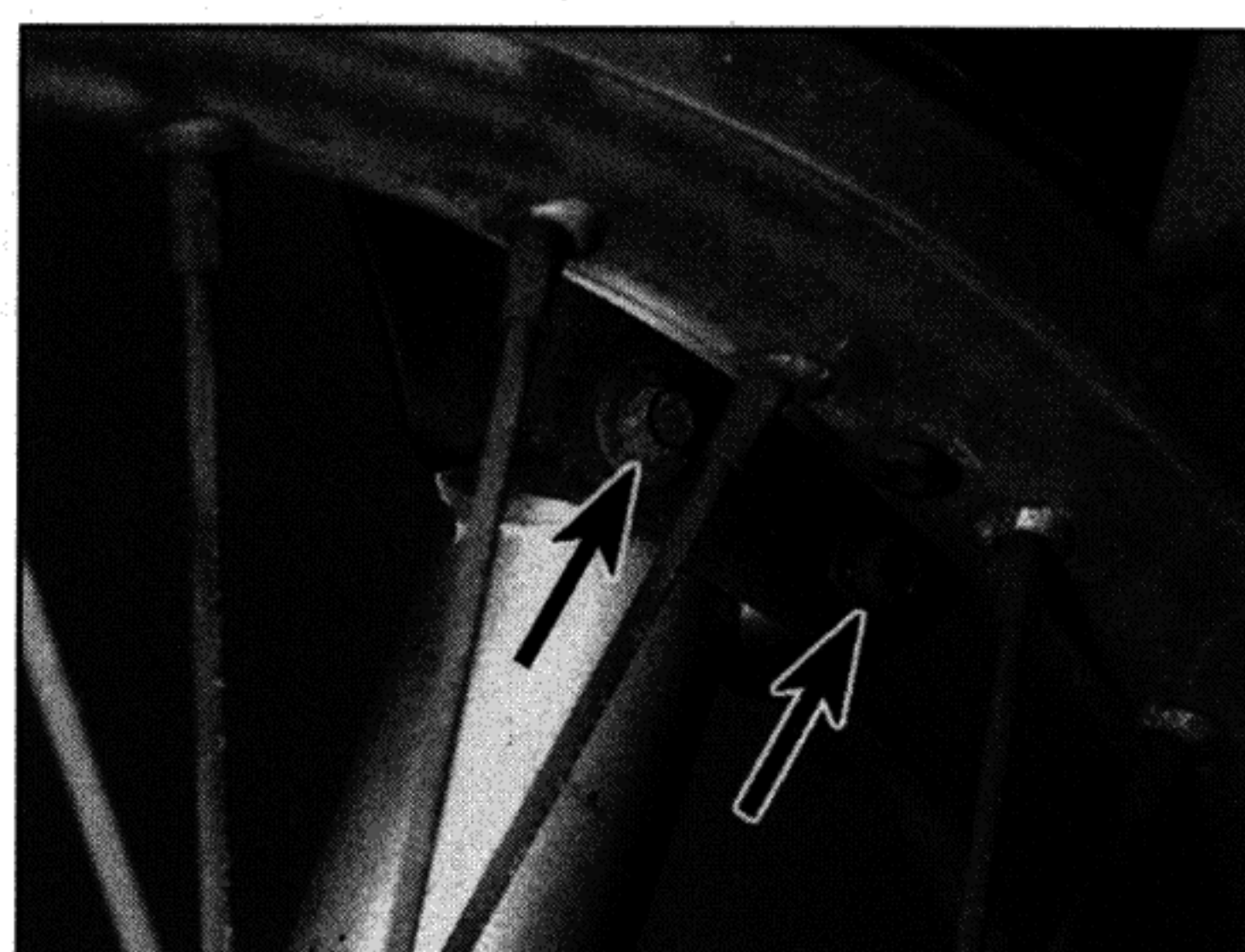
6.2c On XTZ models, the bolts (arrowed) are on the inside of the fork leg
