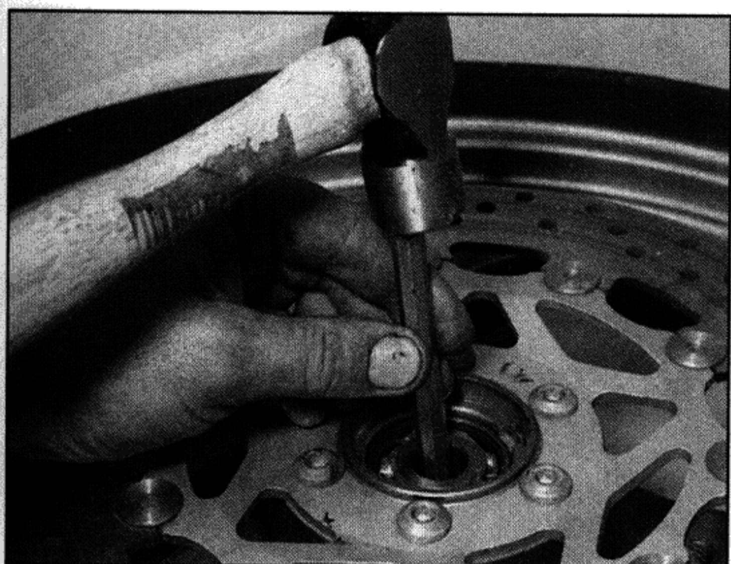
13.5a Knock out the bearings using a drift ...
