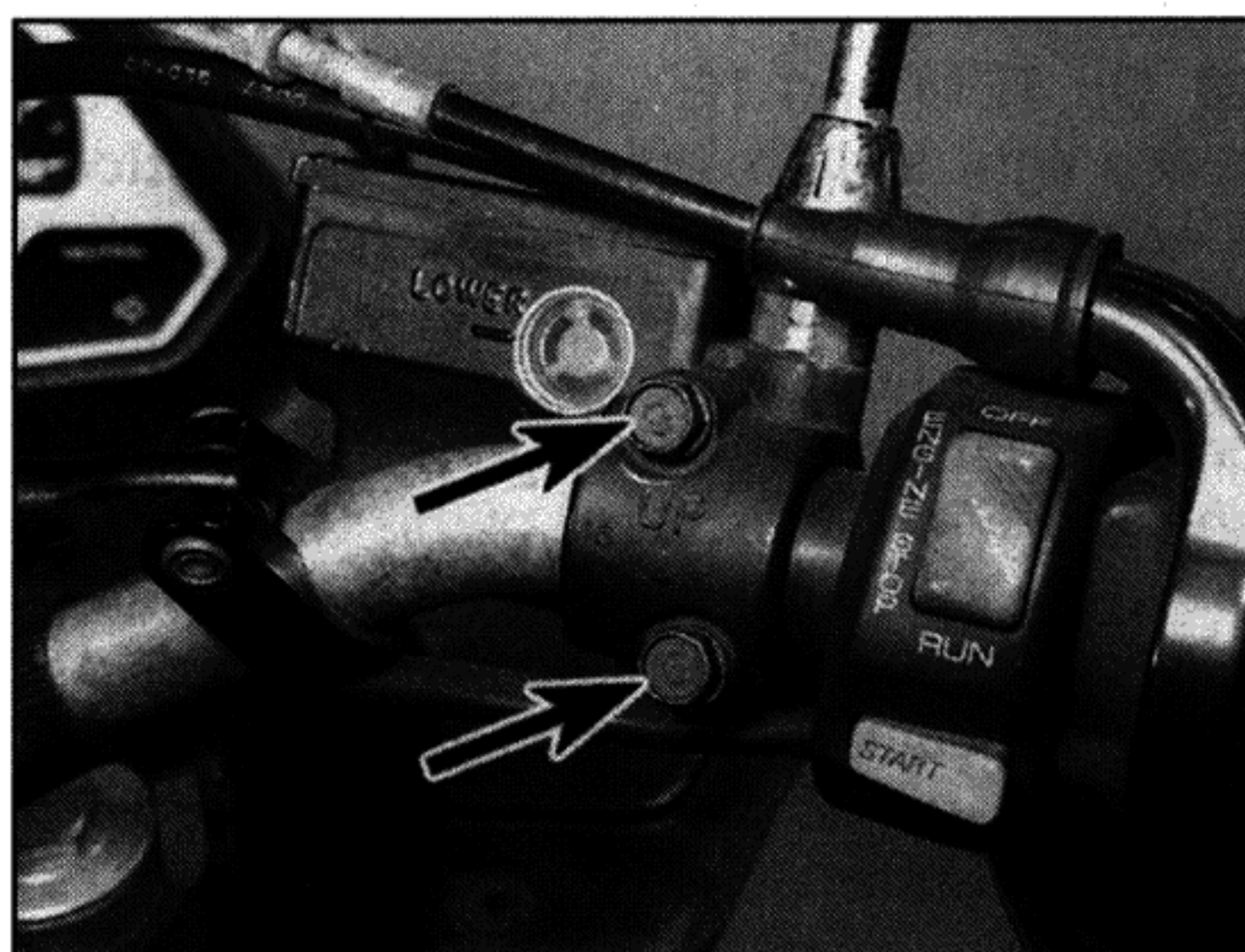
5.8b Master cylinder clamp bolts (arrowed) – XTZ models
