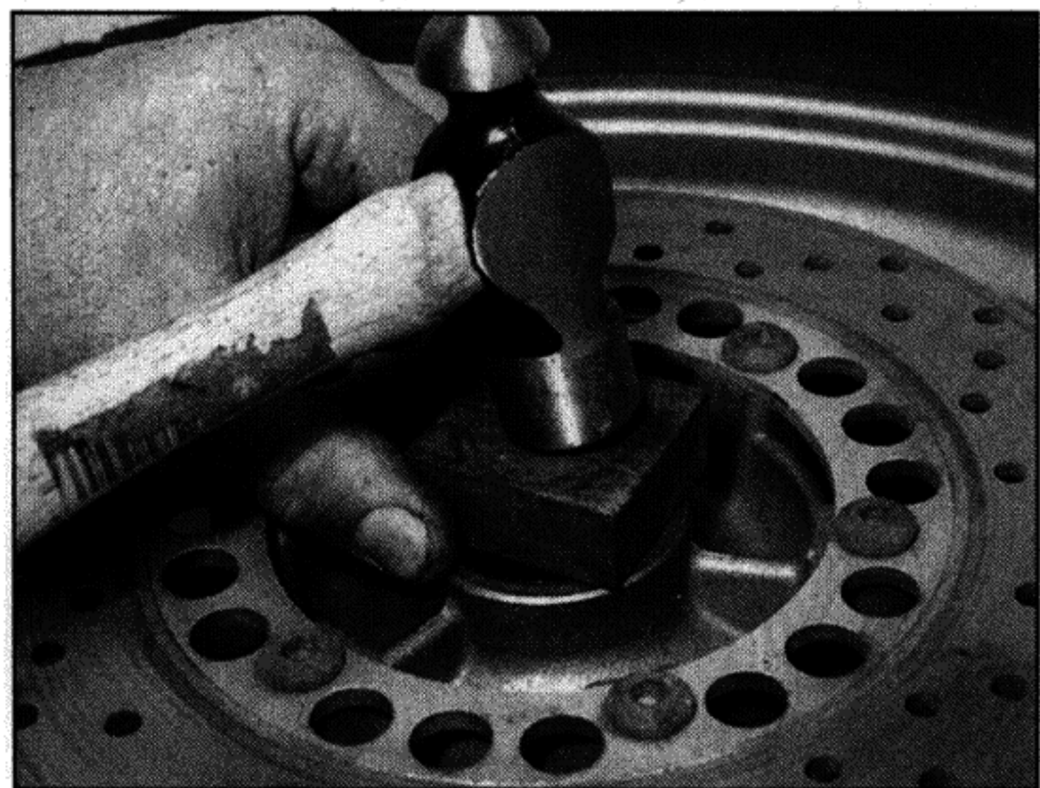
13.23 Where the seal sits flush with the rim, a piece of wood can be used as shown
