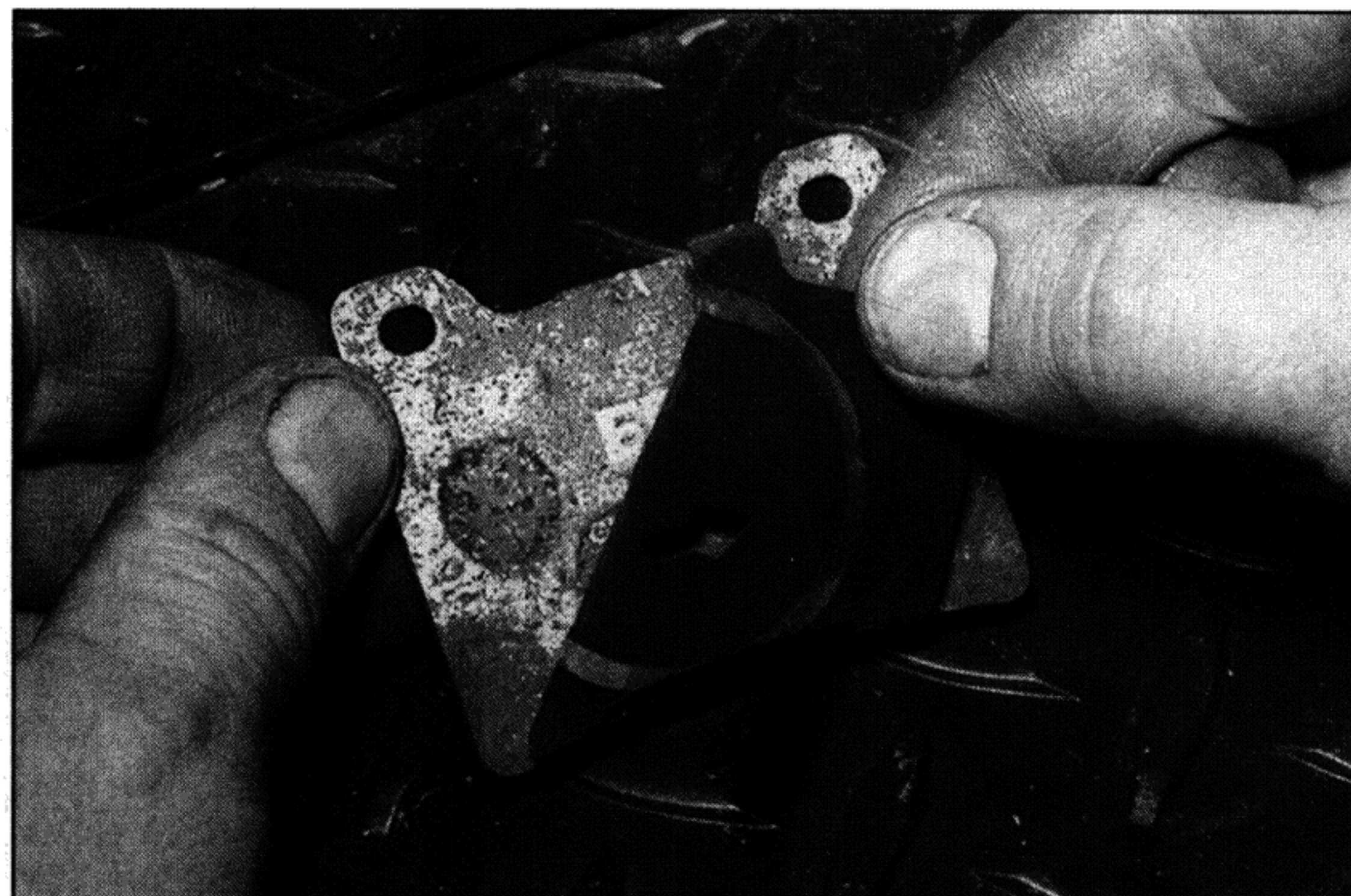
2.9a Fit the shim onto the back of the pad, making sure the arrow points in the direction of normal disc rotation
