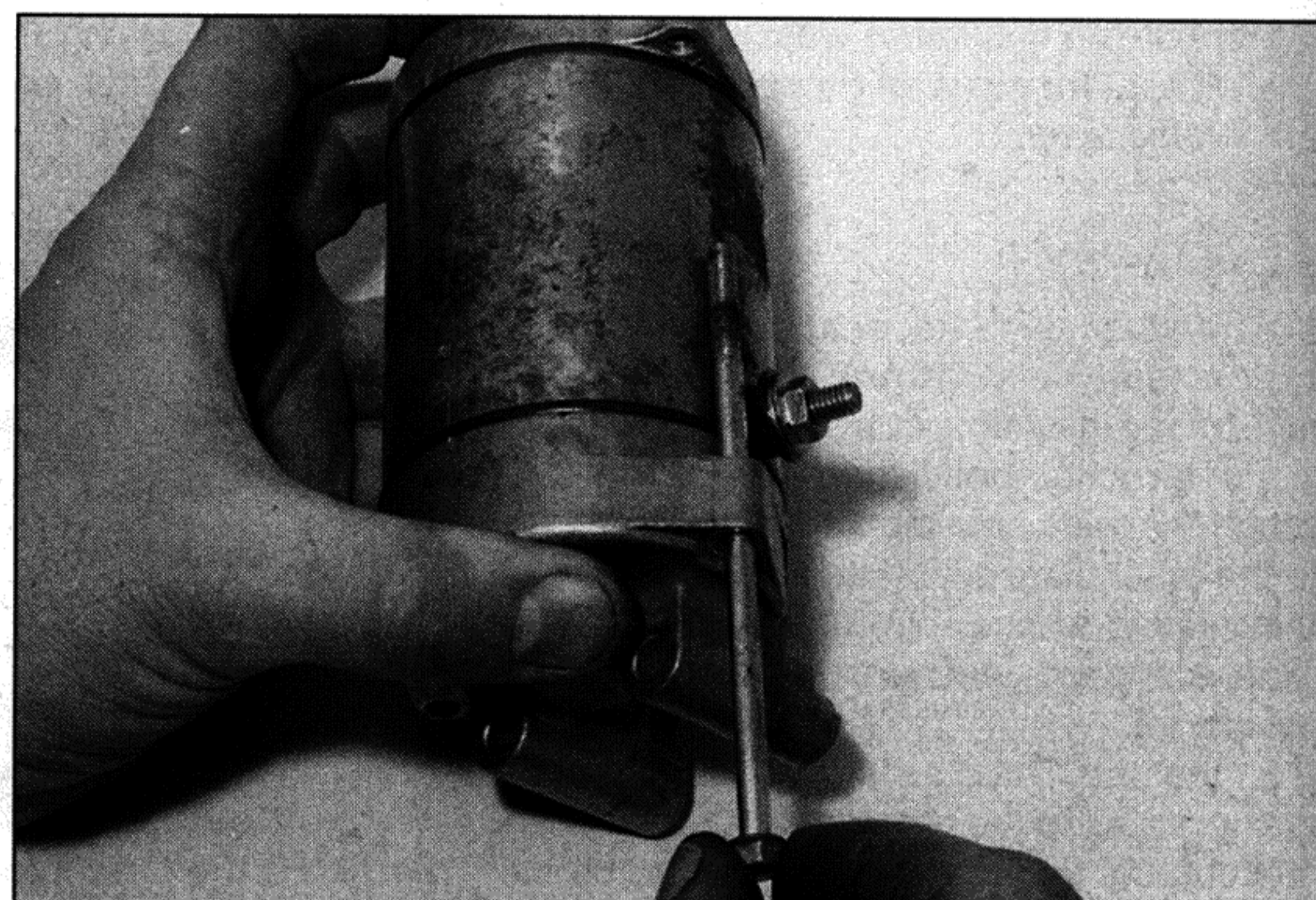
29.21 Install and tighten the long bolts
