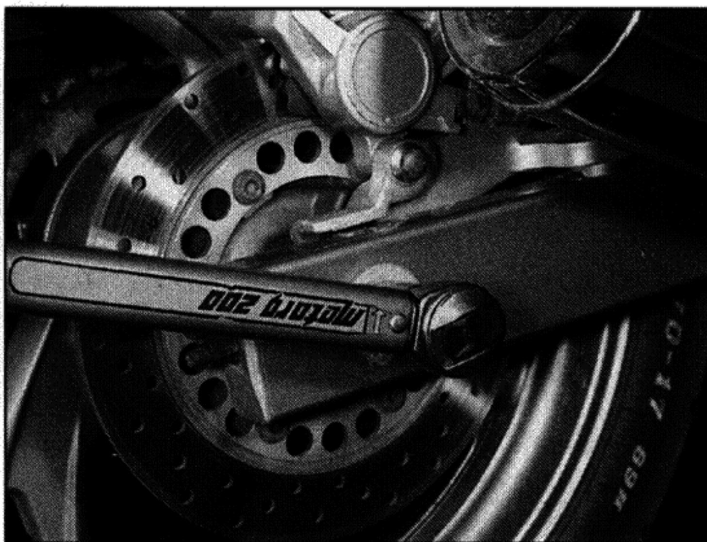
1.13a Tighten the axle nut to the specified torque
