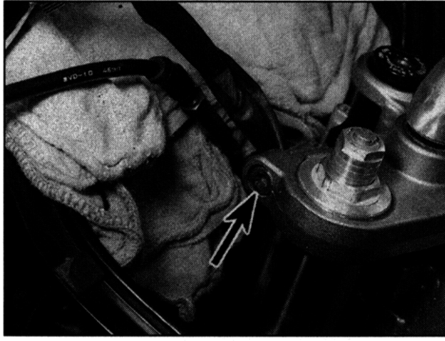
21.6a Slacken the fork clamp bolts (arrowed) . . .
