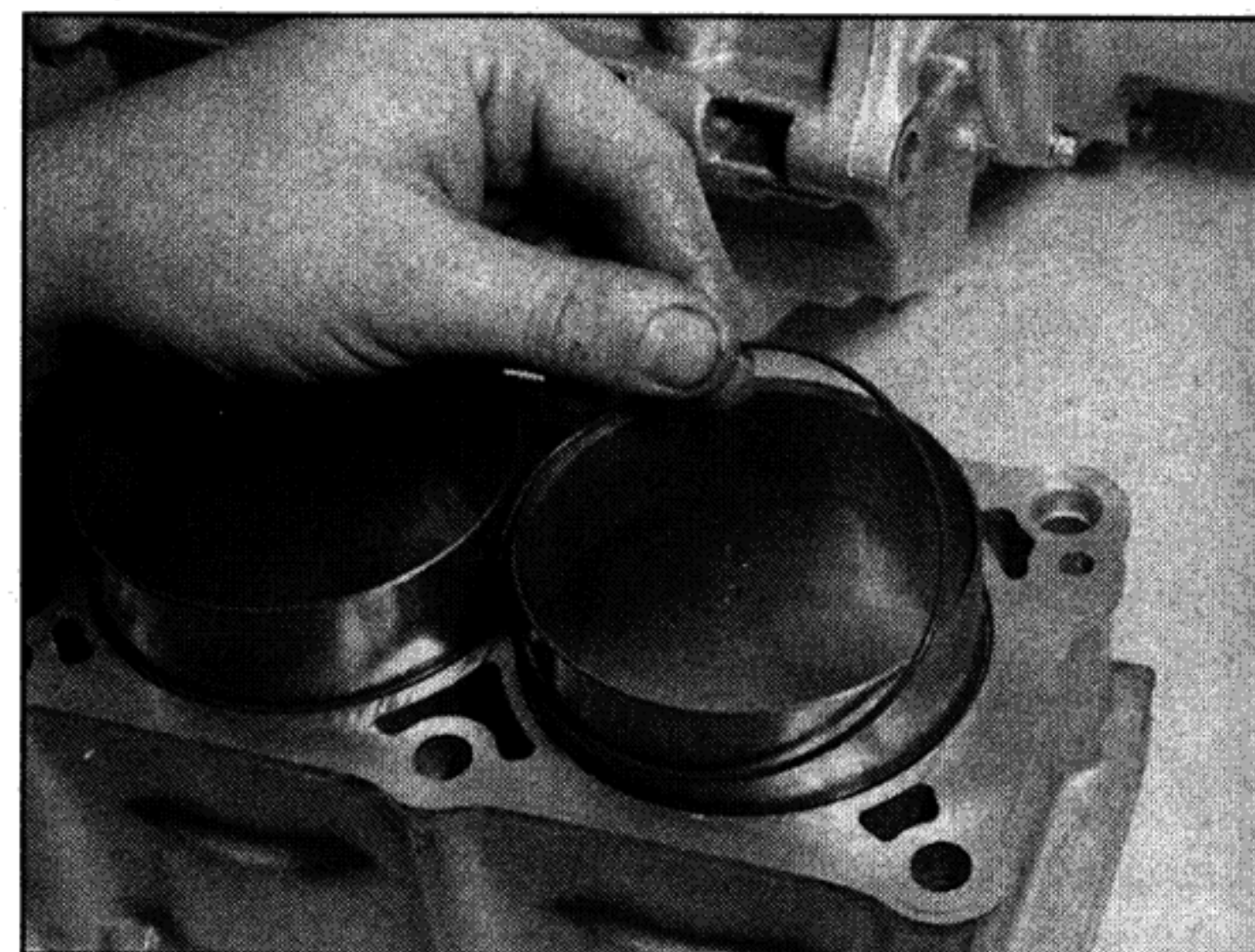
13.14 Fit a new O-ring into the groove around the liner base
