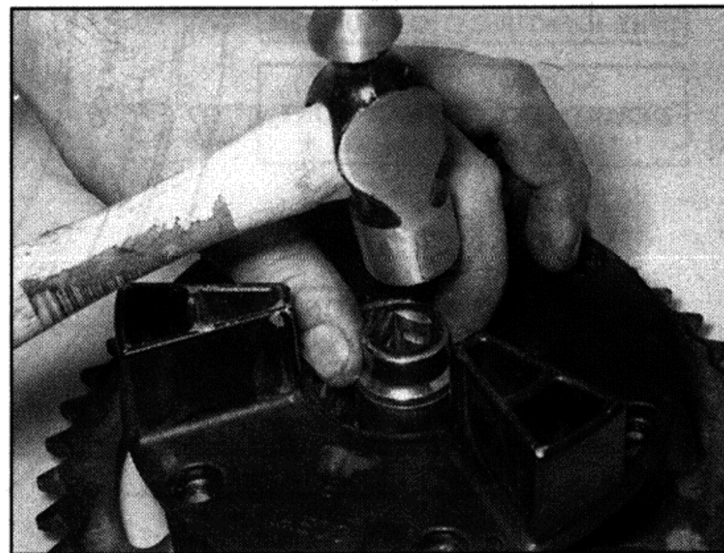
13.27 Drive the bearing out from the inside
