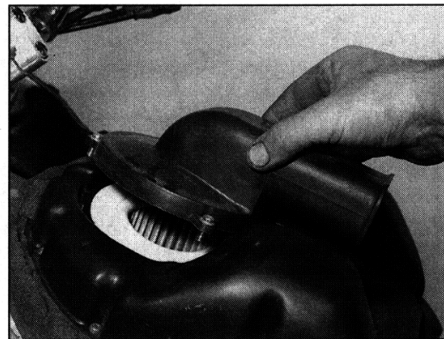
5.6 Make sure the element is correctly seated
