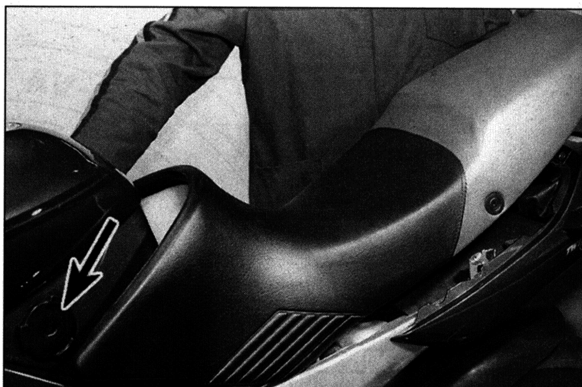
2.3 Make sure the seat locates correctly against the tank – peg-type (arrowed)
