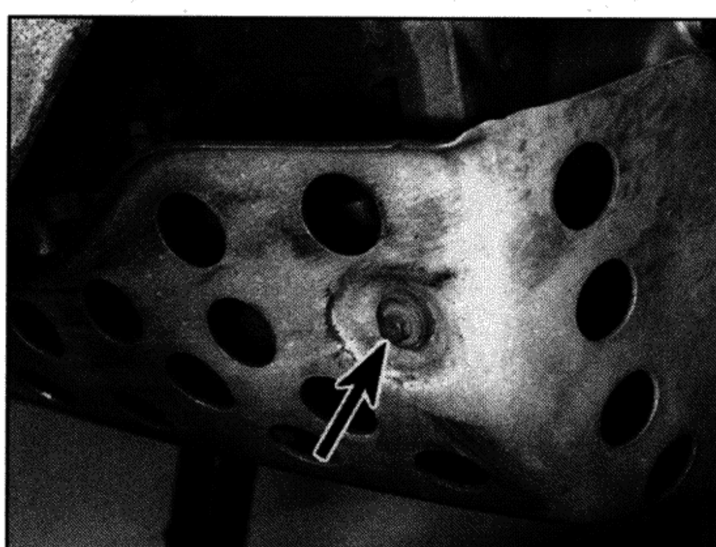
7.2a The bashplate is secured by a bolt (arrowed) on each side at the front . . .
