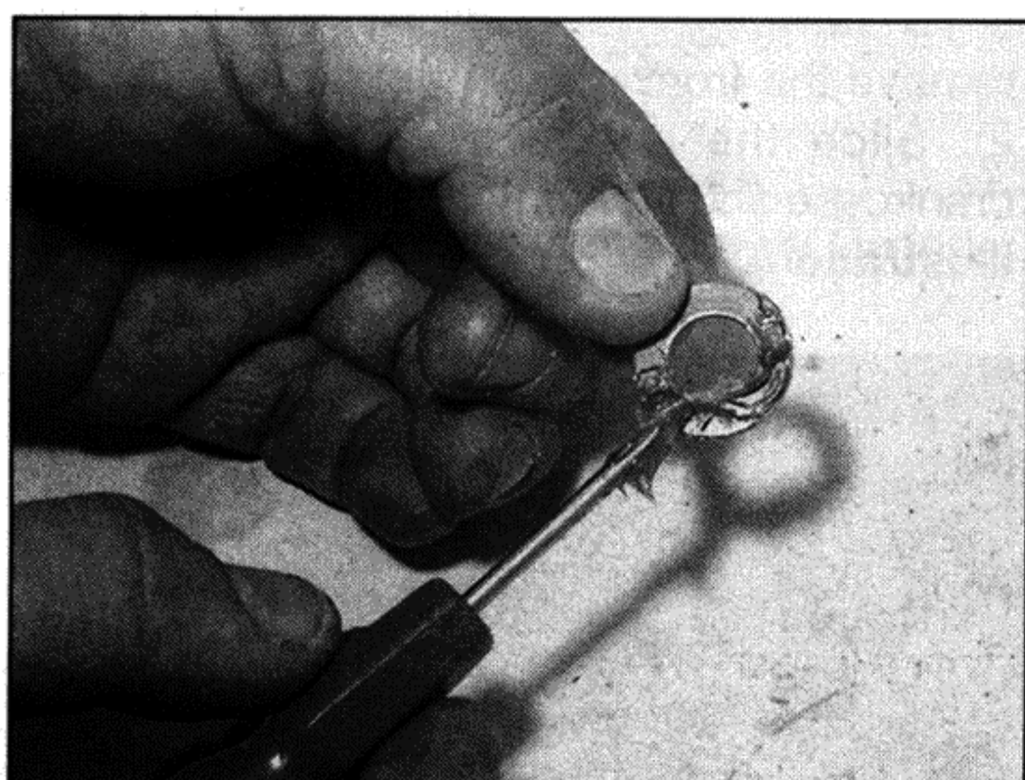
8.12b ... then grease the shim ...
