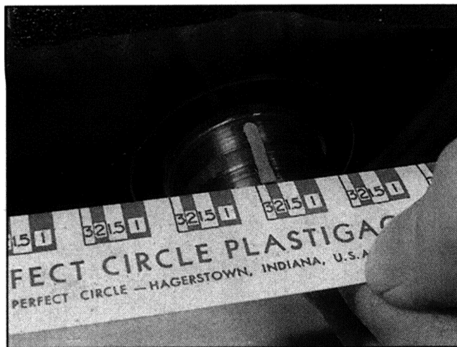
29.20 Measure the width of the crushed Plastigauge (be sure to use the correct scale – metric and imperial are included)
