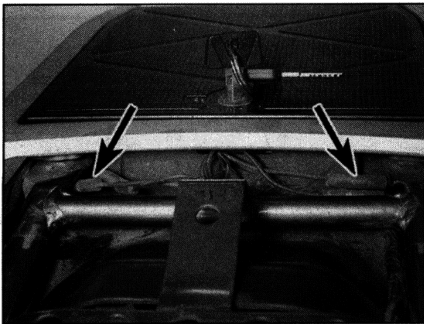
13.1f Rear turn signal wiring connectors – XTZ models
