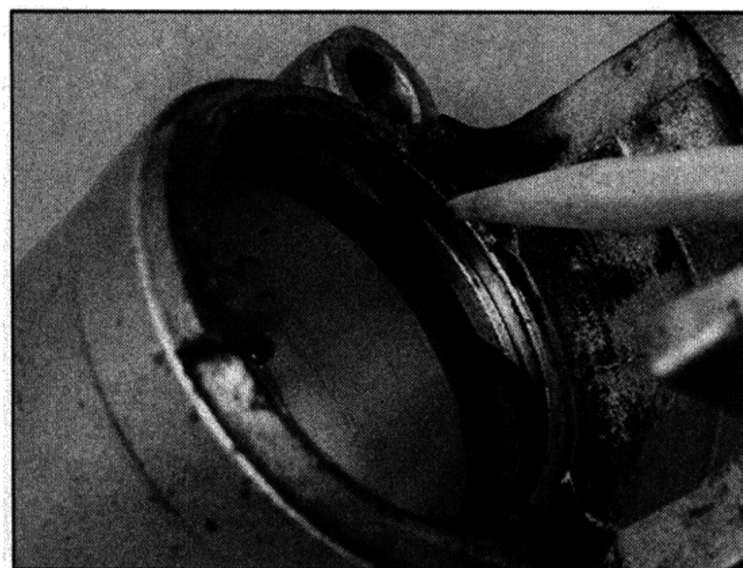
3.7 Use a plastic or wooden tool (such as a pencil) to remove the seals
