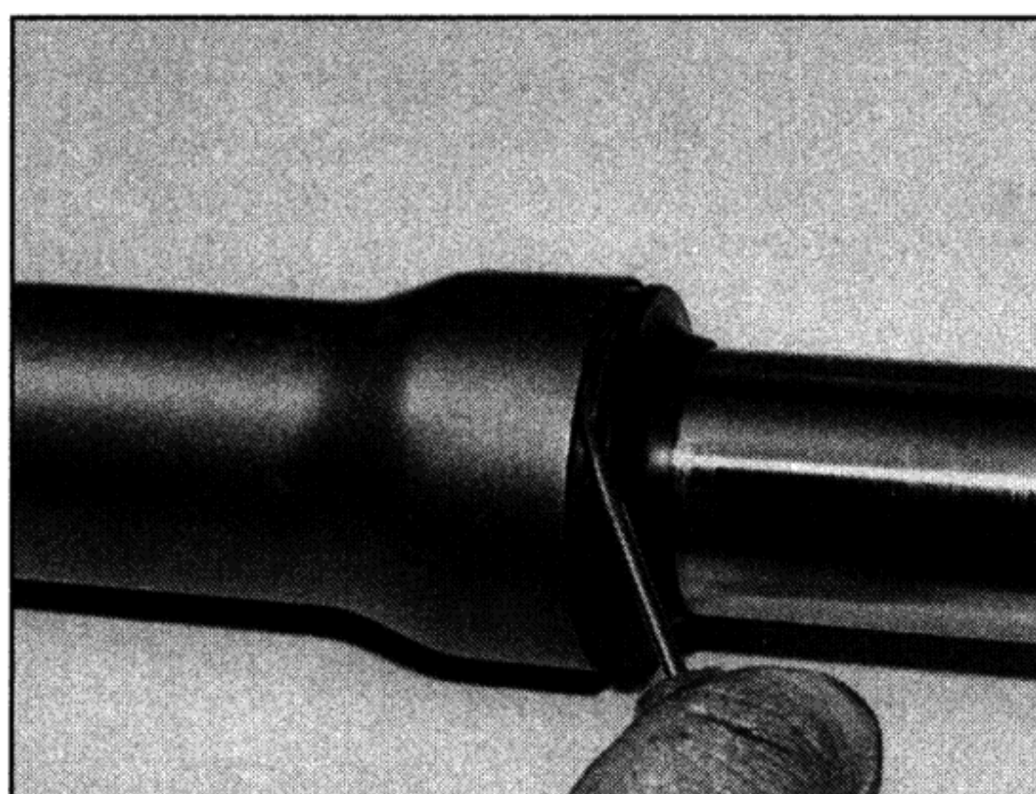
7.10 Prise out the dust seal using a flat-bladed screwdriver
