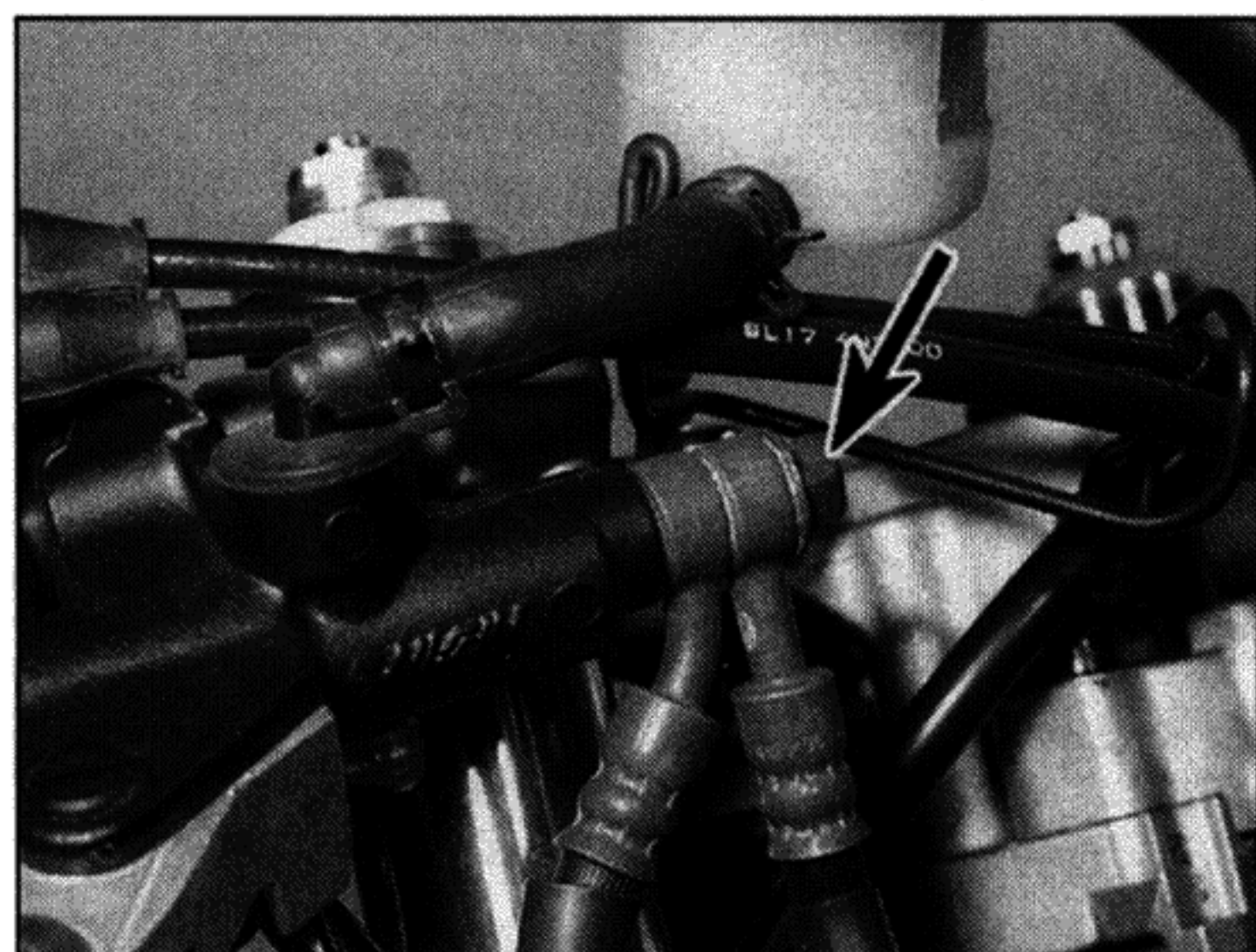
5.6b Brake hose banjo bolt (arrowed) – TRX models
