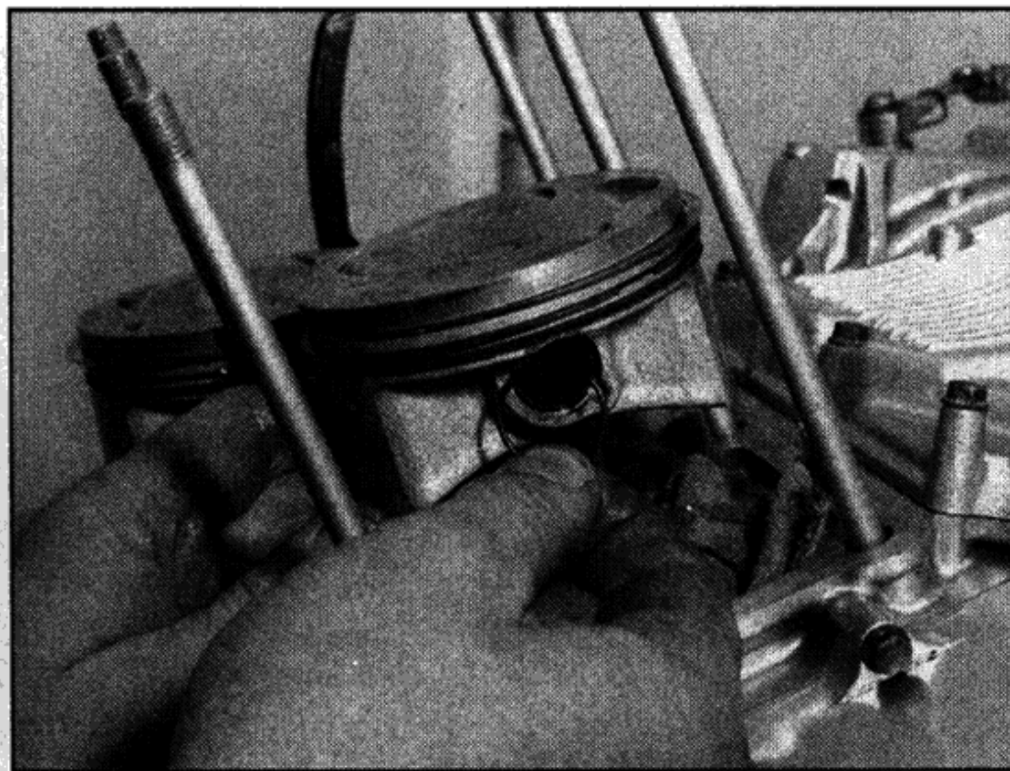
14.16b Do not over-compress the circlip when fitting it into the piston
