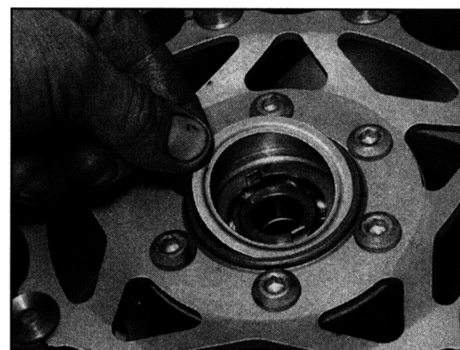
13.12b . . . then fit the retainer plate
