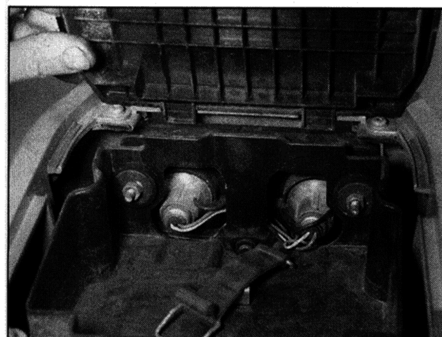
9.1 On XTZ models, remove the storage cover to access the bulbs
