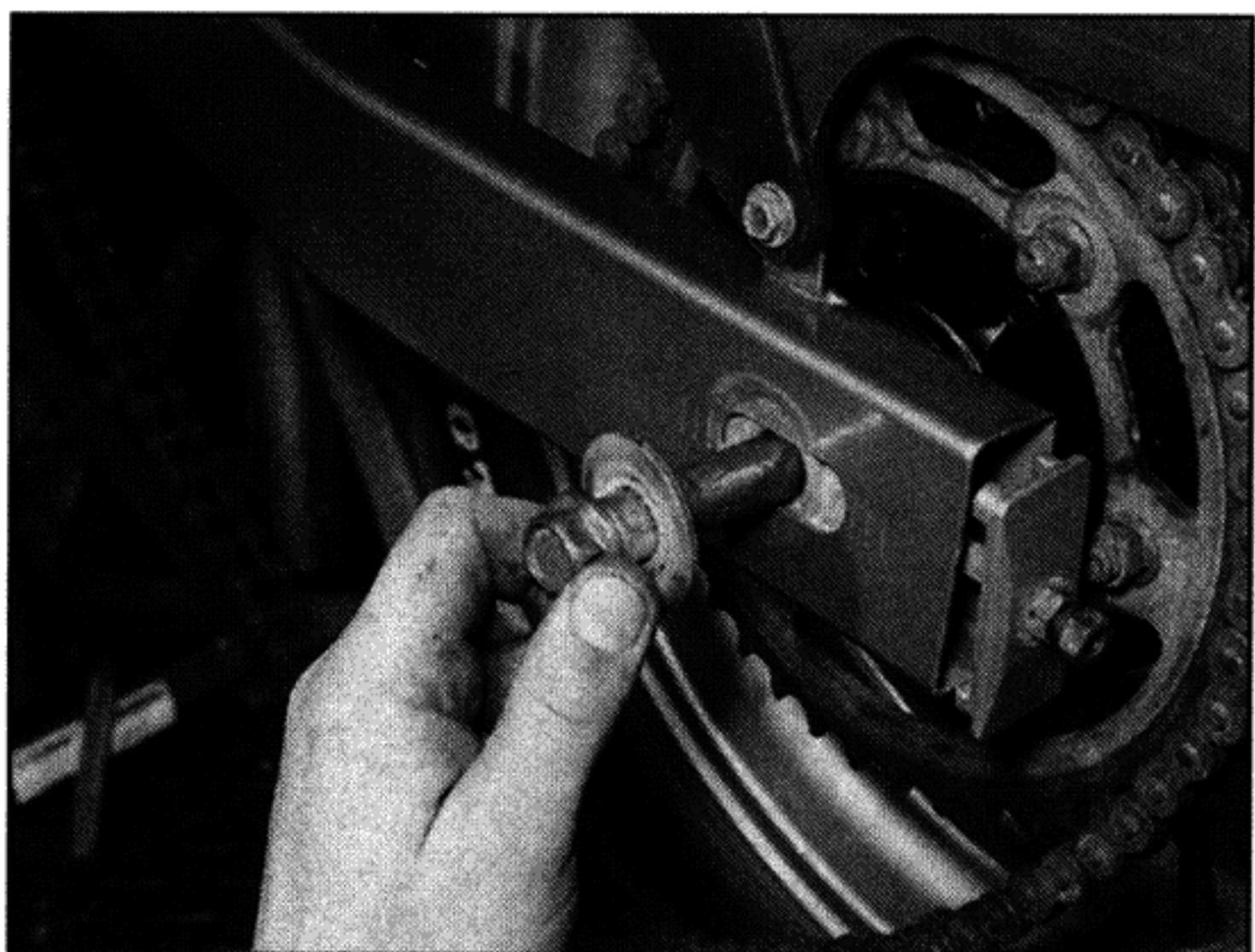
12.4 Withdraw the axle and remove the wheel
