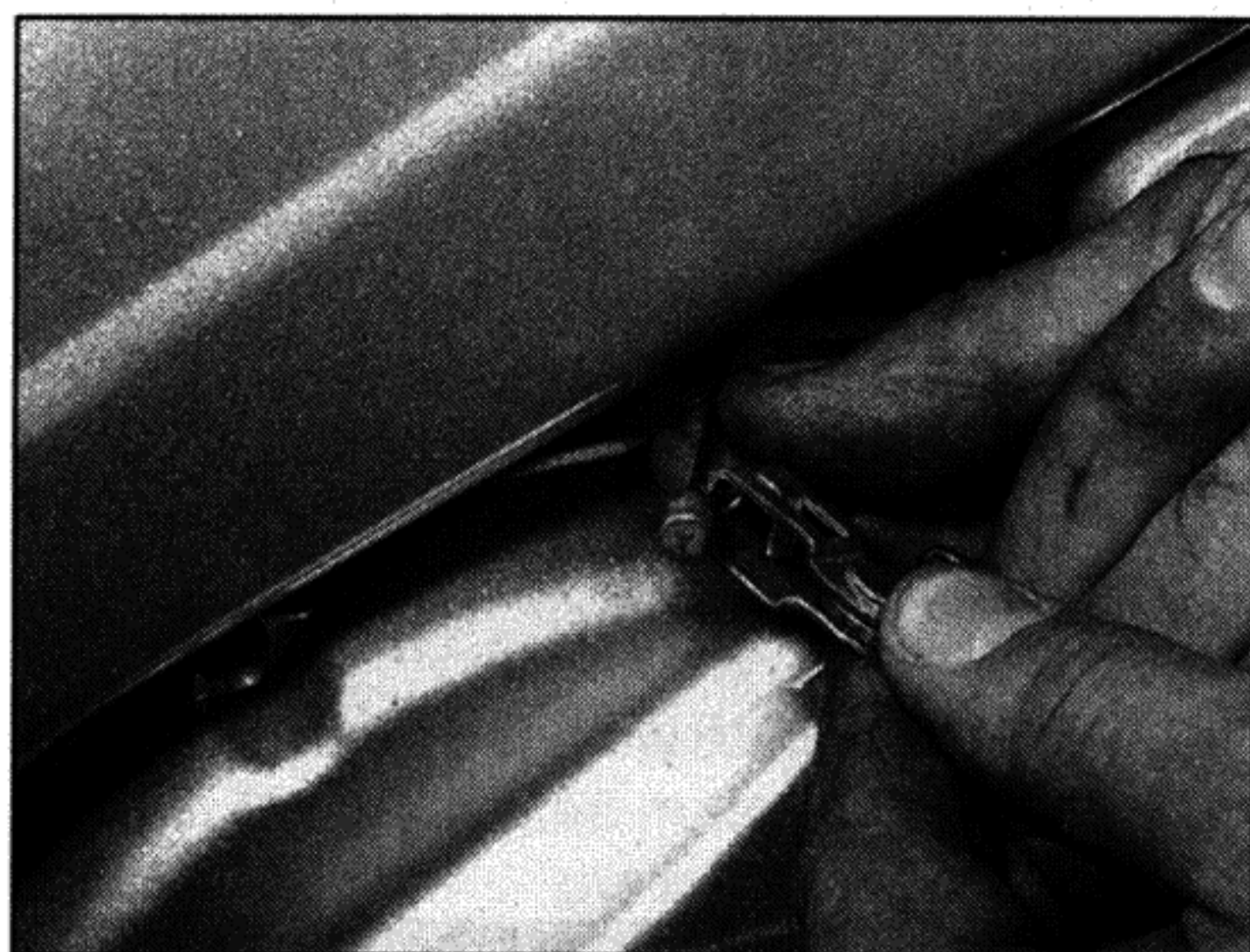
17.1d . . . and detach the cable
