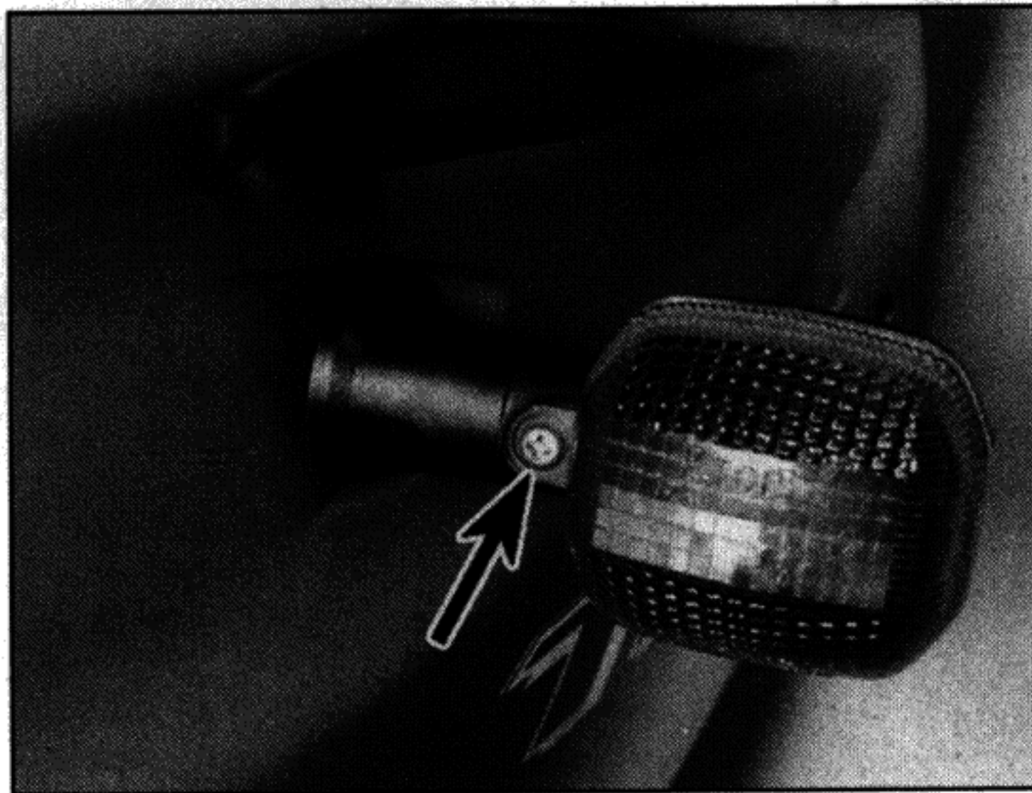
12.1b Turn signal lens screw (arrowed) – TRX models
