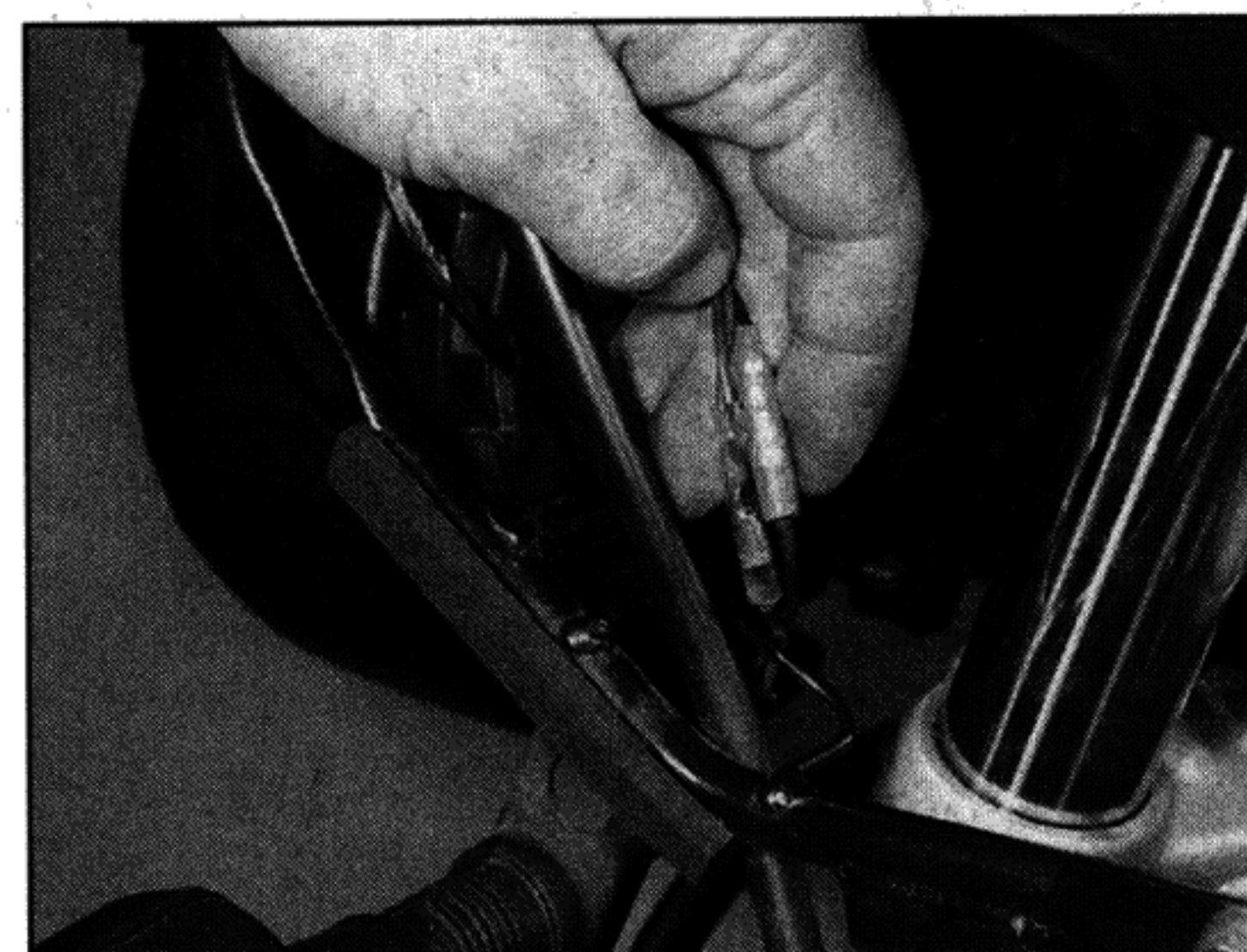
13.1a Front turn signal wiring connectors – TDM models
