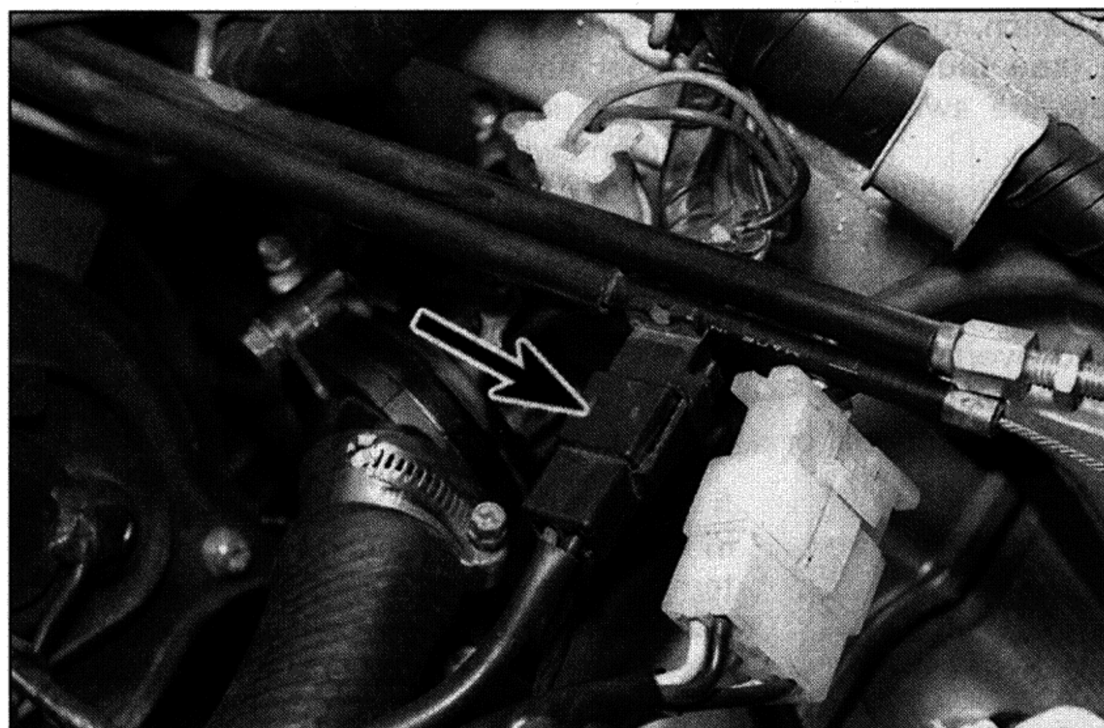
4.3a Fan motor wiring connector (arrowed) – TDM models
