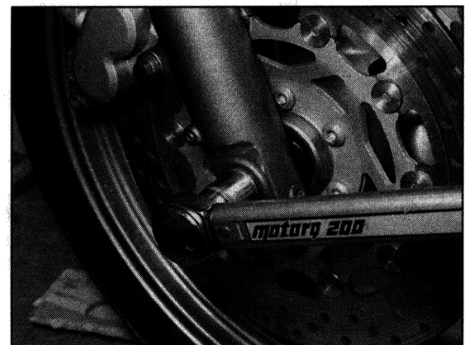
11.13 Tighten the axle to the specified torque
