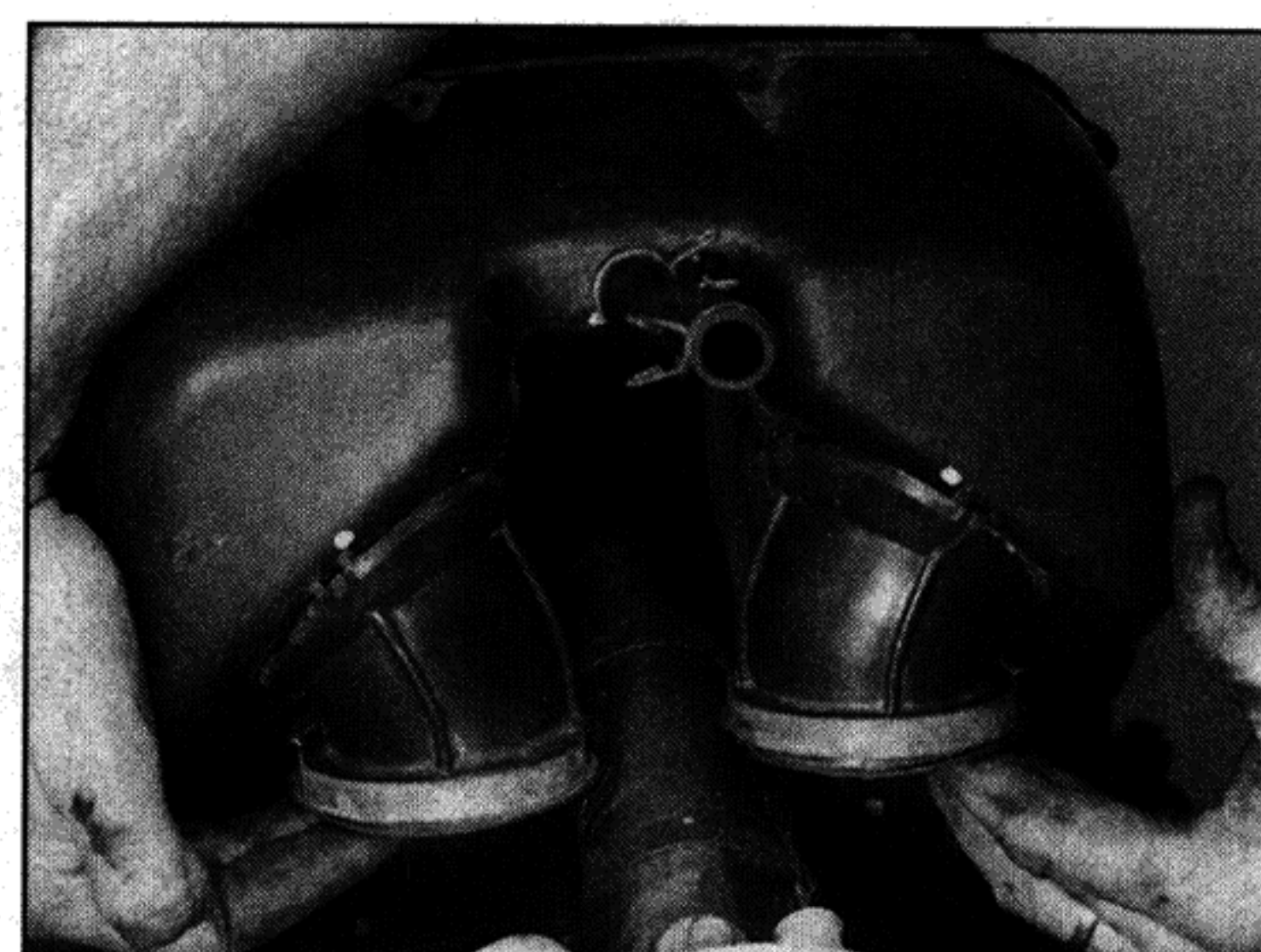
4.4b On XTZ models, draw the ducts apart to clear the frame
