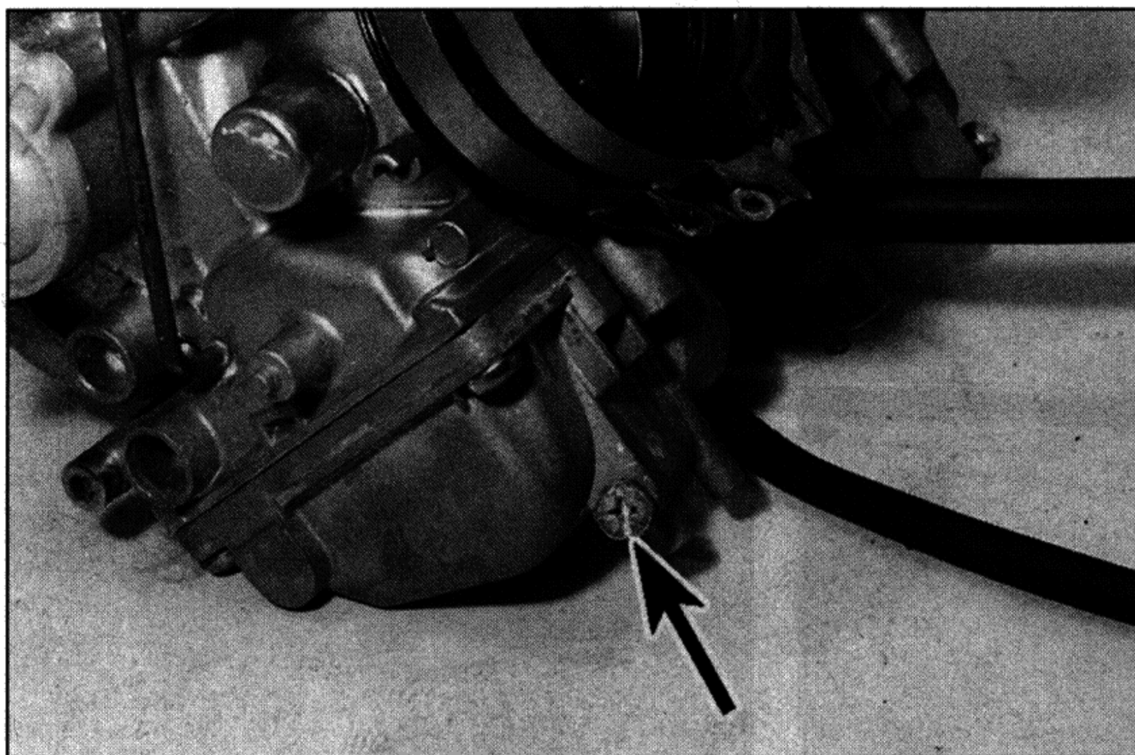
7.8 Float chamber drain screw (arrowed)
