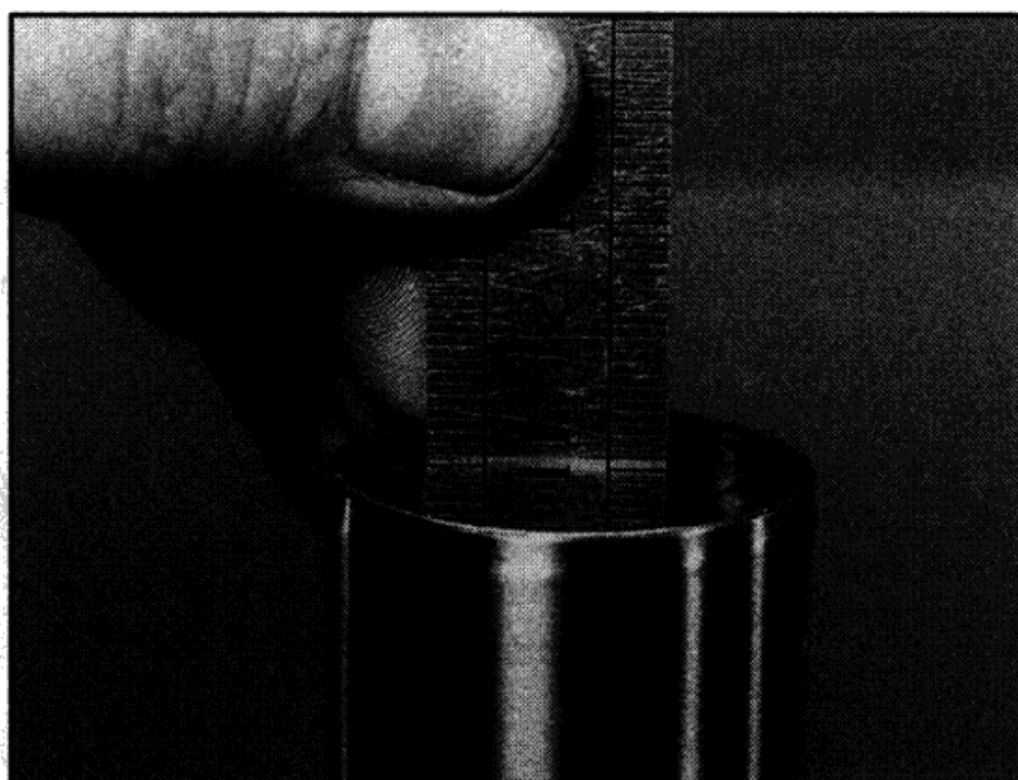
7.26b Measure the oil level with the fork held vertical
