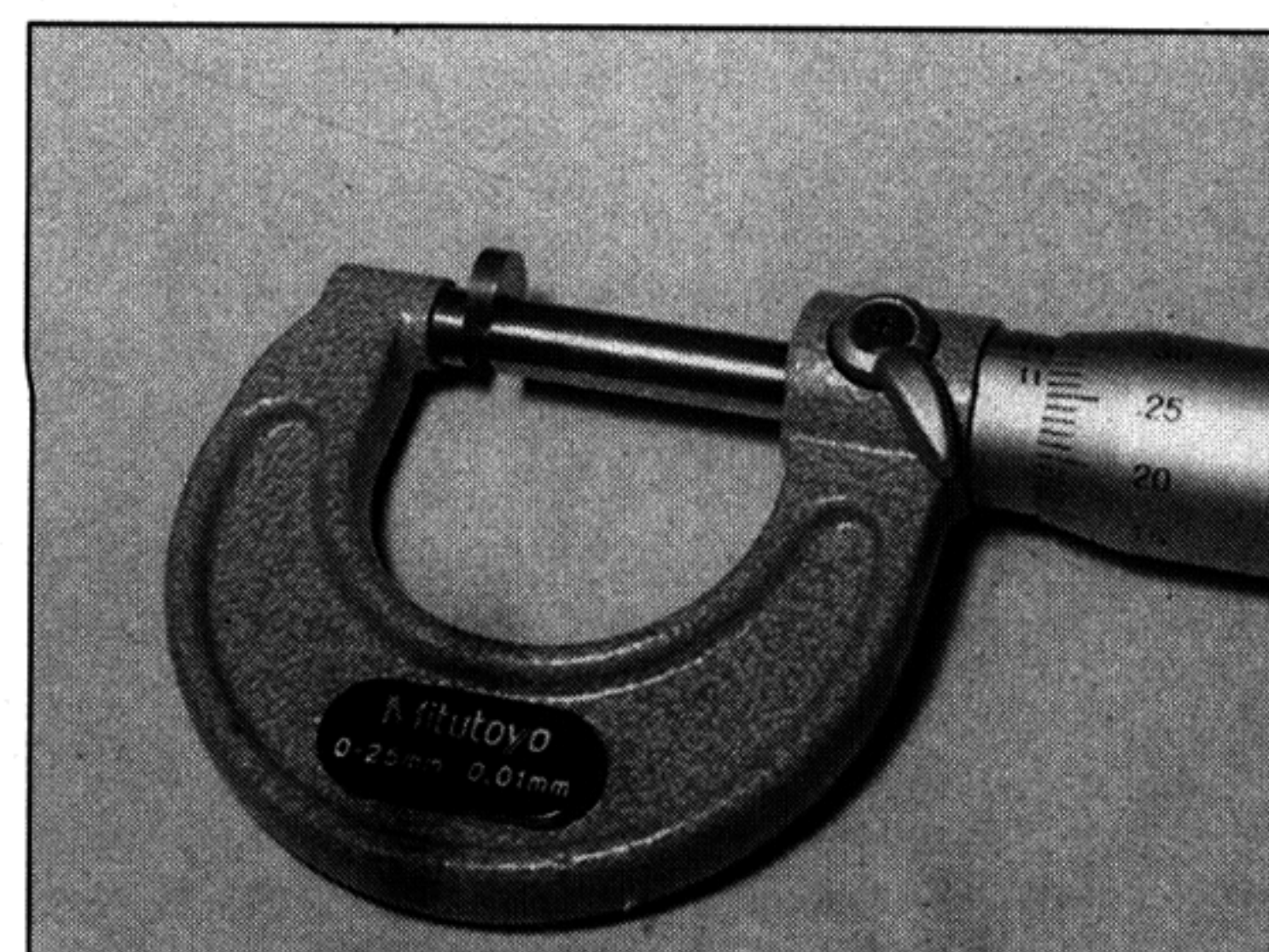
28.11 Measure the shim using a micrometer
