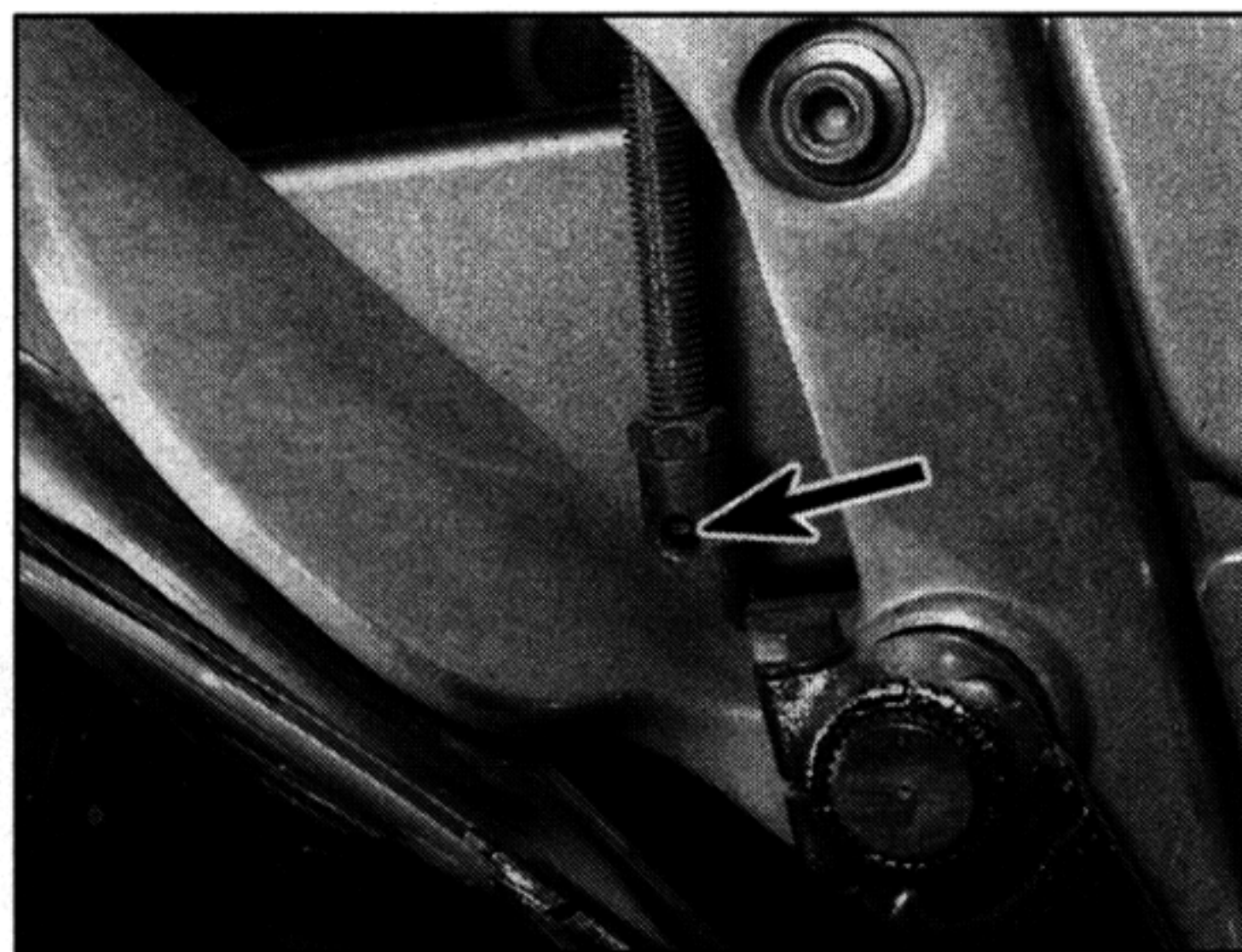
9.8b . . . making sure the rod end is still visible in the hole (arrowed) (TDM and TRX models)
