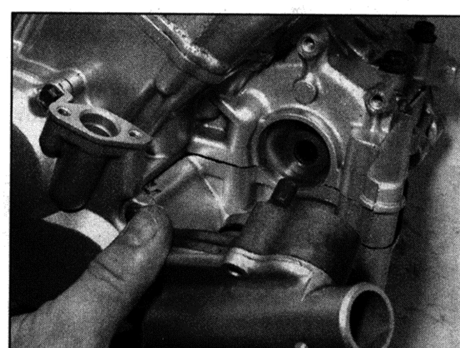
8.12d Install the pump, making sure it locates correctly into the drive gear
