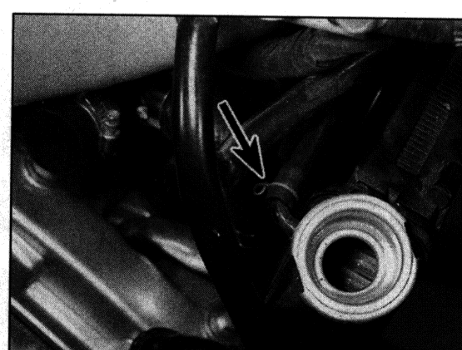
7.3c ... and on TDM and TRX models the overflow hose (arrowed)
