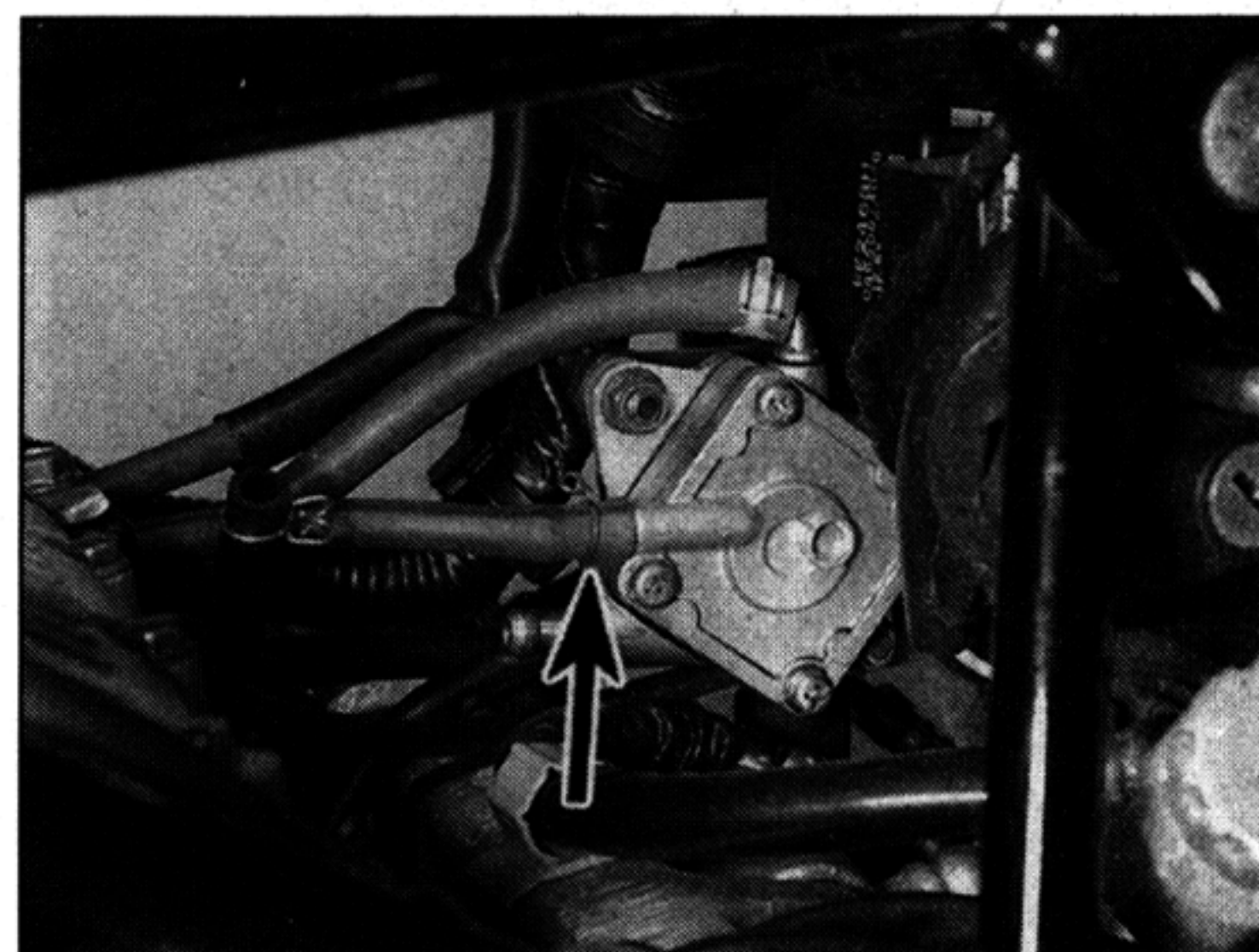
4.6 On TRX models, detach the No. 2 vacuum hose (arrowed) from the fuel pump
