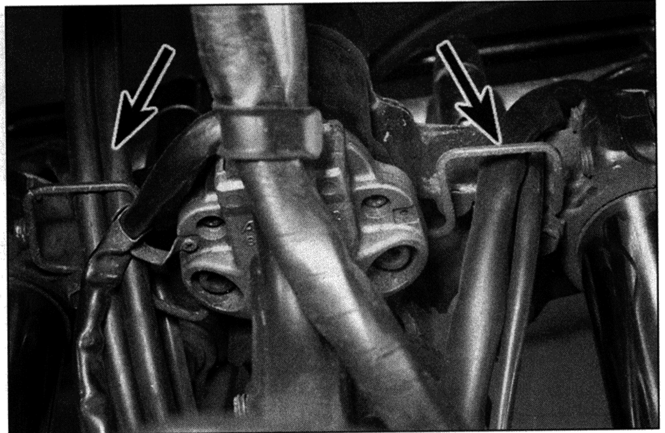
8.4a Free the cable and wiring from the guides (arrowed) on the top yoke . . .
