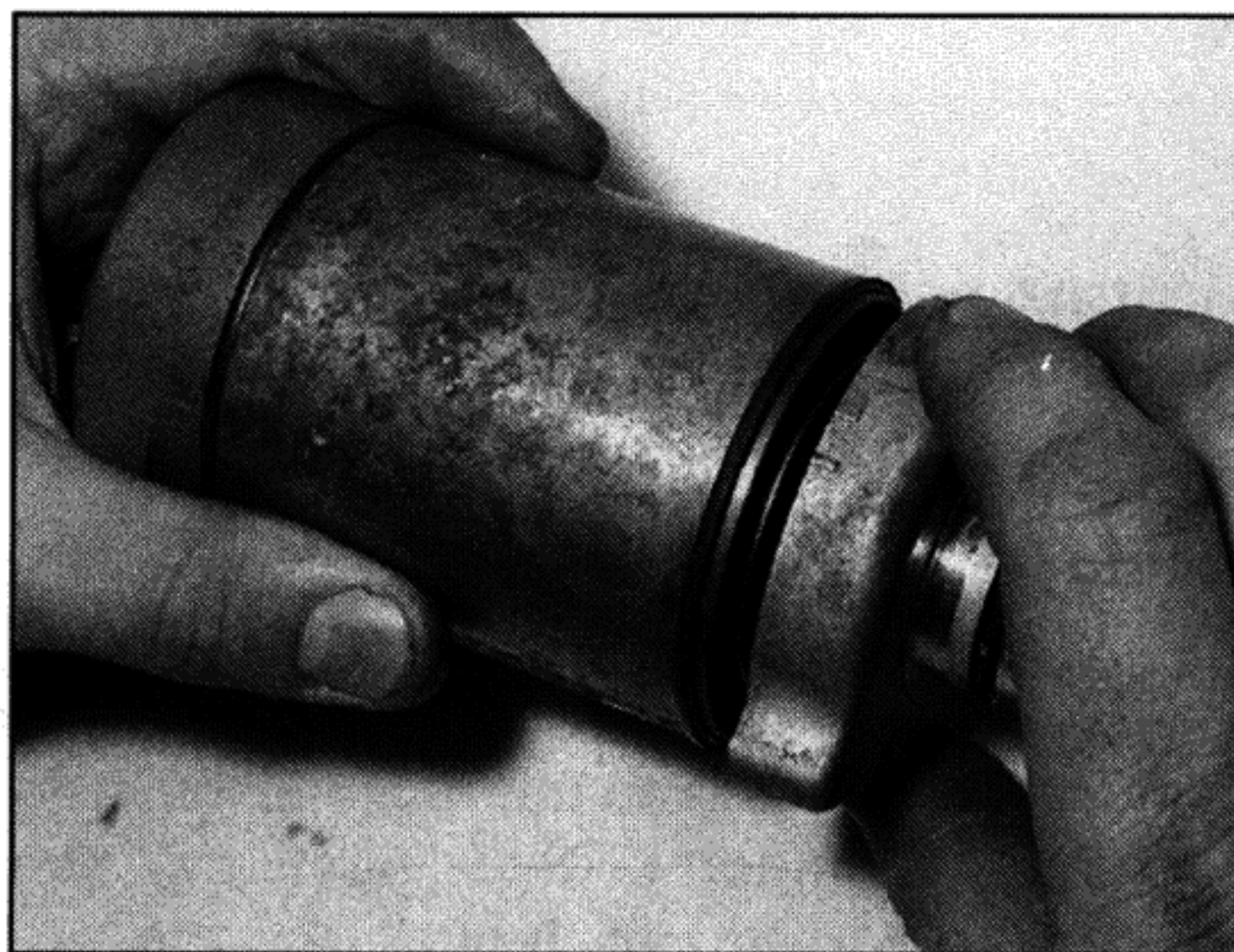
29.4a Remove the front cover . . .
