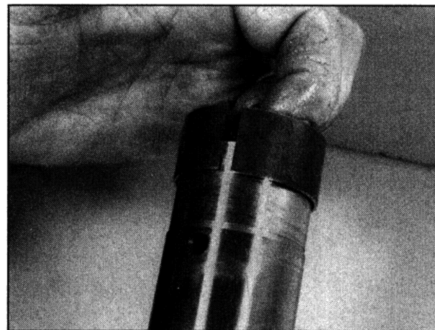
7.18 Prise off the bottom bush using a flat-bladed screwdriver
