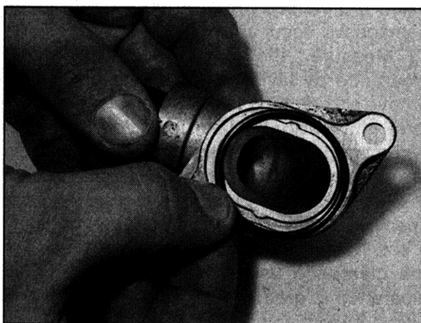
13.20a Fit a new O-ring onto the union . . .
