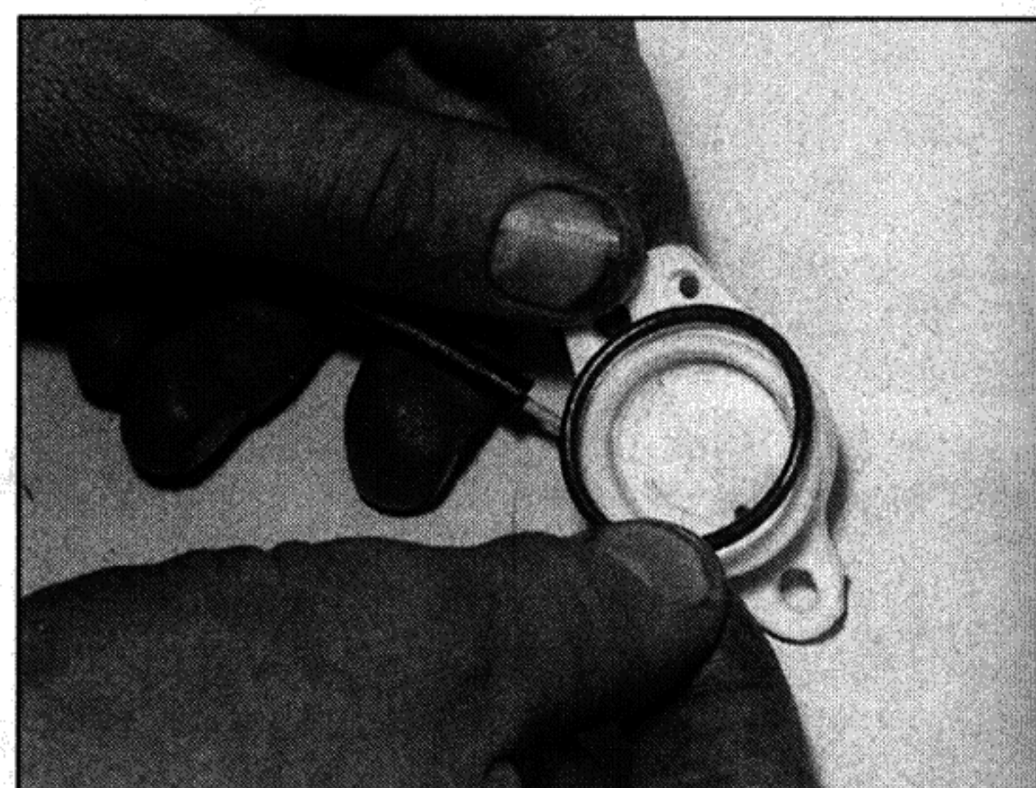
21.11 Fit a new O-ring onto the switch
