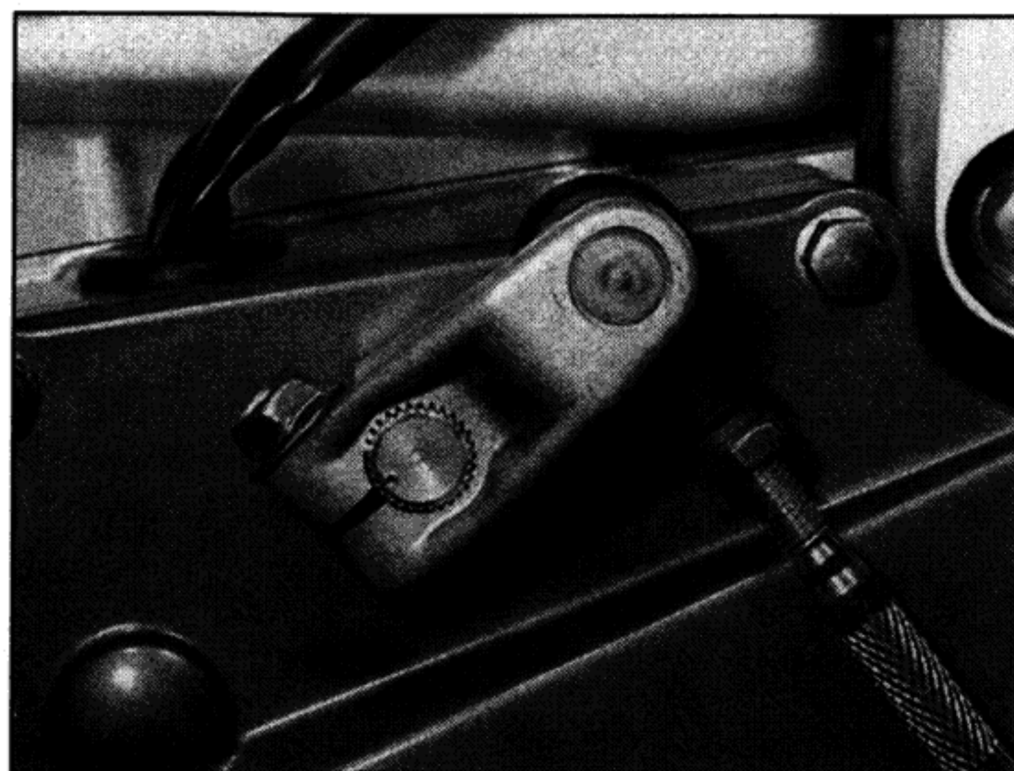
15.3 Linkage arm/shaft alignment – TRX models
