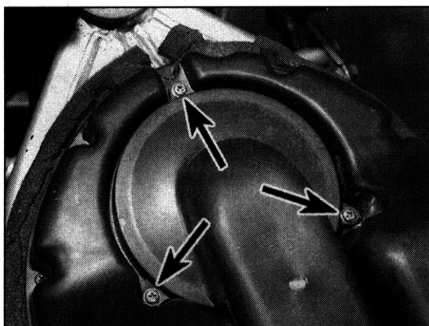
5.2a Remove the screws (arrowed) and lift off the cover . . .
