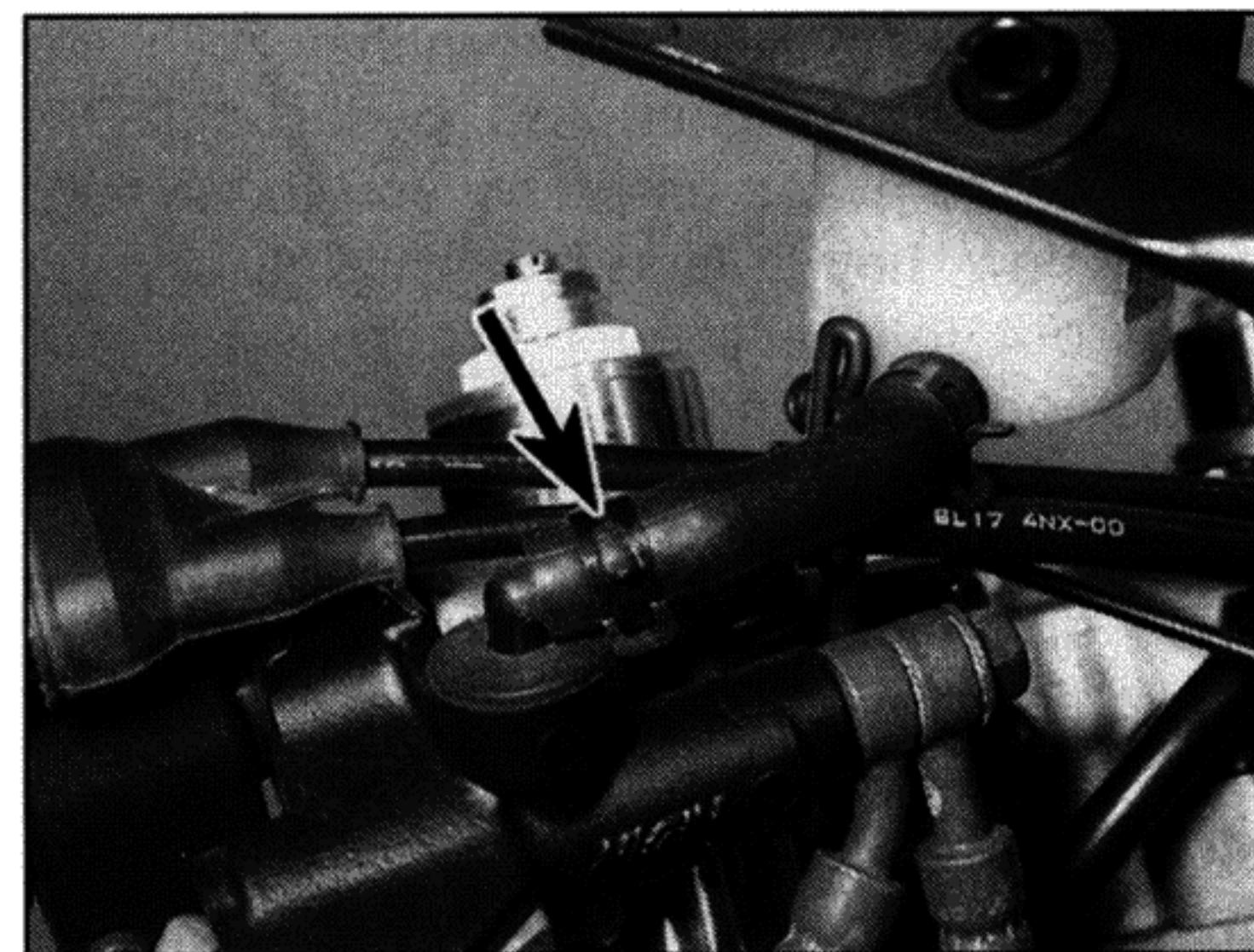
5.7b . . . and hose clamp – TRX models
