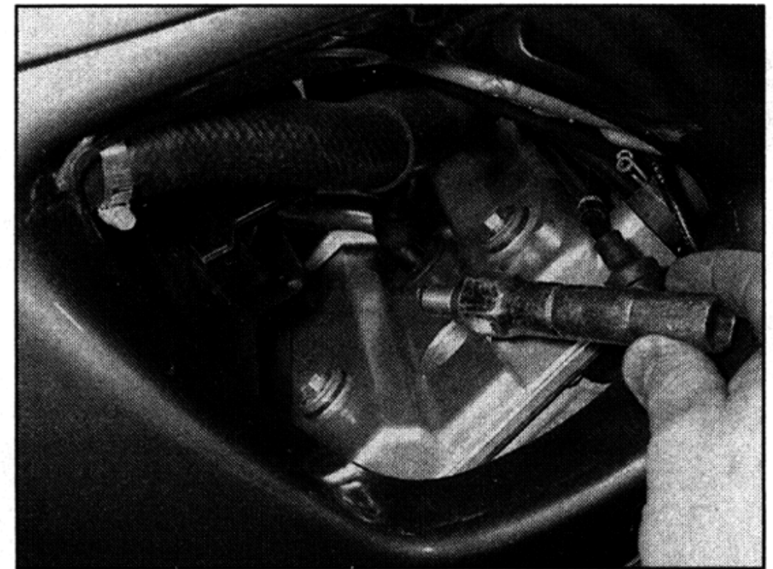
2.9 Thread the plug in as far as possible by turning the tool by hand
