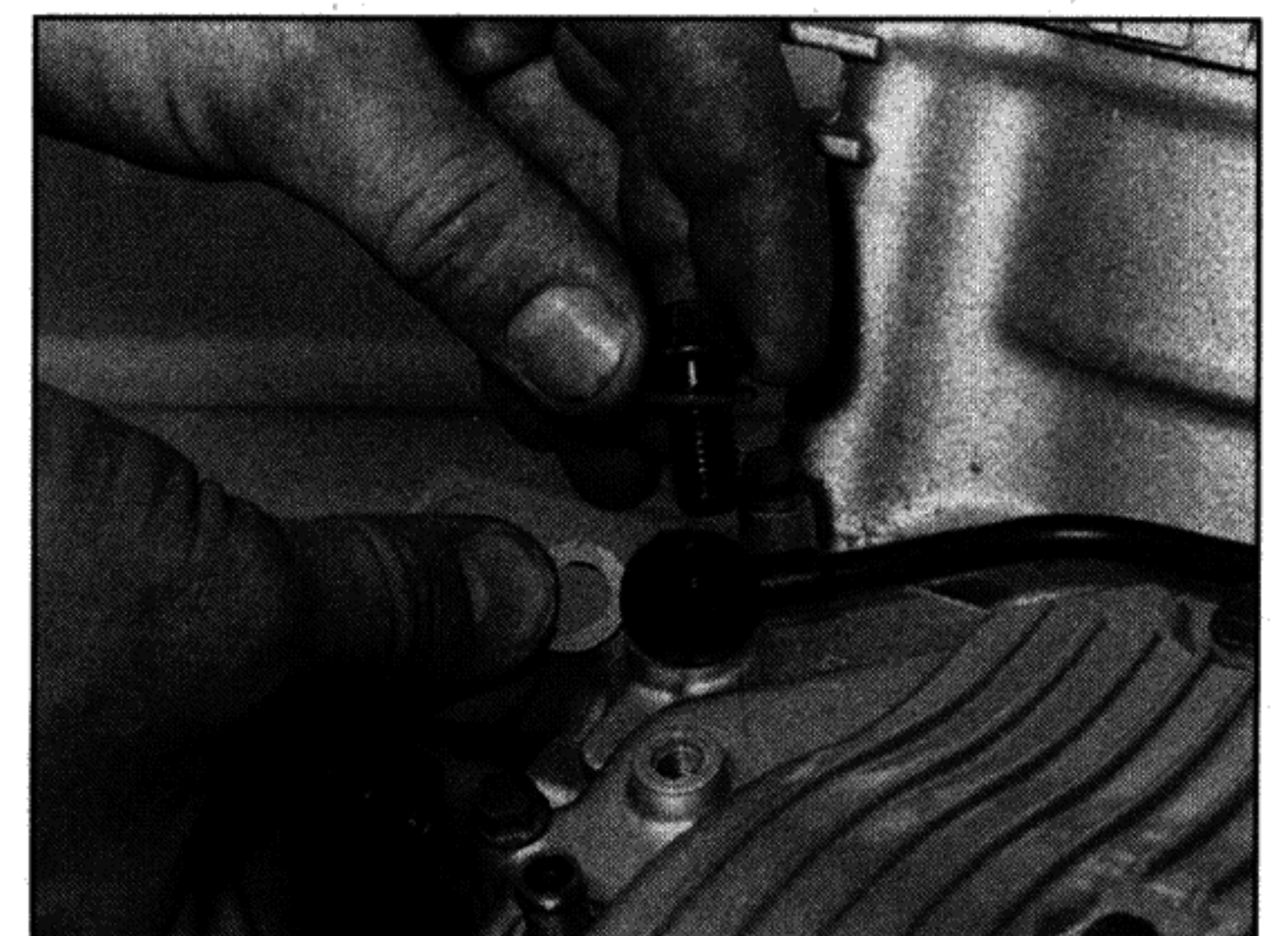
23.16c Use new sealing washers on each side of the union
