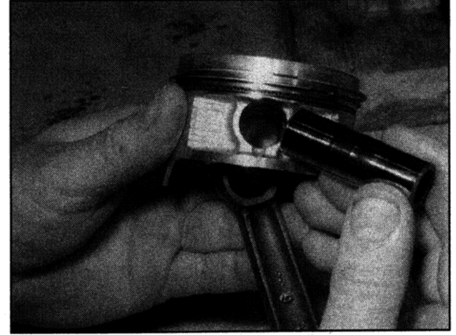
14.16a Align the piston with the connecting rod small-end and insert the pin
