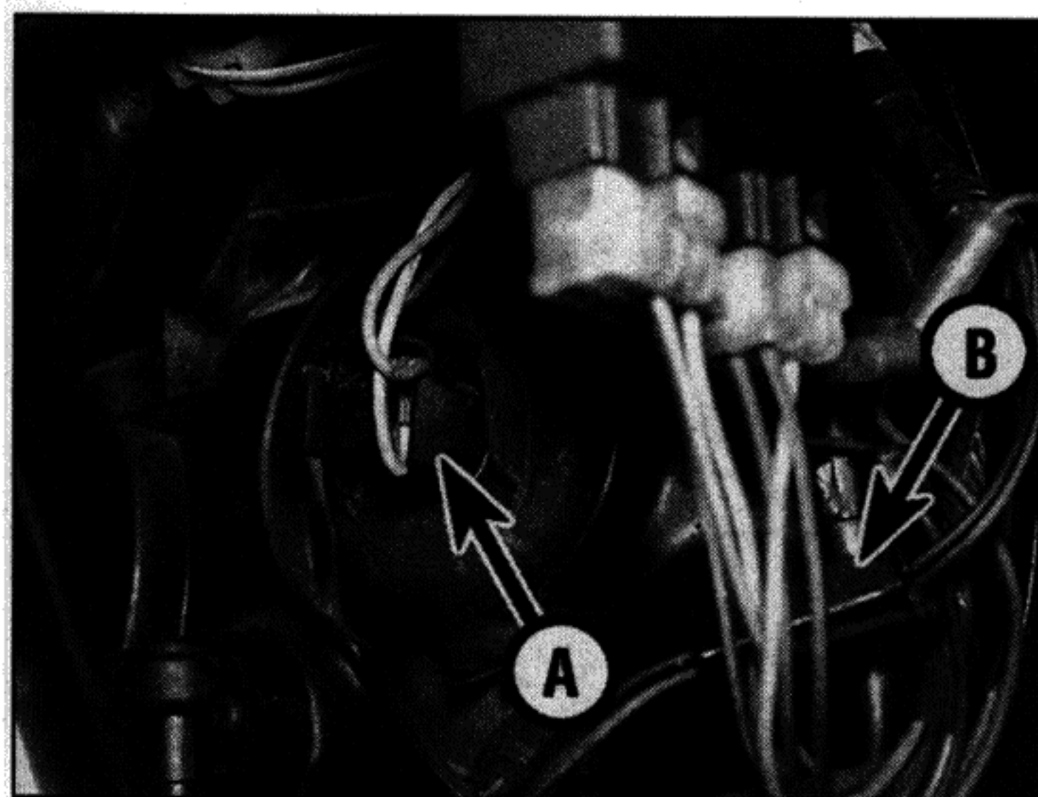
5.15 Disconnect the headlight wiring connector (A) and the auxiliary light wiring connector (B) for each light
