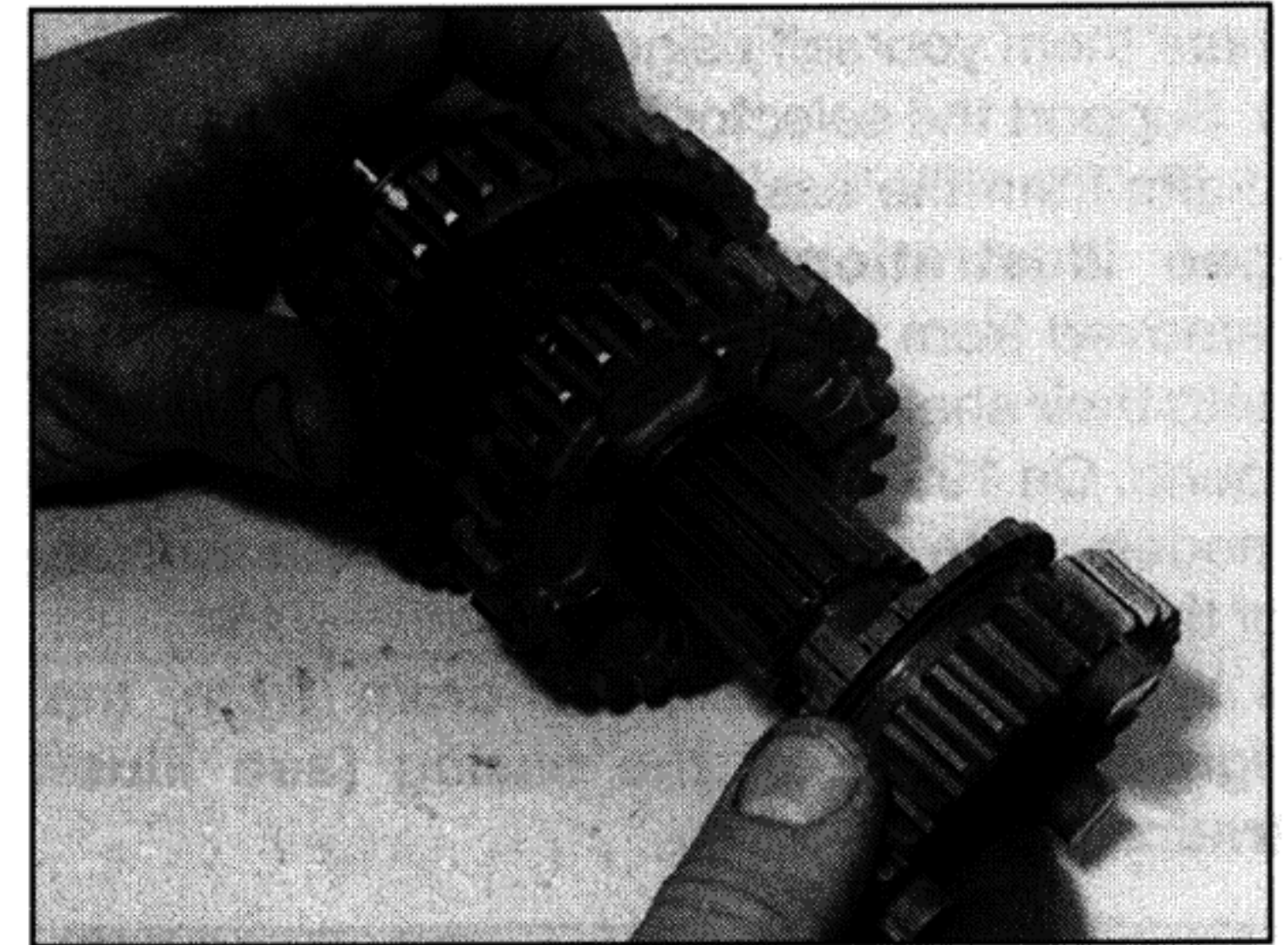
31.40a Slide on the 4th gear pinion, making sure it is the correct way round ...
