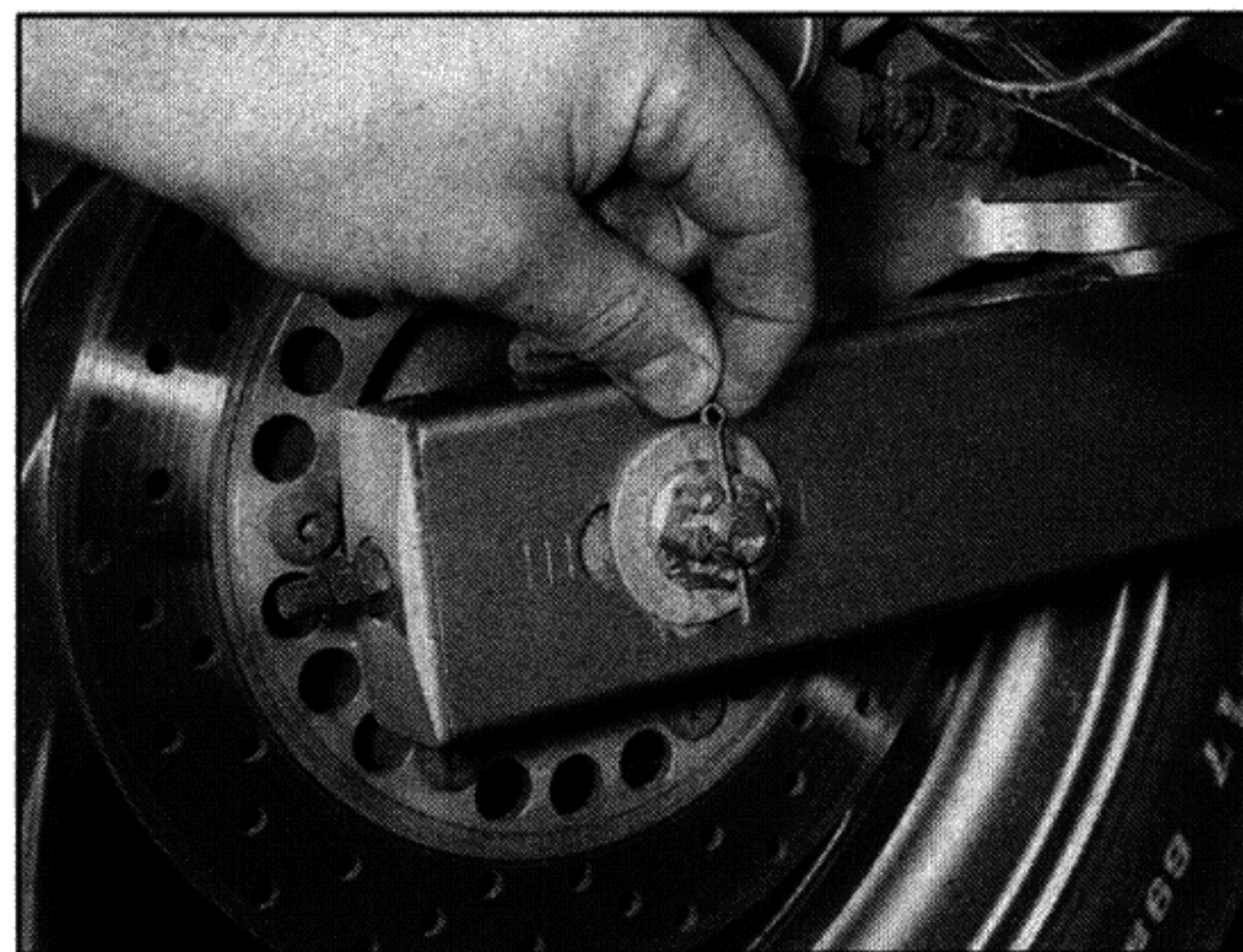
1.13b Use a new split pin, where appropriate
