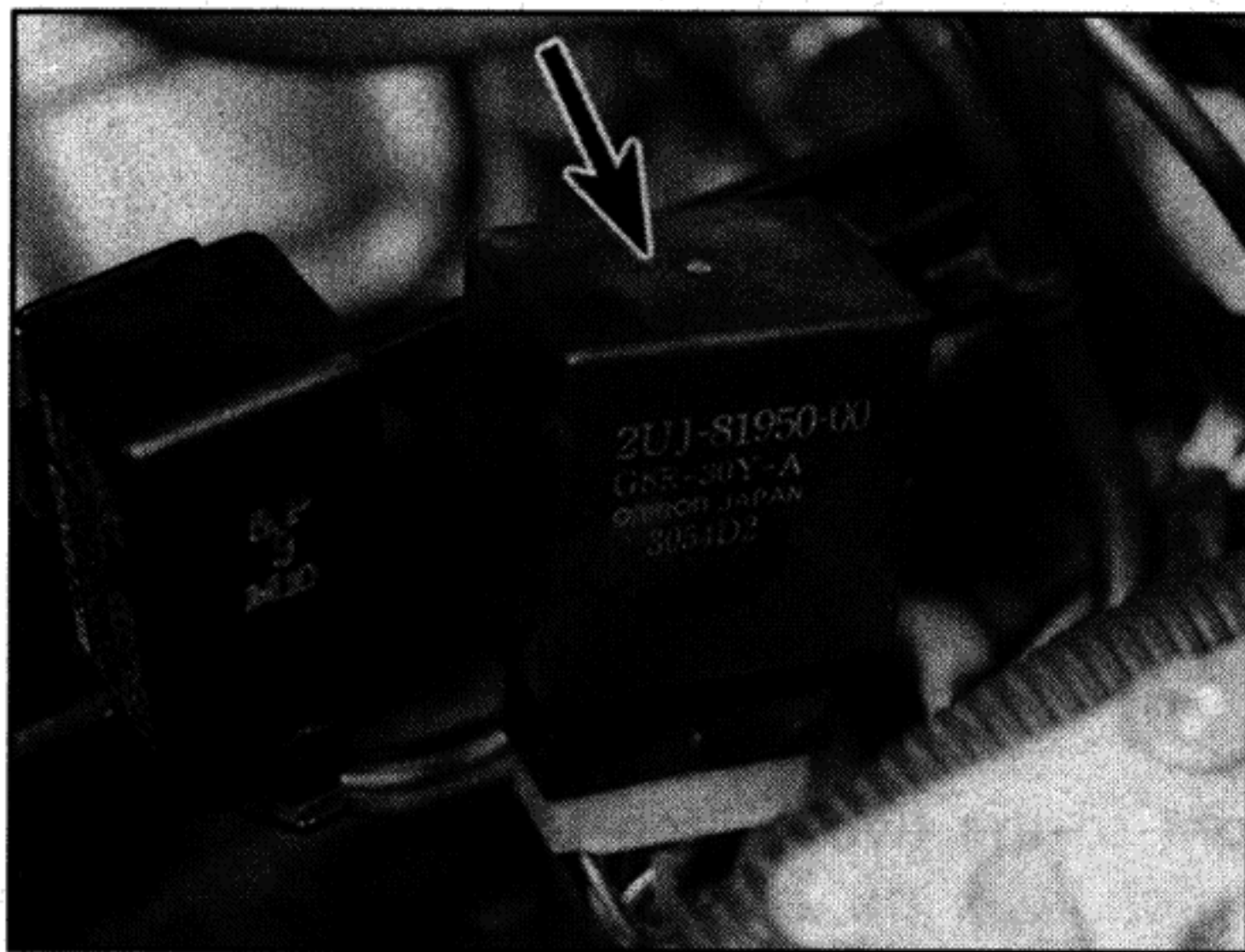
25.2a Starter circuit cut-off relay (arrowed) – TDM models
