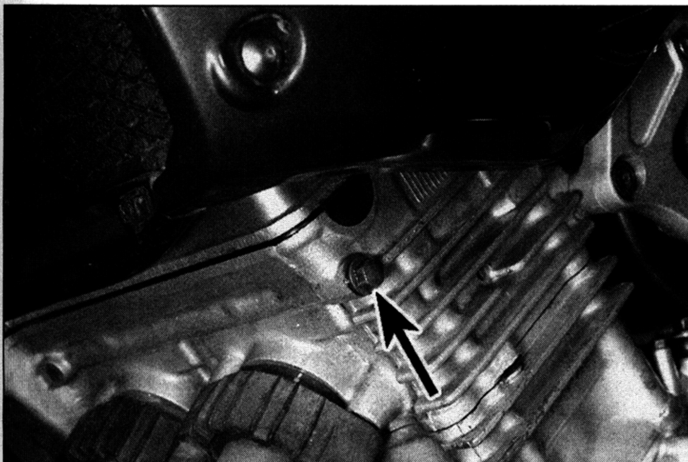
32.3 Slacken the gallery bolt (arrowed) . . .
