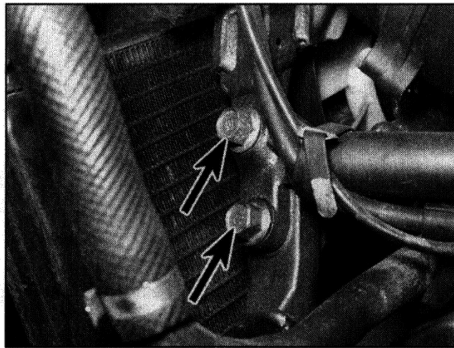
5.23b Downtube upper bolts (arrowed)
