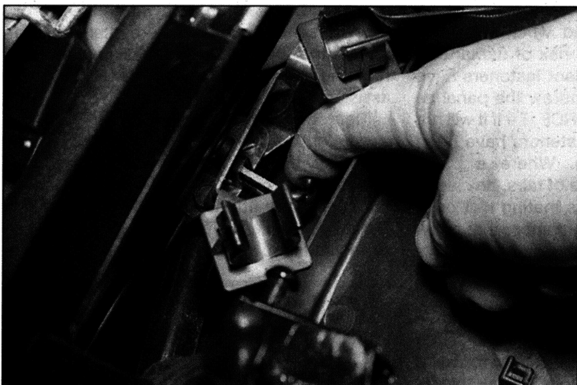
2.7 Pull back the latch to release the rider's seat
