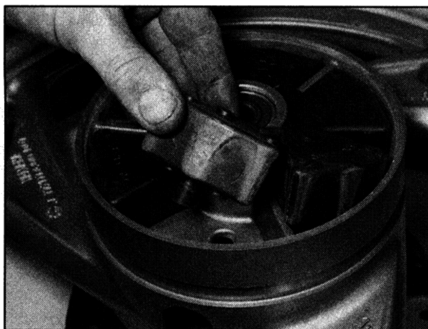
17.3 . . . and remove the rubber dampers
