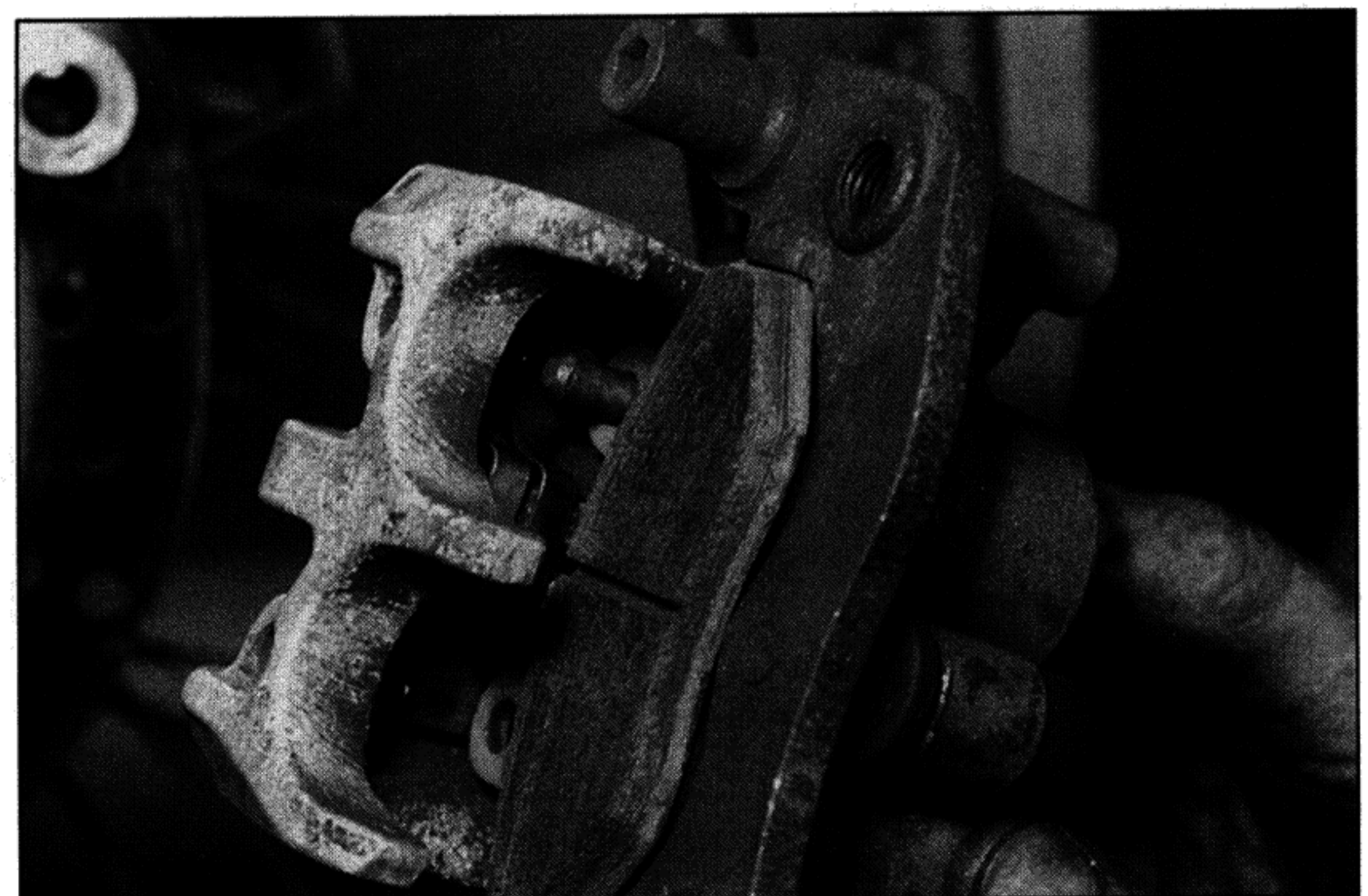
2.11b Locate the outer pad into the caliper as shown
