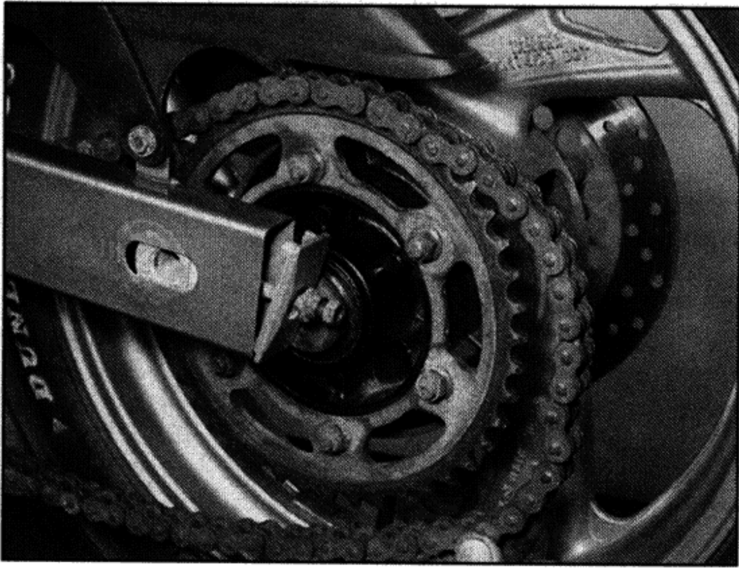
12.10 Manoeuvre the wheel into position and fit the chain onto the sprocket
