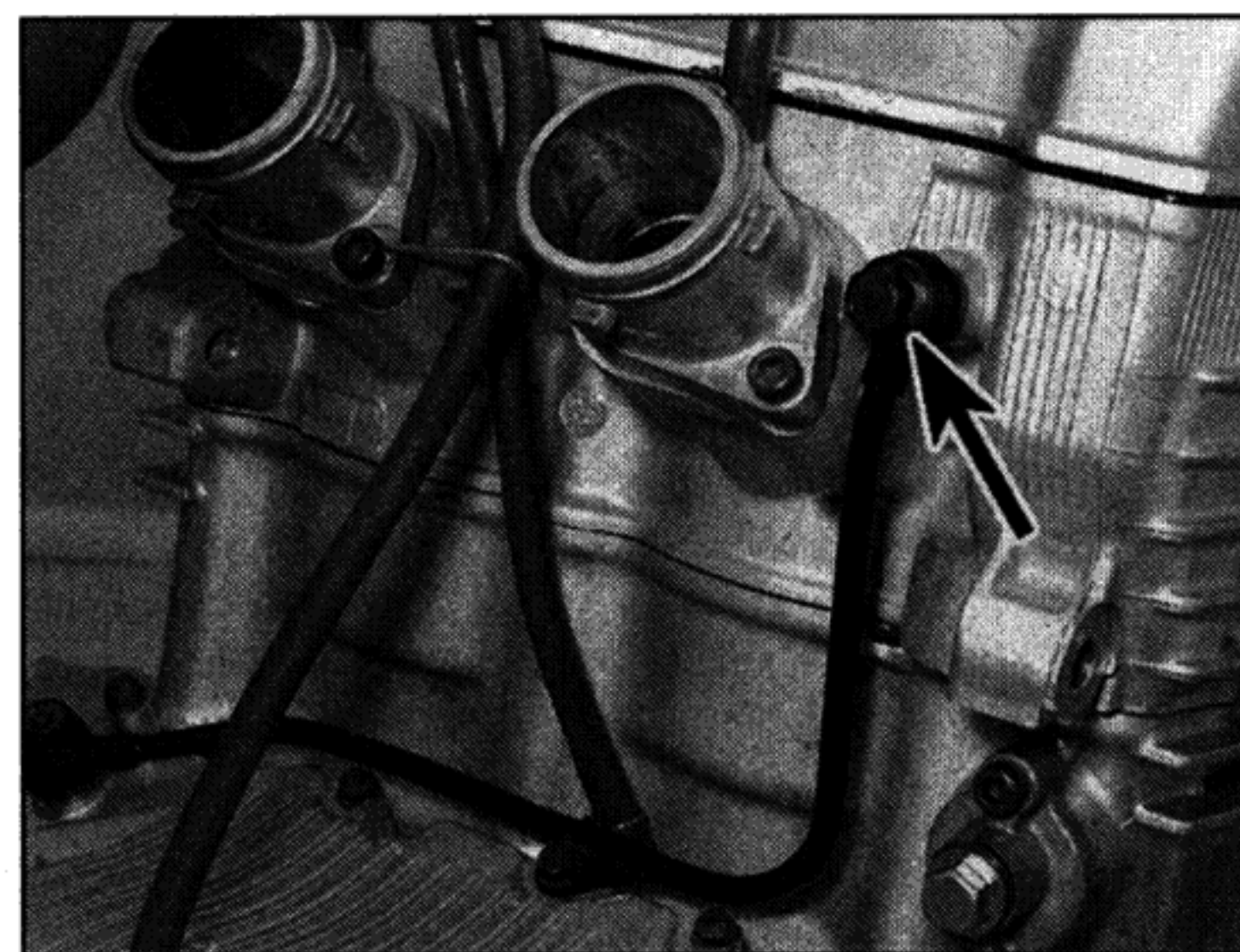
10.5 Unscrew the banjo bolt (arrowed) and detach the oil pipe
