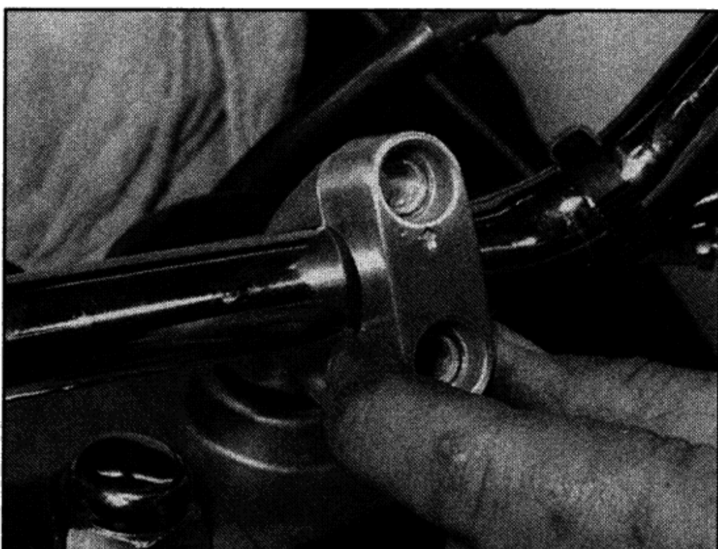
5.8b Fit the clamps with the arrow pointing up . . .
