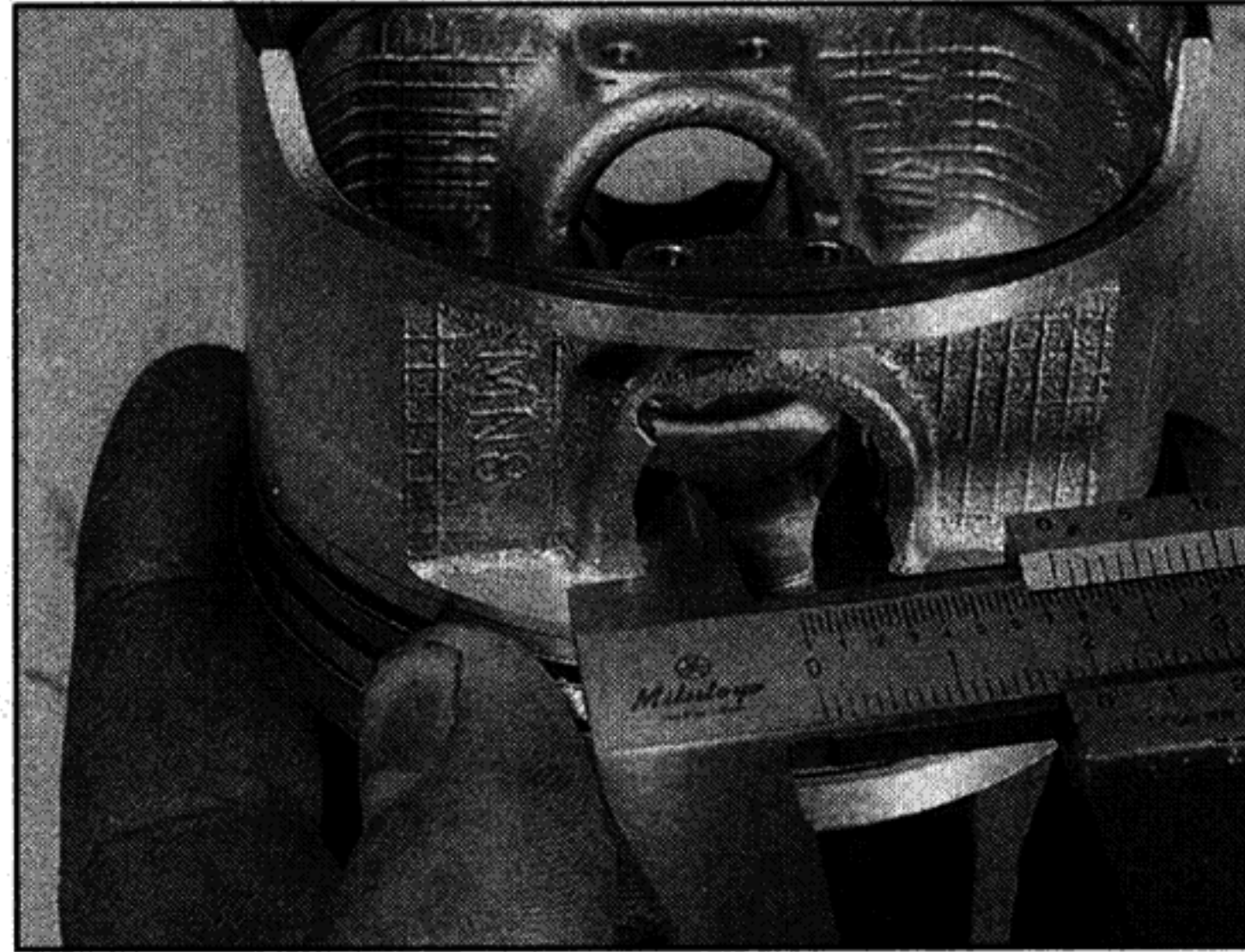
14.13b Measuring the internal diameter of the bore in the piston
