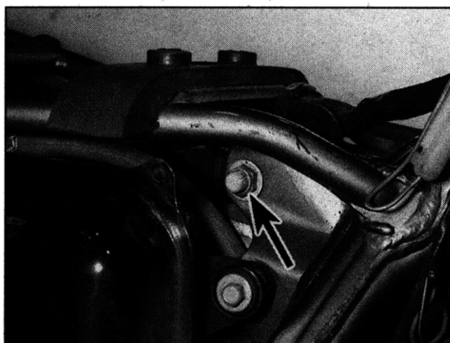
10.9b Shock absorber upper mounting bolt (arrowed) – XTZ models
