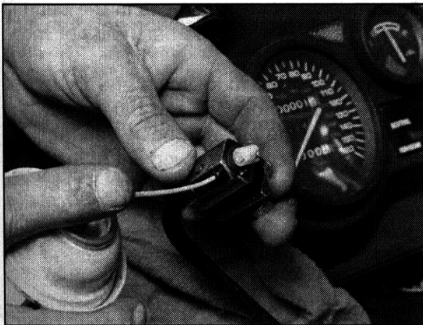
18.3a Lubricating a cable with a cable oiler clamp
