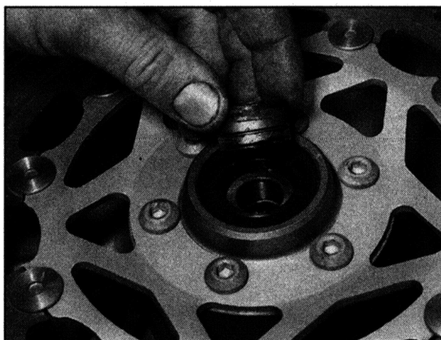
11.7a Remove the spacer ...
