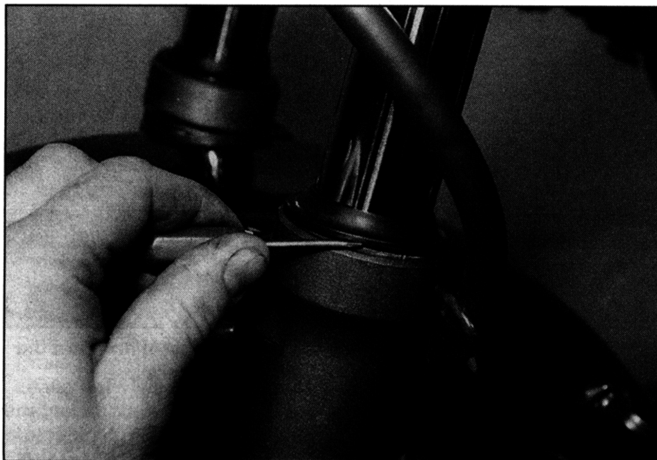
20.3 Check above and below the dust seal for signs of fluid leakage
