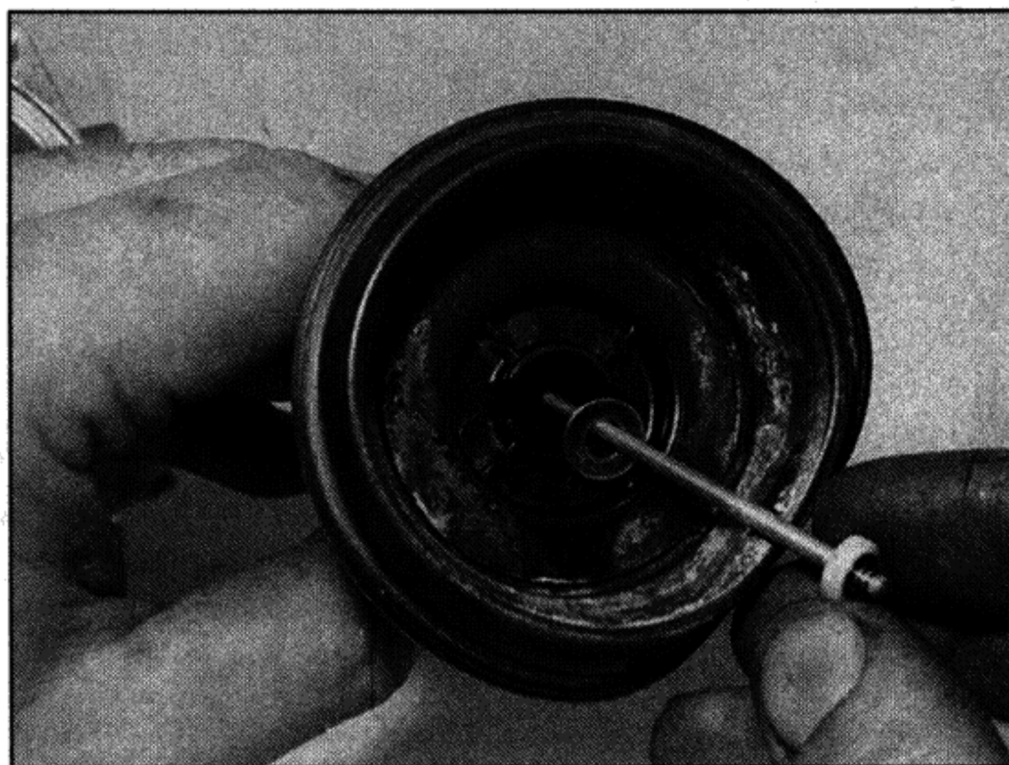
8.5 Remove the jet needle and its washer
