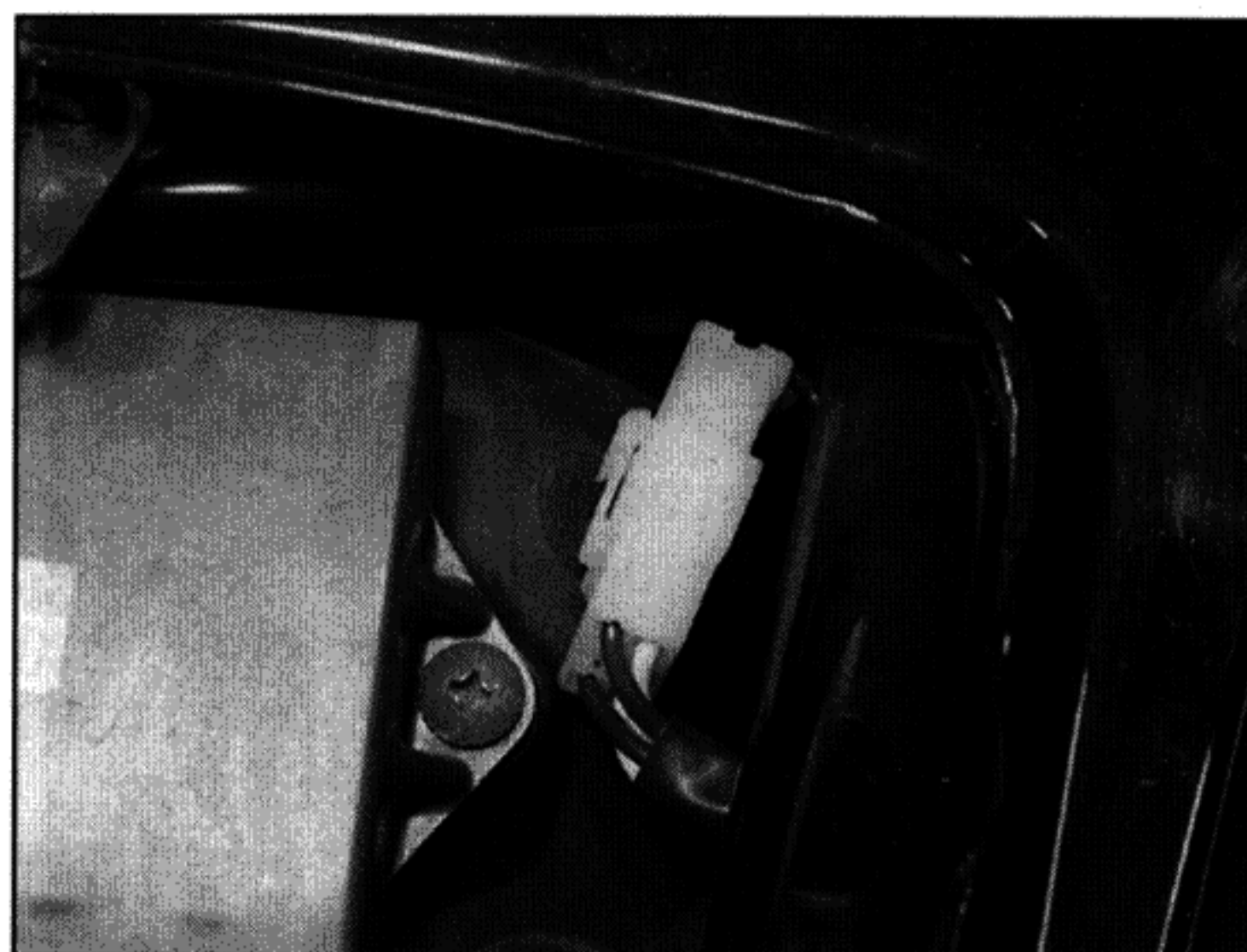
33.4b Regulator/rectifier wiring connector – TRX models
