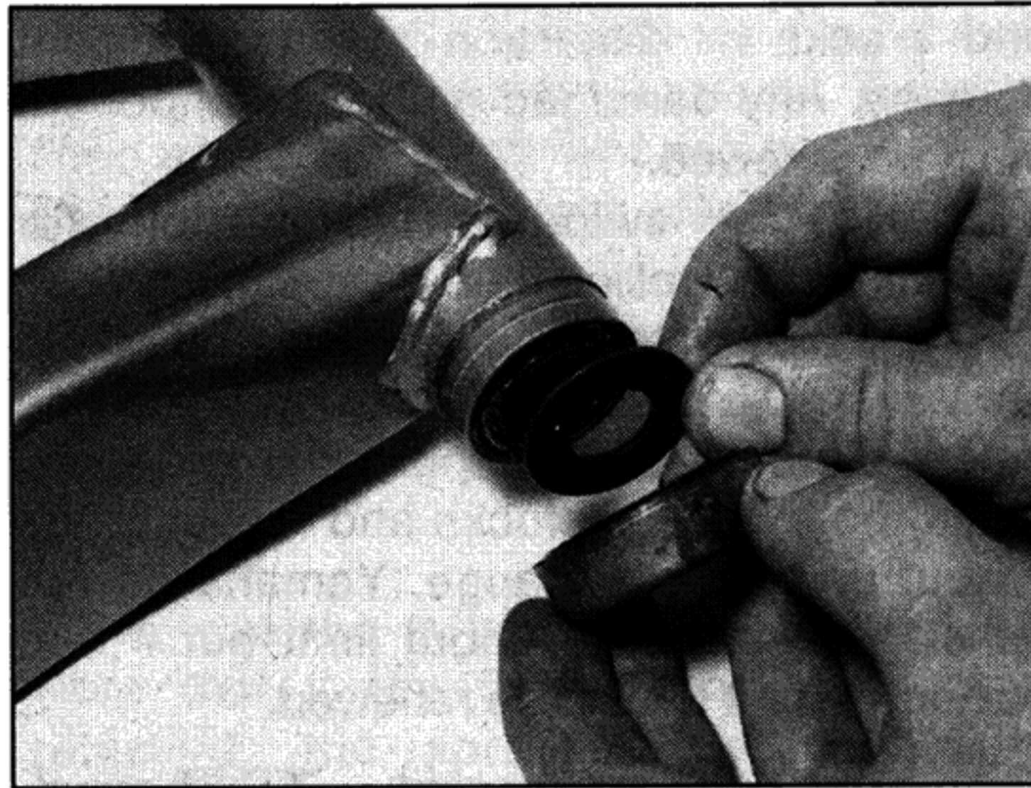
13.14a Remove the cap and washer (where fitted) . . .
