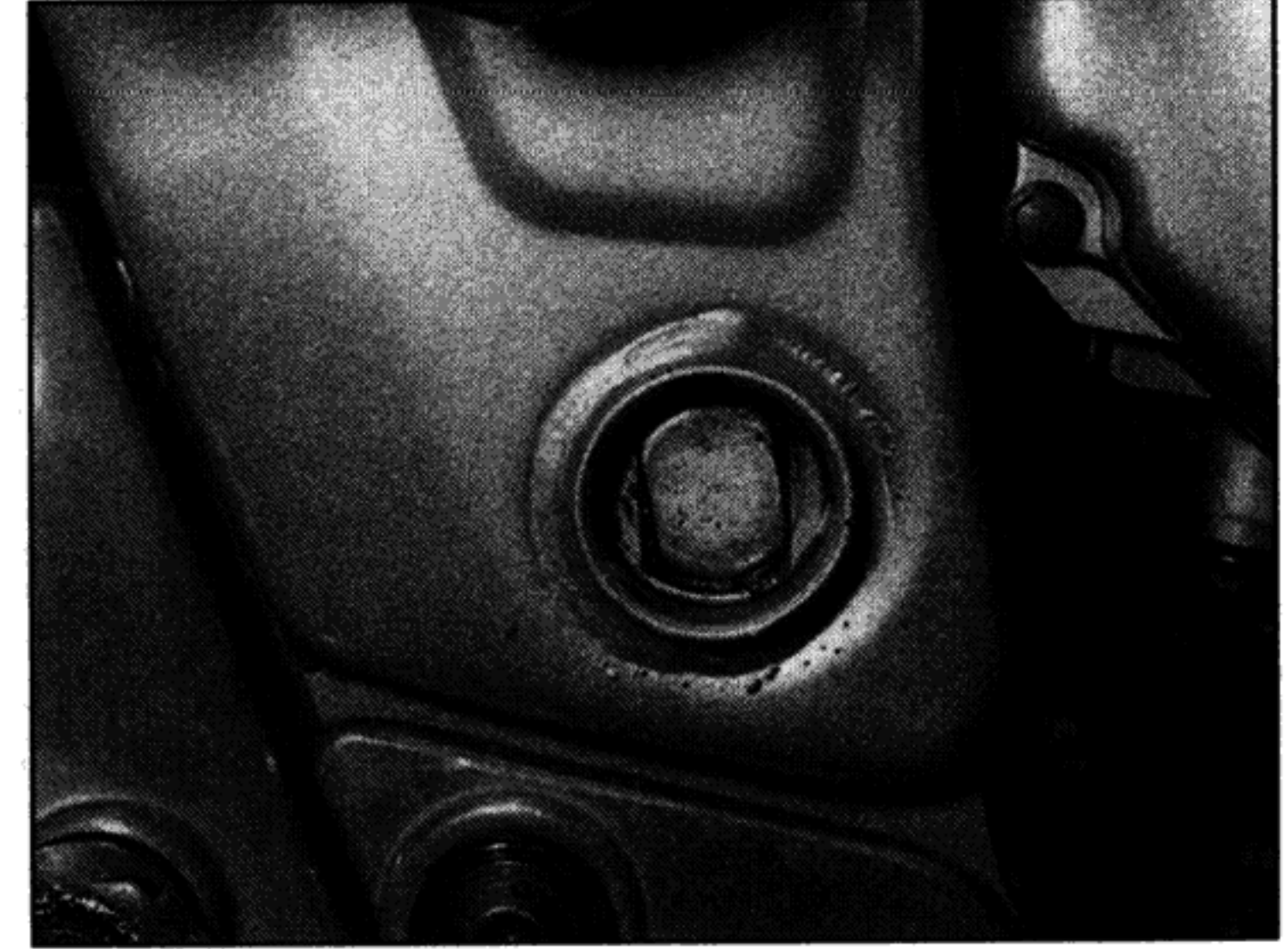
13.15b On TDM models, make sure the bolt head flats locate correctly
