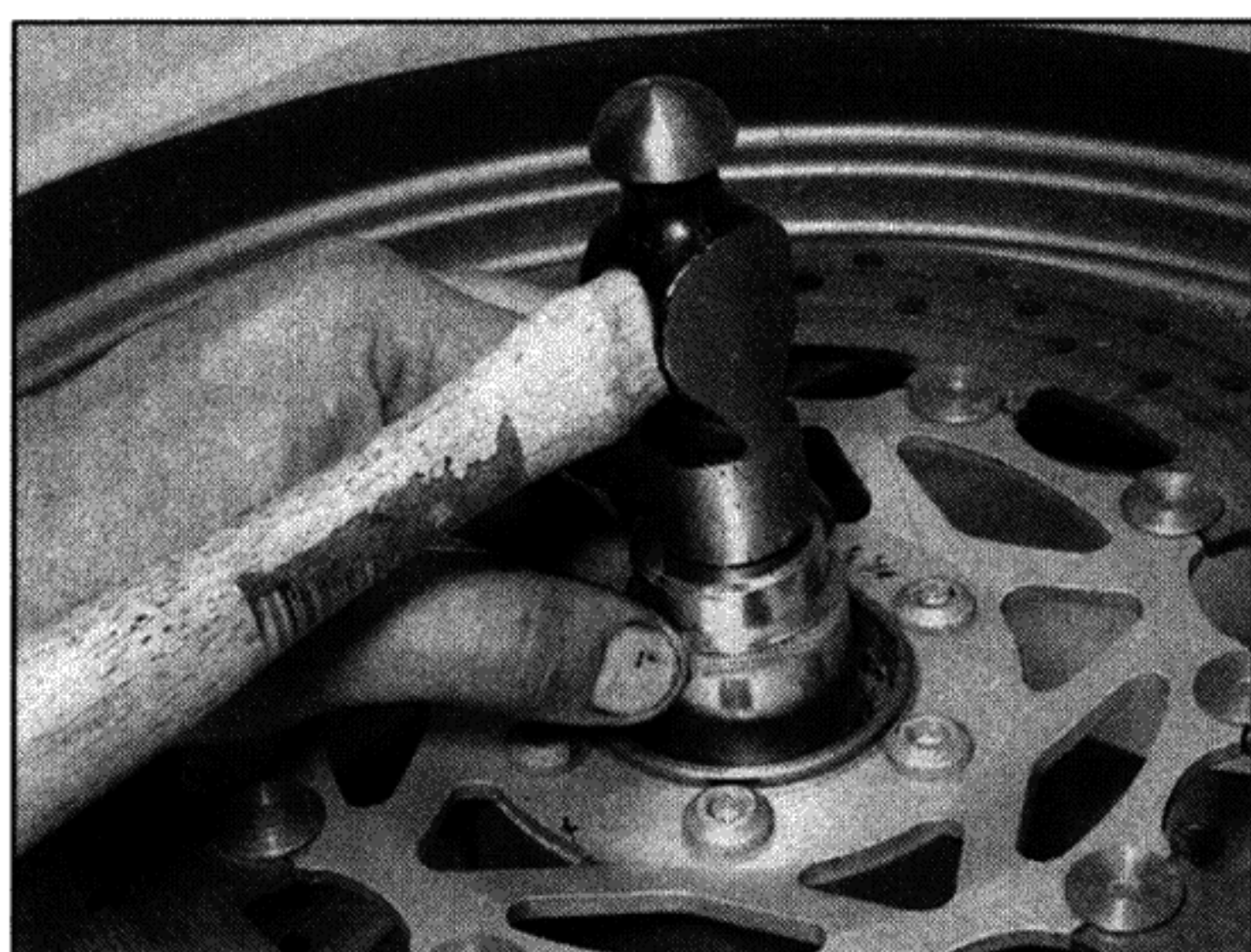
13.10 A socket can be used to drive in the bearing
