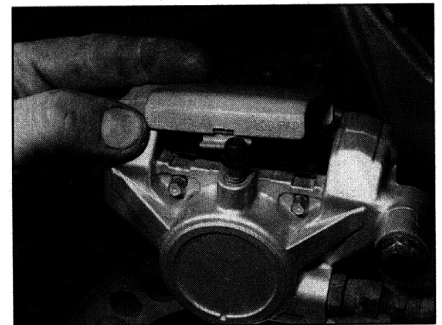
2.10 Clip the cover onto the caliper, making sure it is secure
