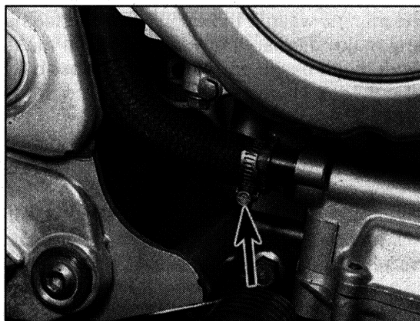
5.19b Slacken the clamp screw (arrowed) and detach the hose
