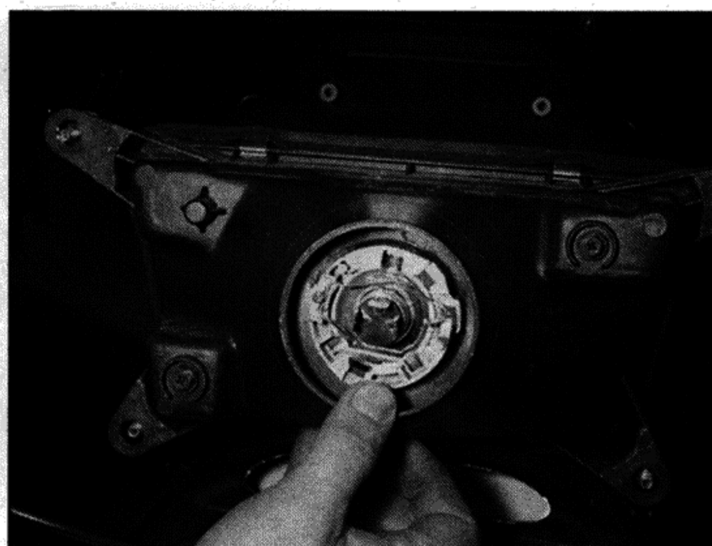
8.2a Removing the headlight – TRX models
