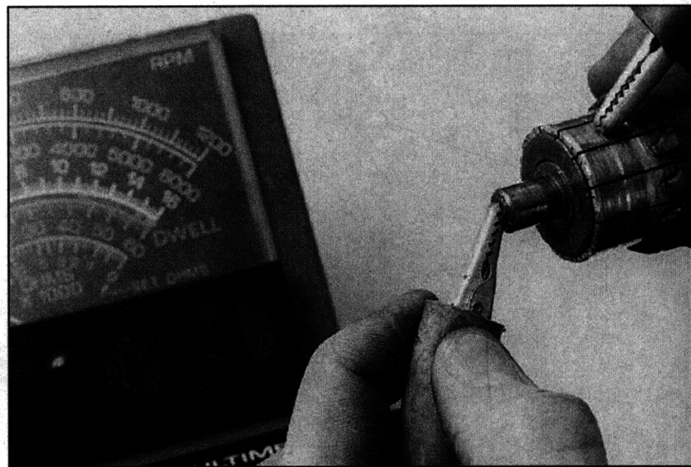
29.10b There should be no continuity between the commutator bars and the armature shaft
