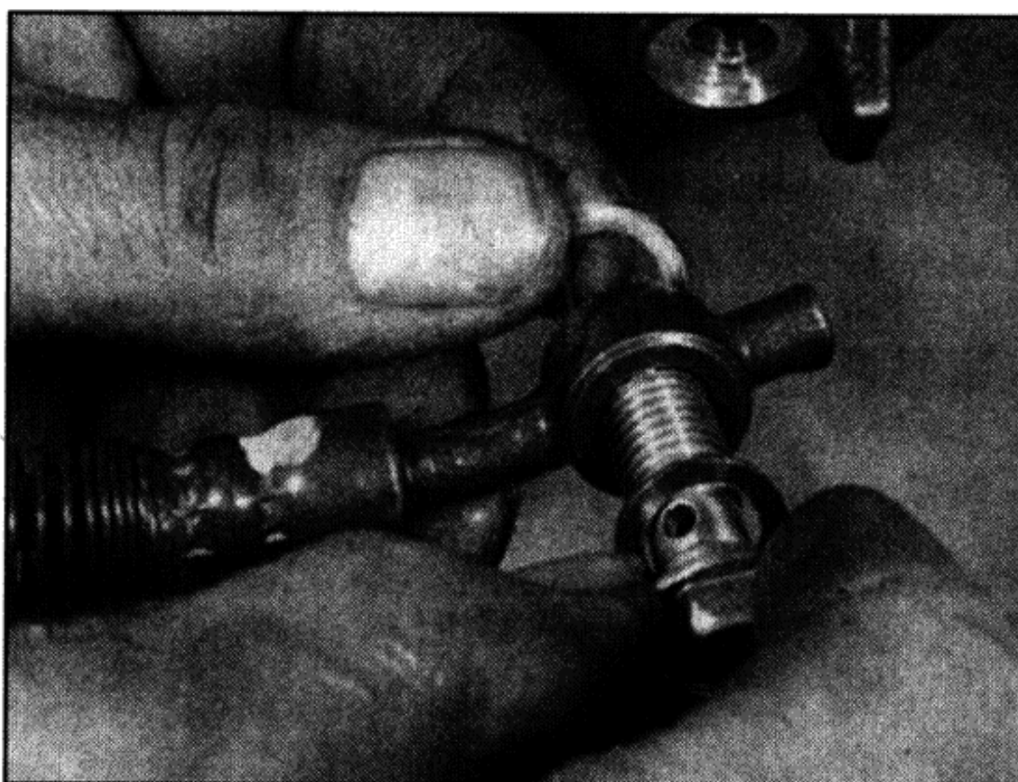
7.4 Remove the banjo bolt and separate the hose from the caliper; there is a sealing washer on each side of the fitting
