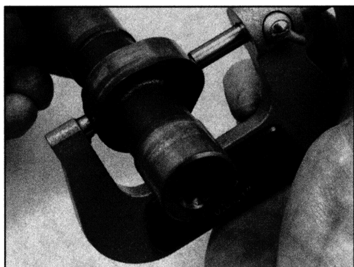
8.12b Measure the height of the camshaft lobes with a micrometer
