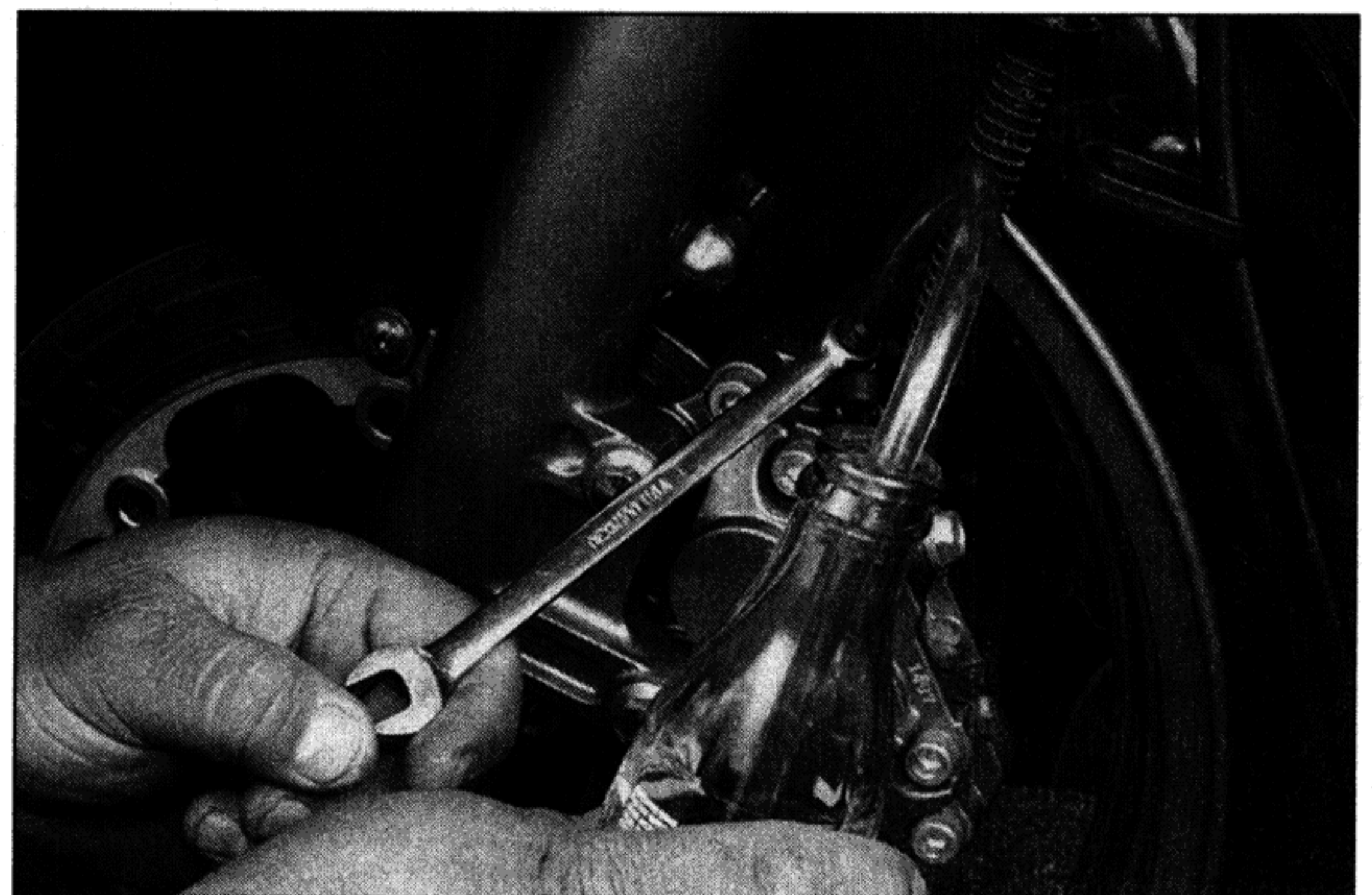
8.6b To bleed the brakes, you need a spanner, a short section of clear tubing, and a clear container half-filled with brake fluid
