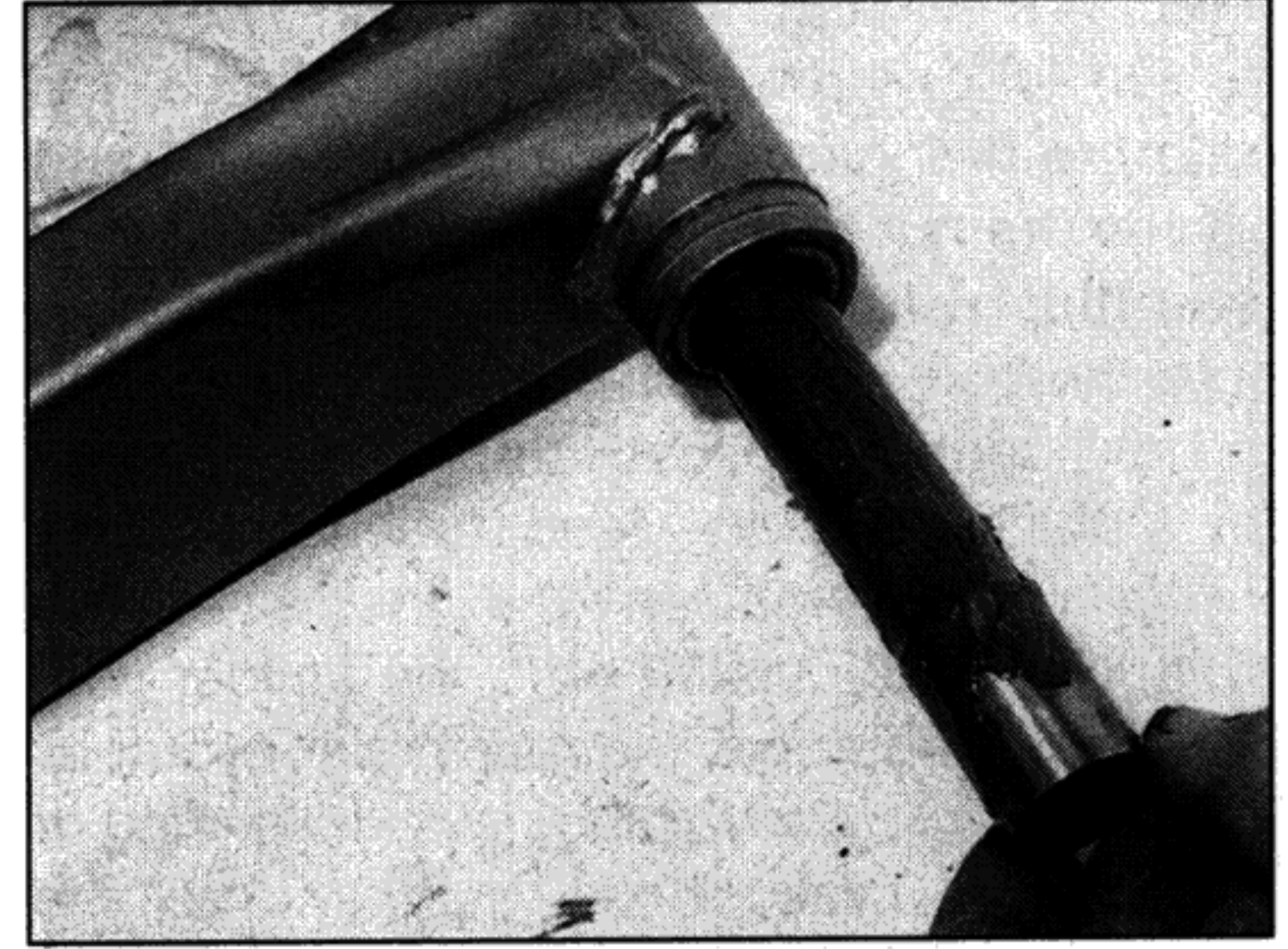
13.14b . . . then withdraw the collar . . .
