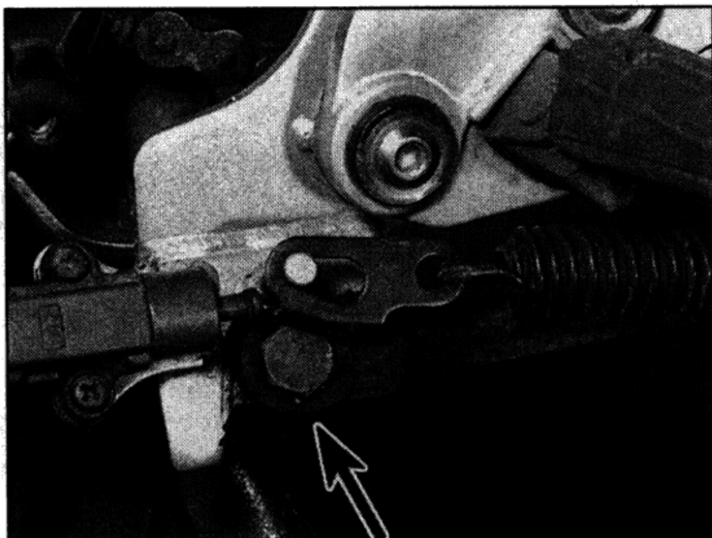
4.2 Sidestand pivot bolt (arrowed) – TDM models
