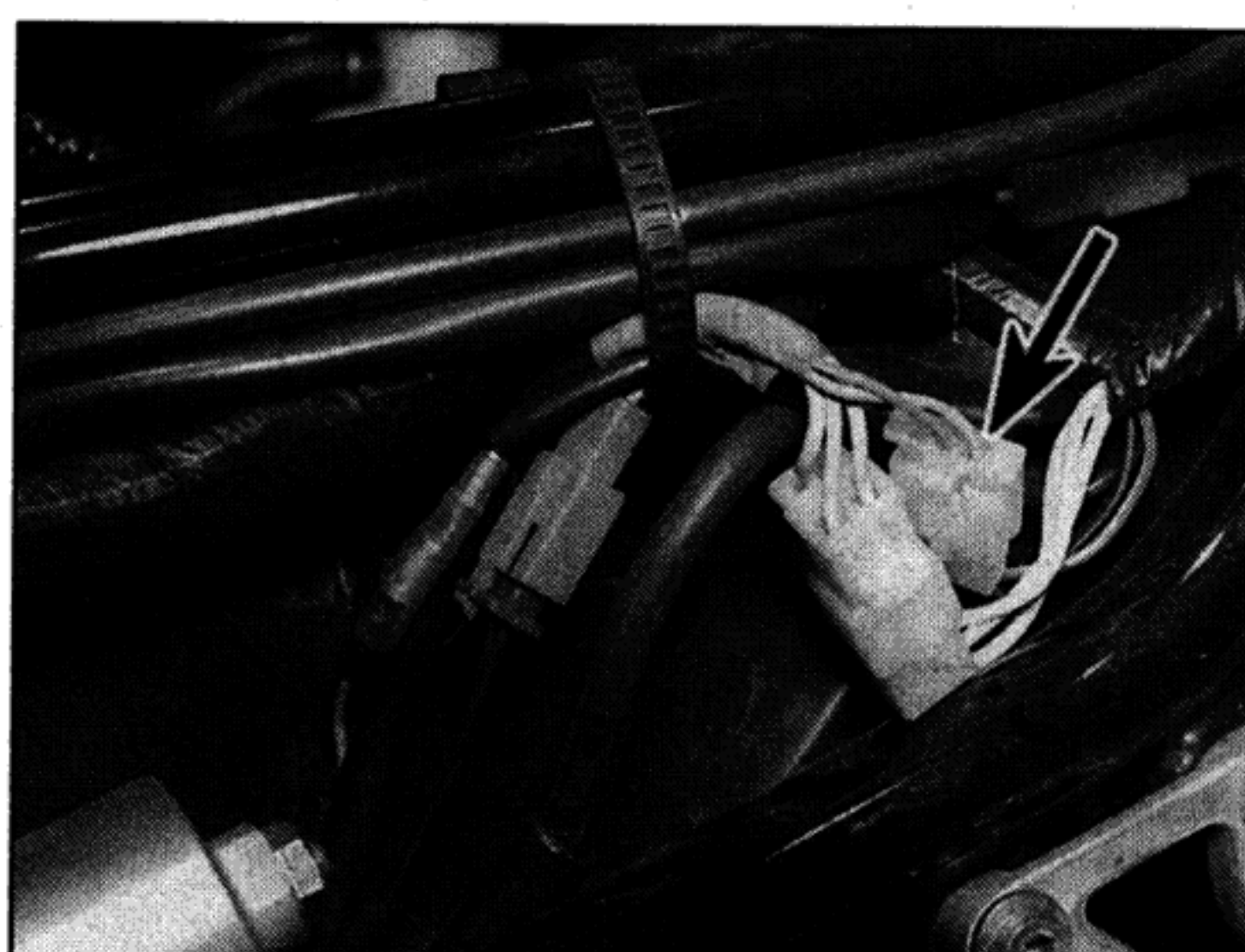
4.3b Pick-up coil wiring connector (arrowed) – TRX models
