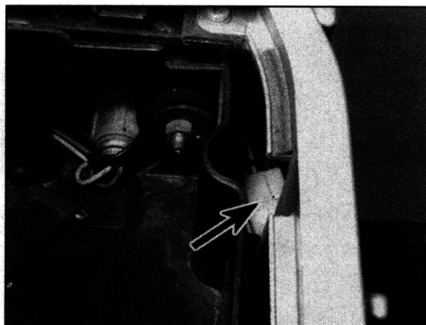
10.2b Tail light wiring connector (arrowed) – XTZ models
