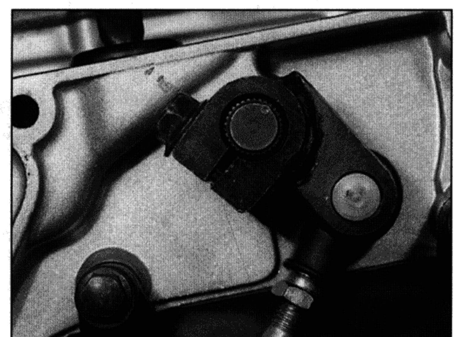
32.6b Gearchange arm/shaft alignment – TDM models
