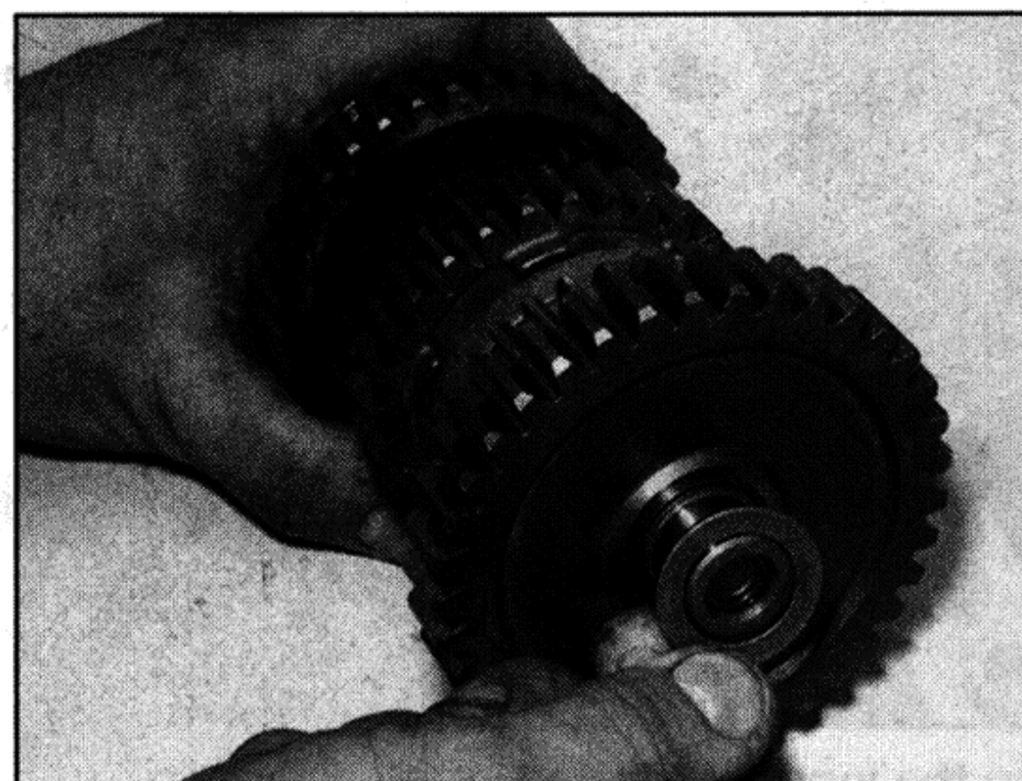
31.40c ... the thrust washer ...
