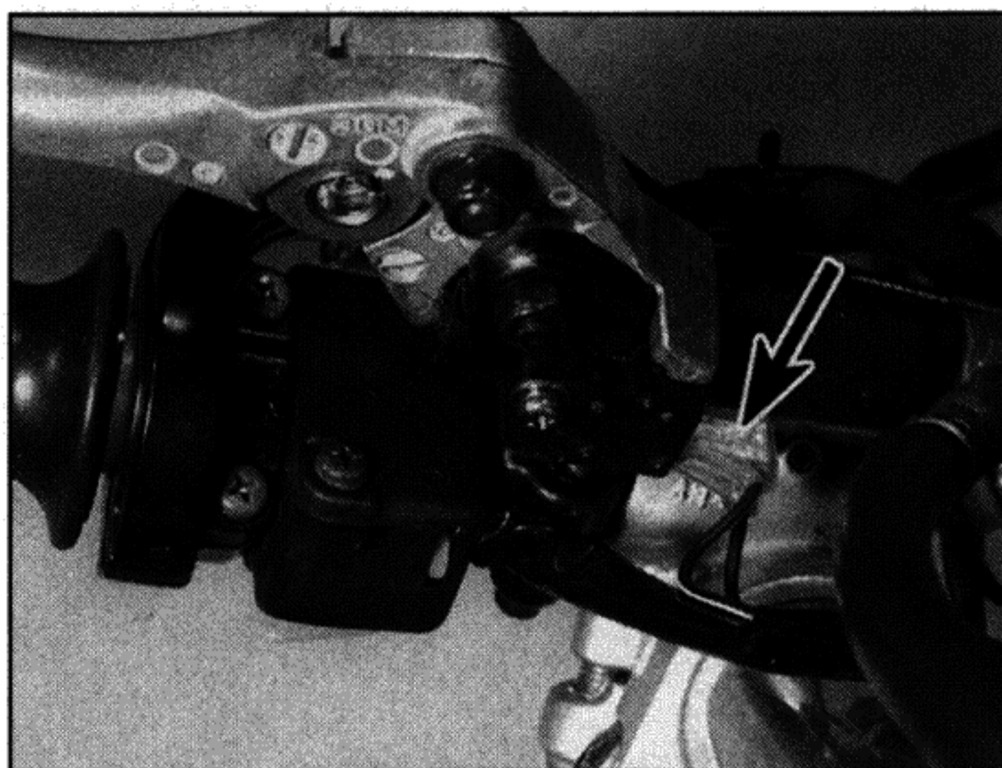
5.4b Brake switch wiring connectors (arrowed) – TRX models
