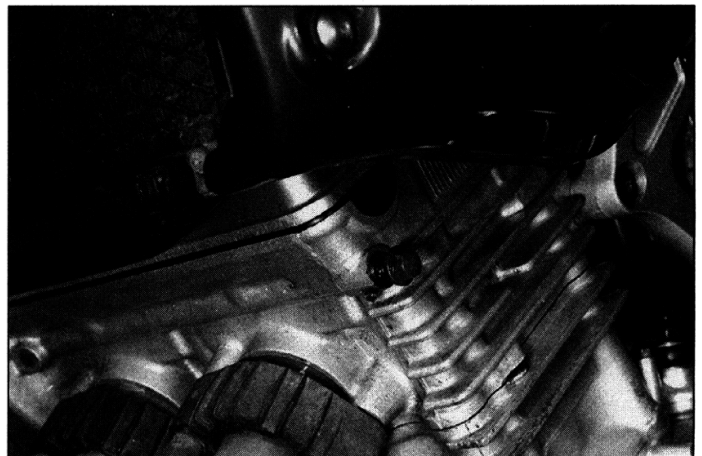
32.4 . . . then start the engine and check that the oil dribbles out within a minute
