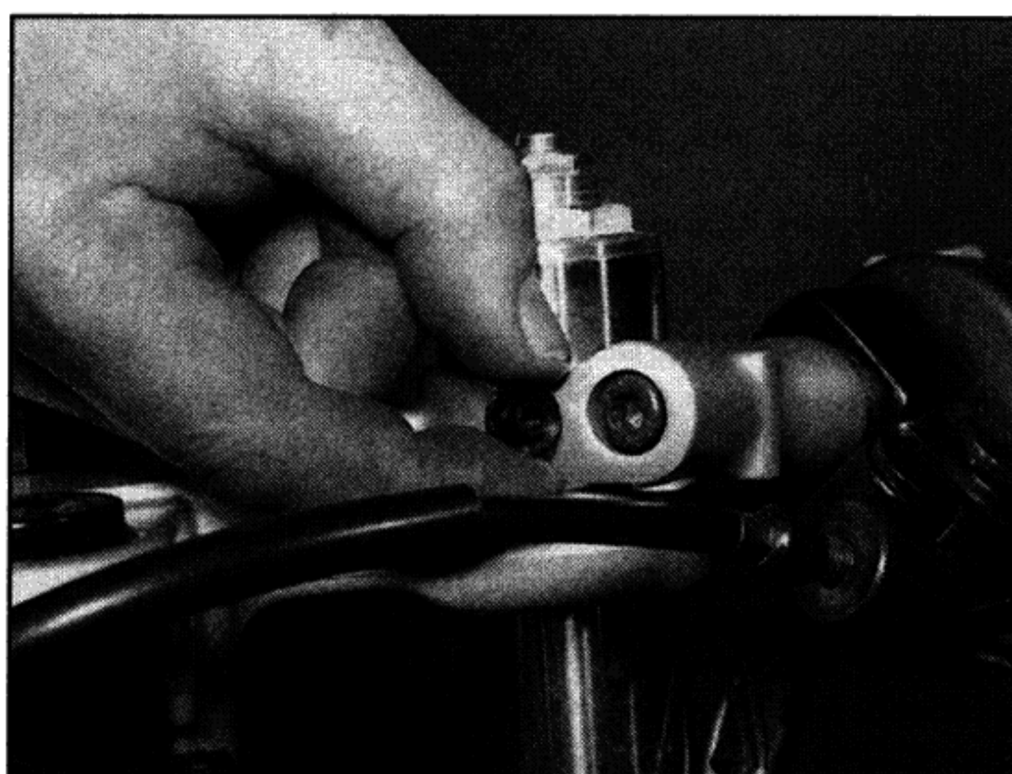
5.6 Remove the cap to access the bolt
