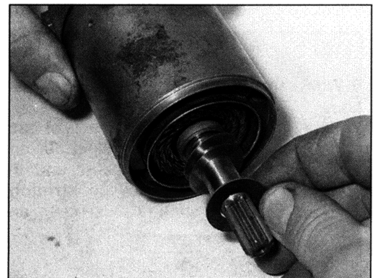
29.4b . . . and slide off the shims
