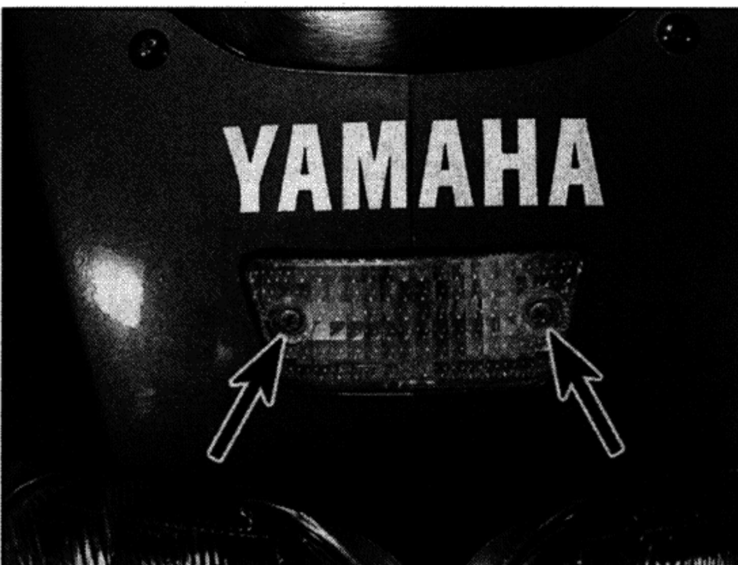
7.7a Remove the screws (arrowed) and the lens ...
