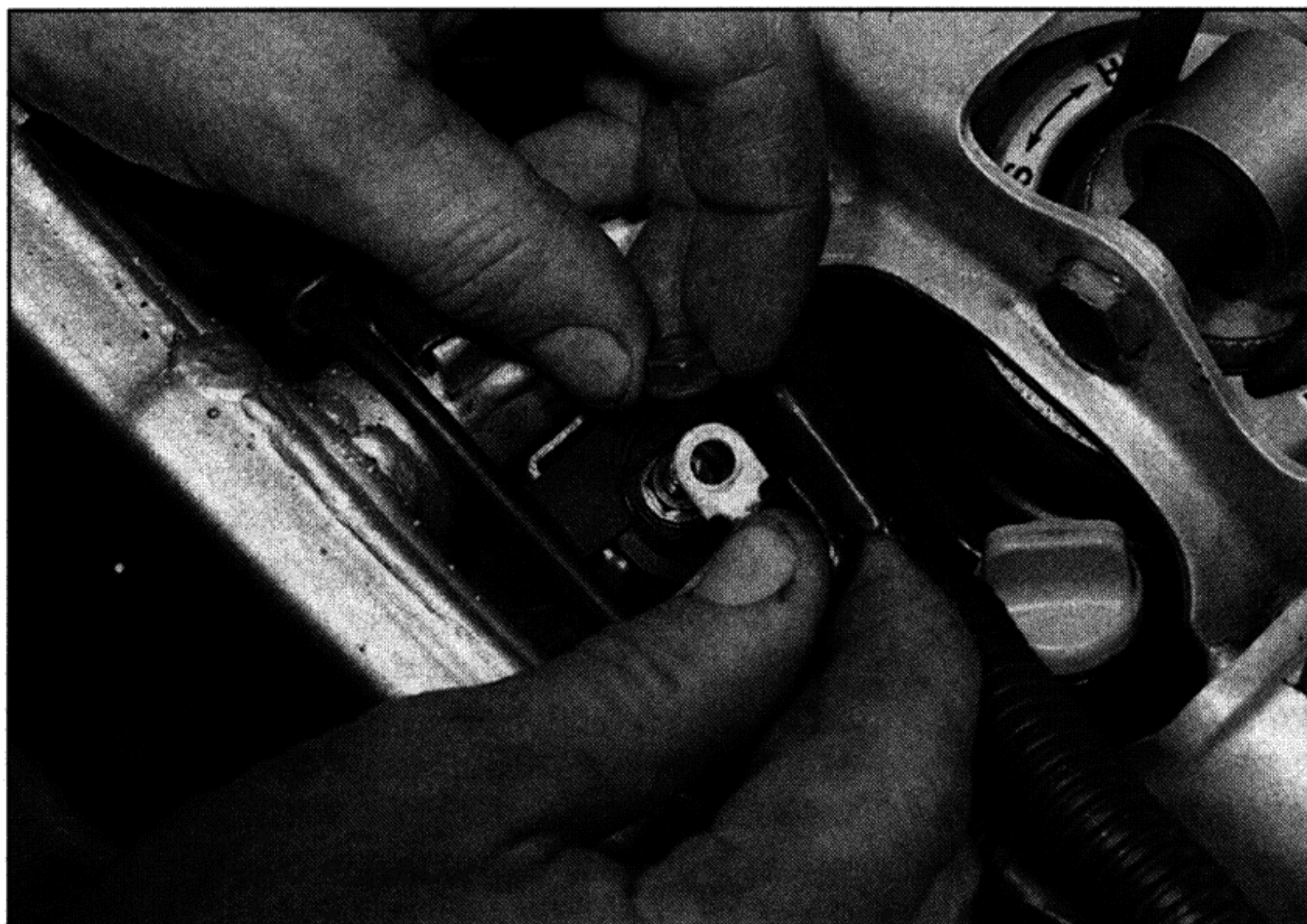
5.14 Unscrew the nut and detach the starter motor lead from the starter relay
