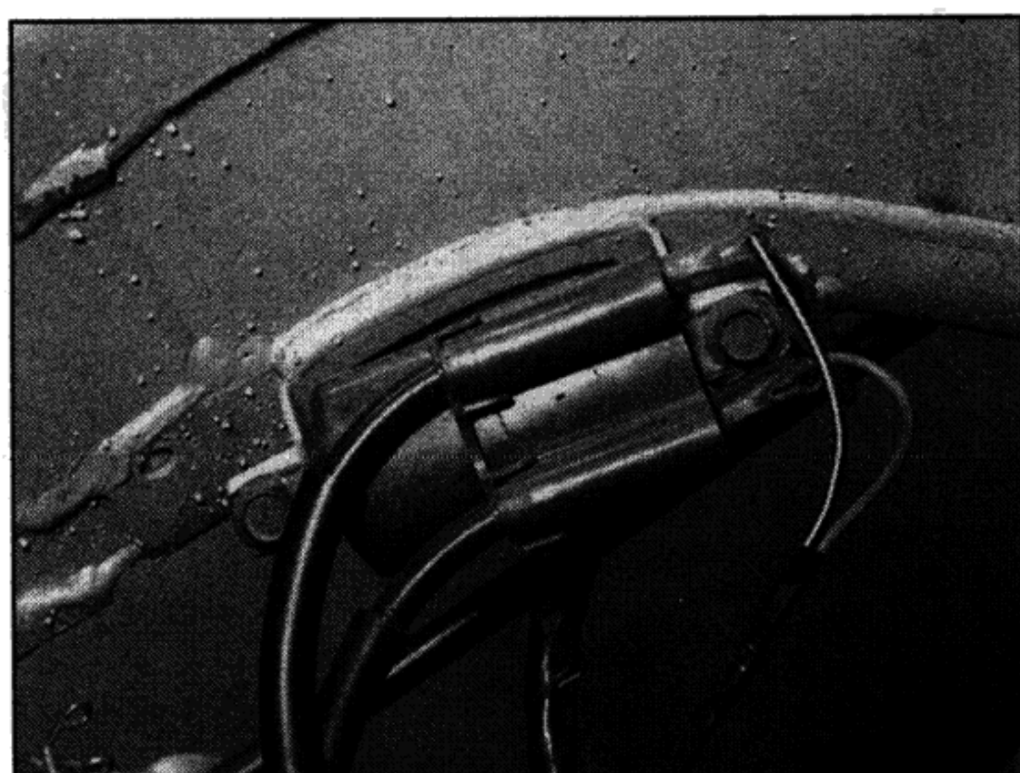
3.4a Ignition coil – 1991 to 1995 TDM models
