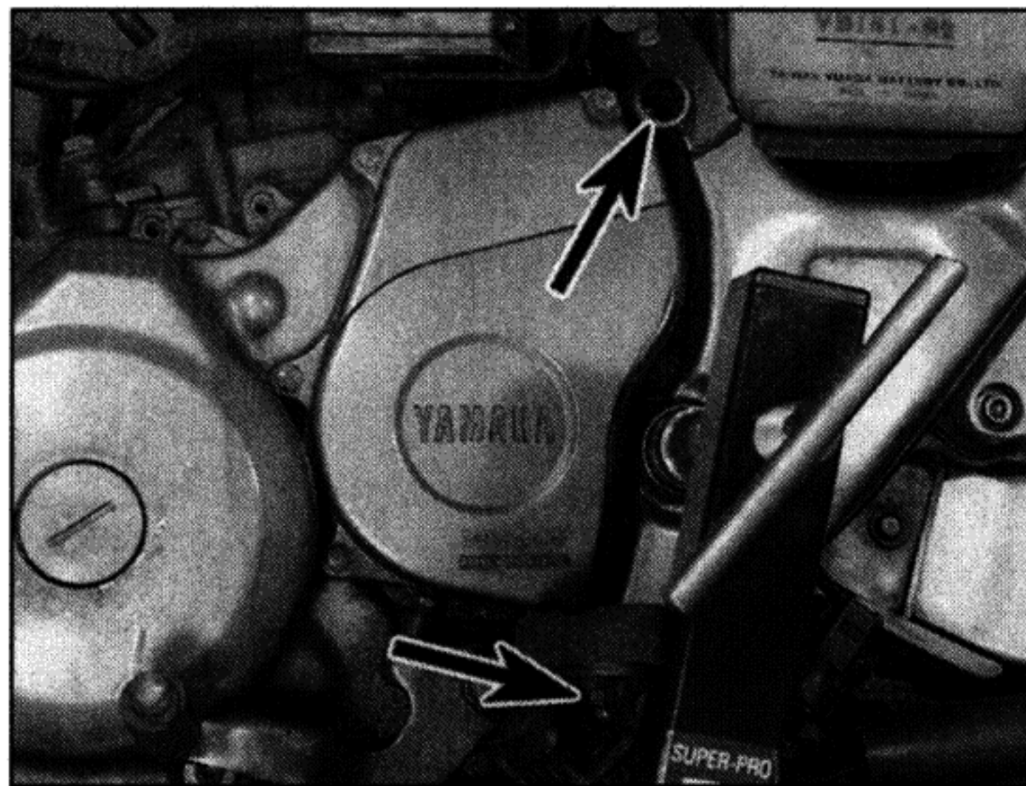
5.23d Upper and lower rear mounting bolts (arrowed)
