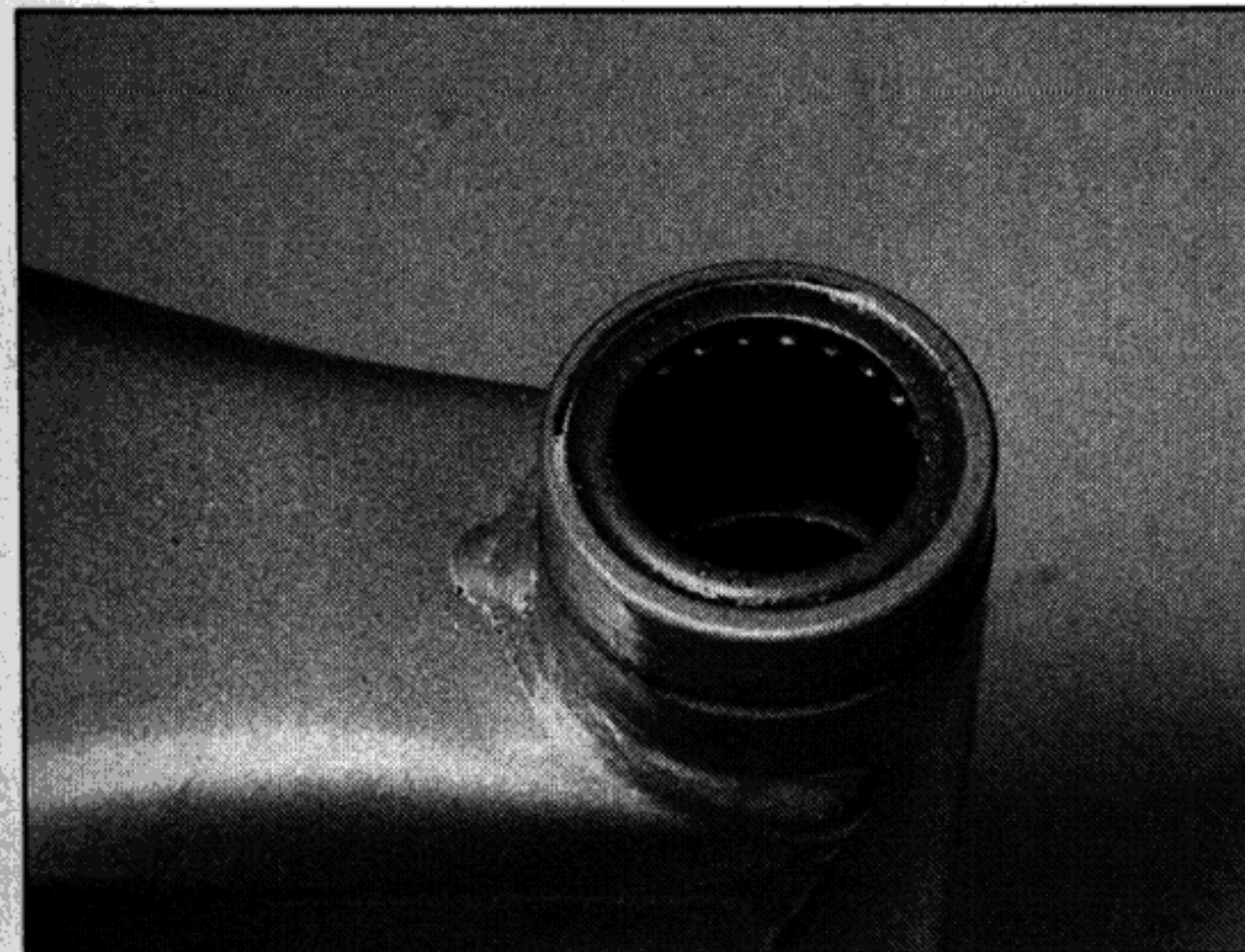
13.14c . . . and grease the bearings and other components as described
