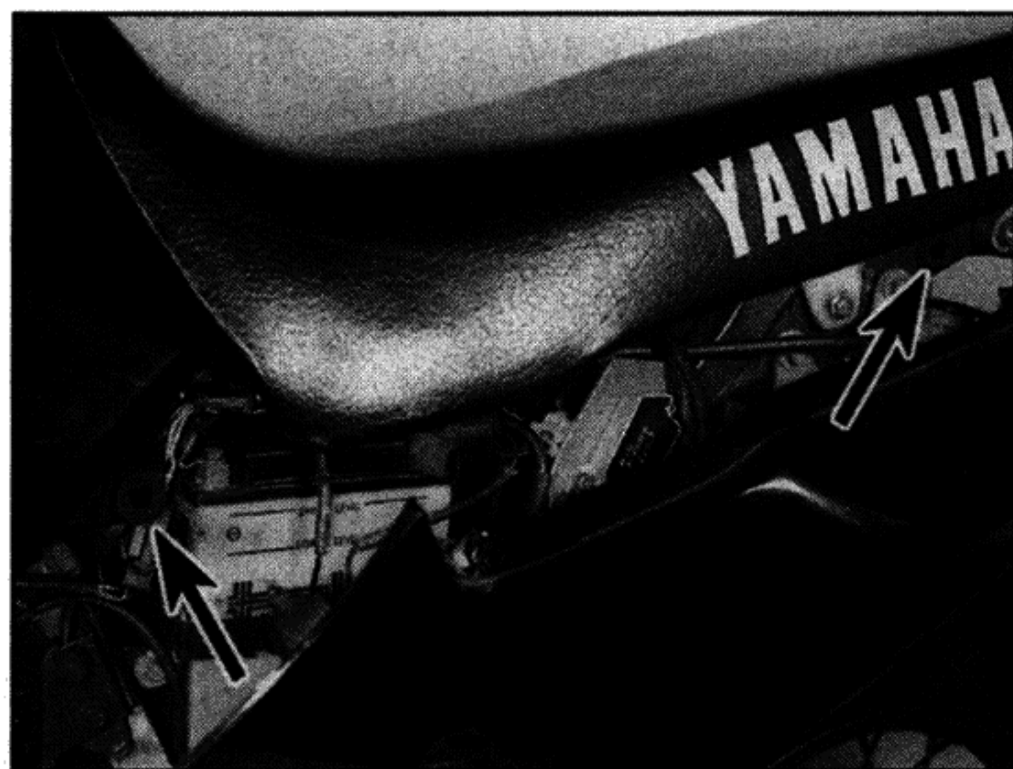
3.7b ... then draw the cover away to release the pegs from the grommets (arrowed)
