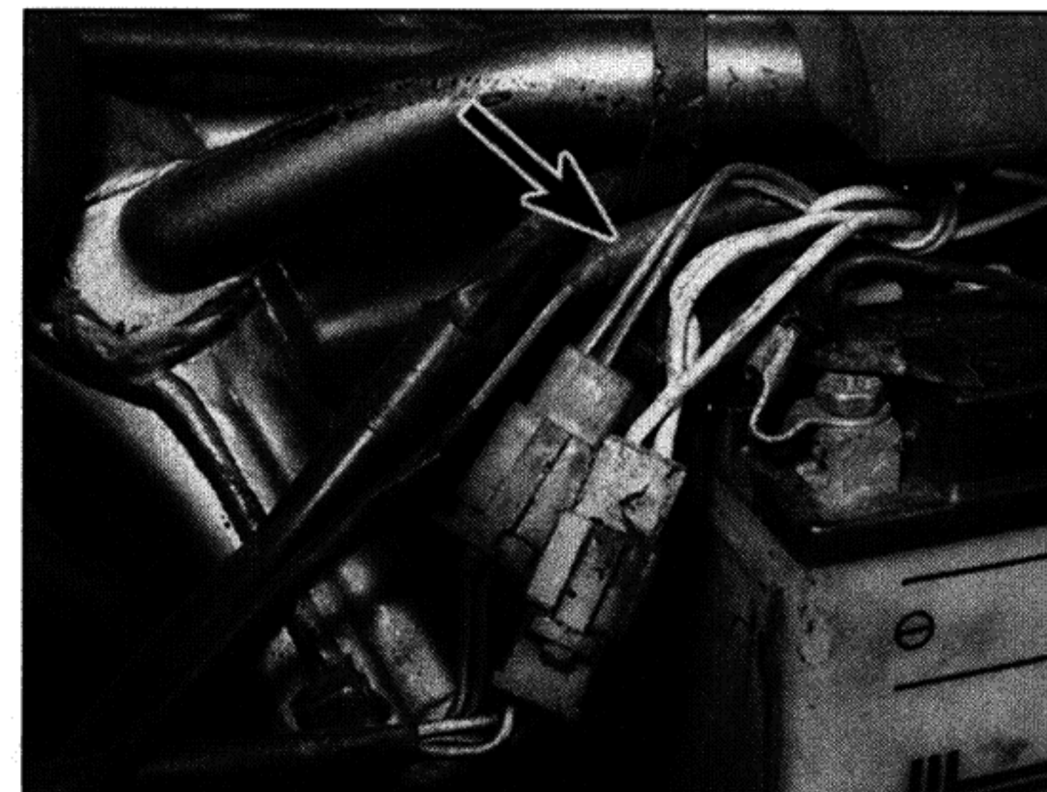
21.2c Neutral switch wiring connector (arrowed) – XTZ models
