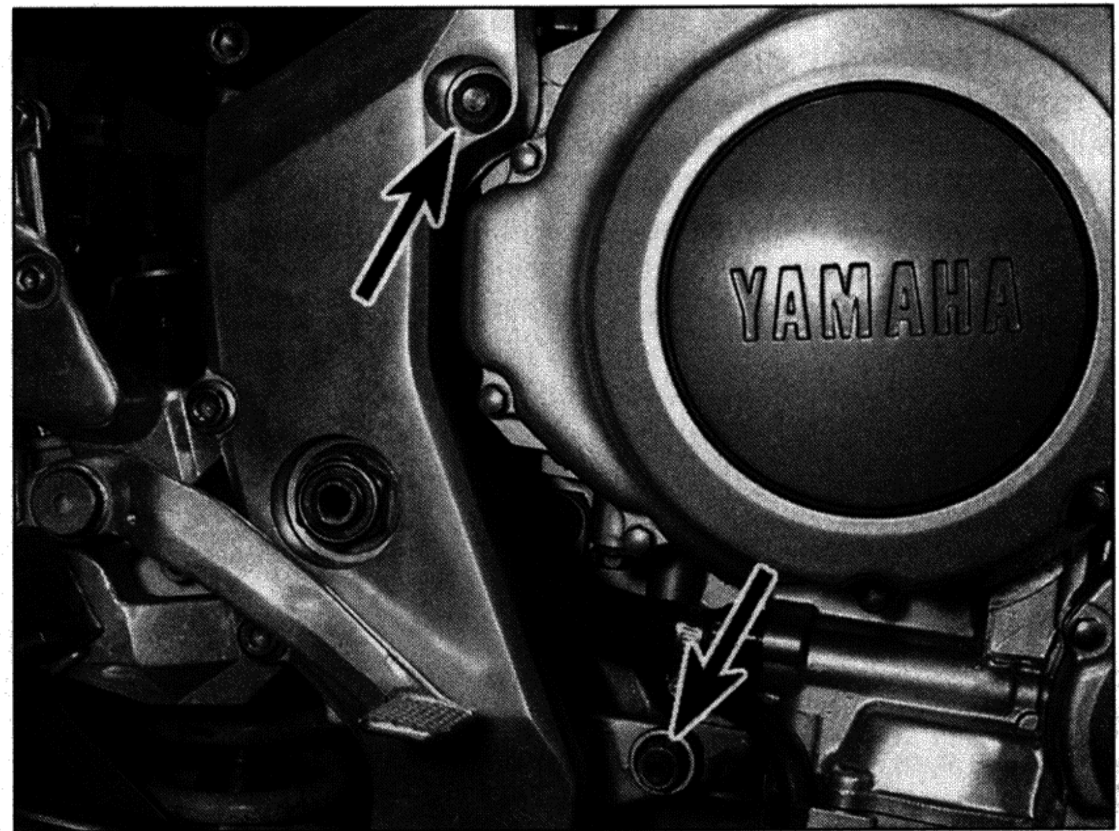
5.22c Upper and lower rear mounting bolts (arrowed)
