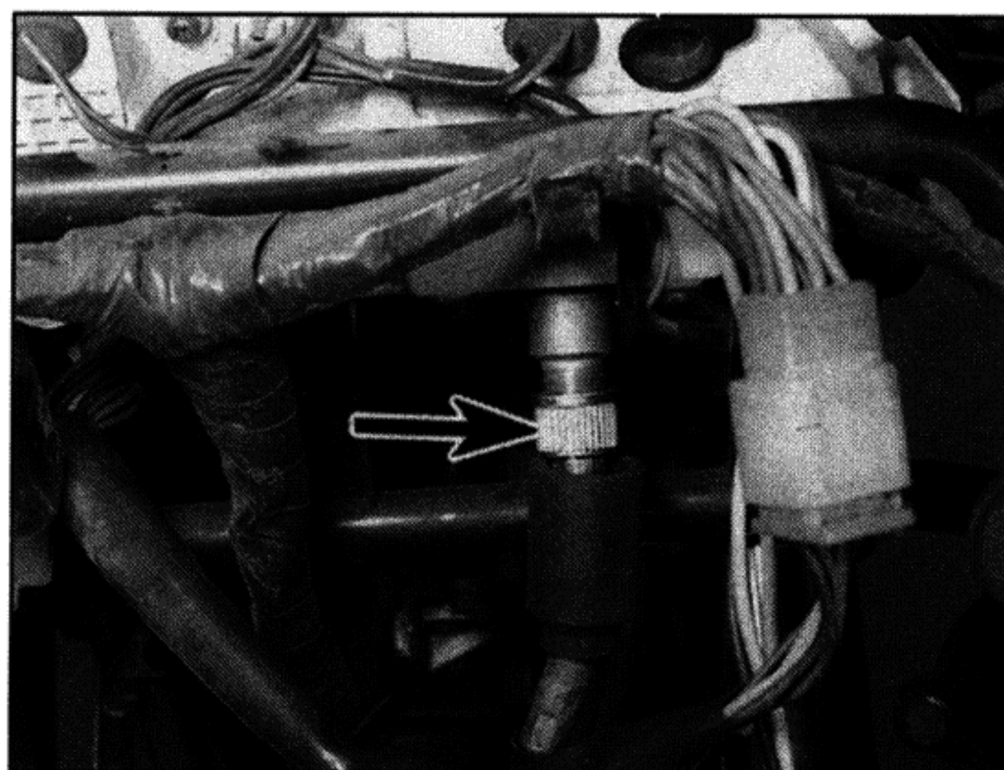
15.6a Unscrew the ring (arrowed) (XTZ shown) ...
