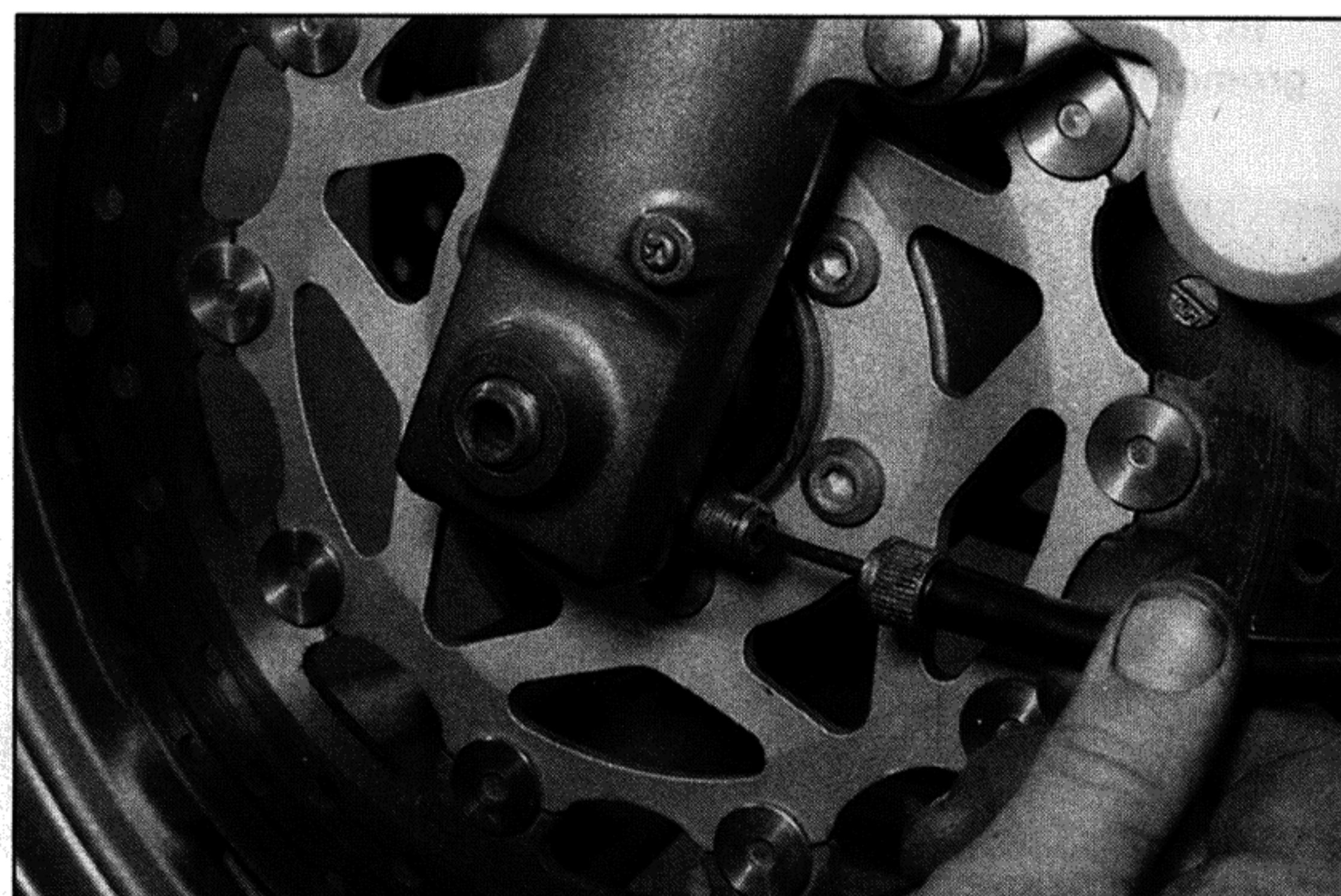
15.7b ... and detach the cable
