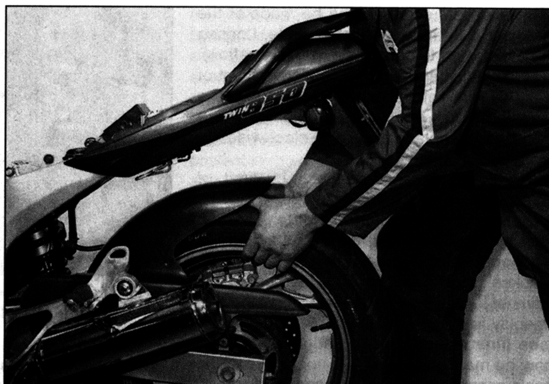
20.7 Checking for play in the rear shock mountings and suspension linkage bearings (TRX and XTZ models)
