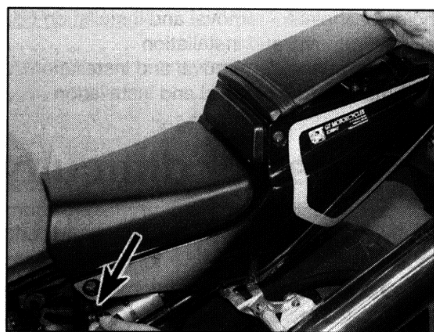
2.6 Turn the key in the lock (arrowed) and remove the passenger seat
