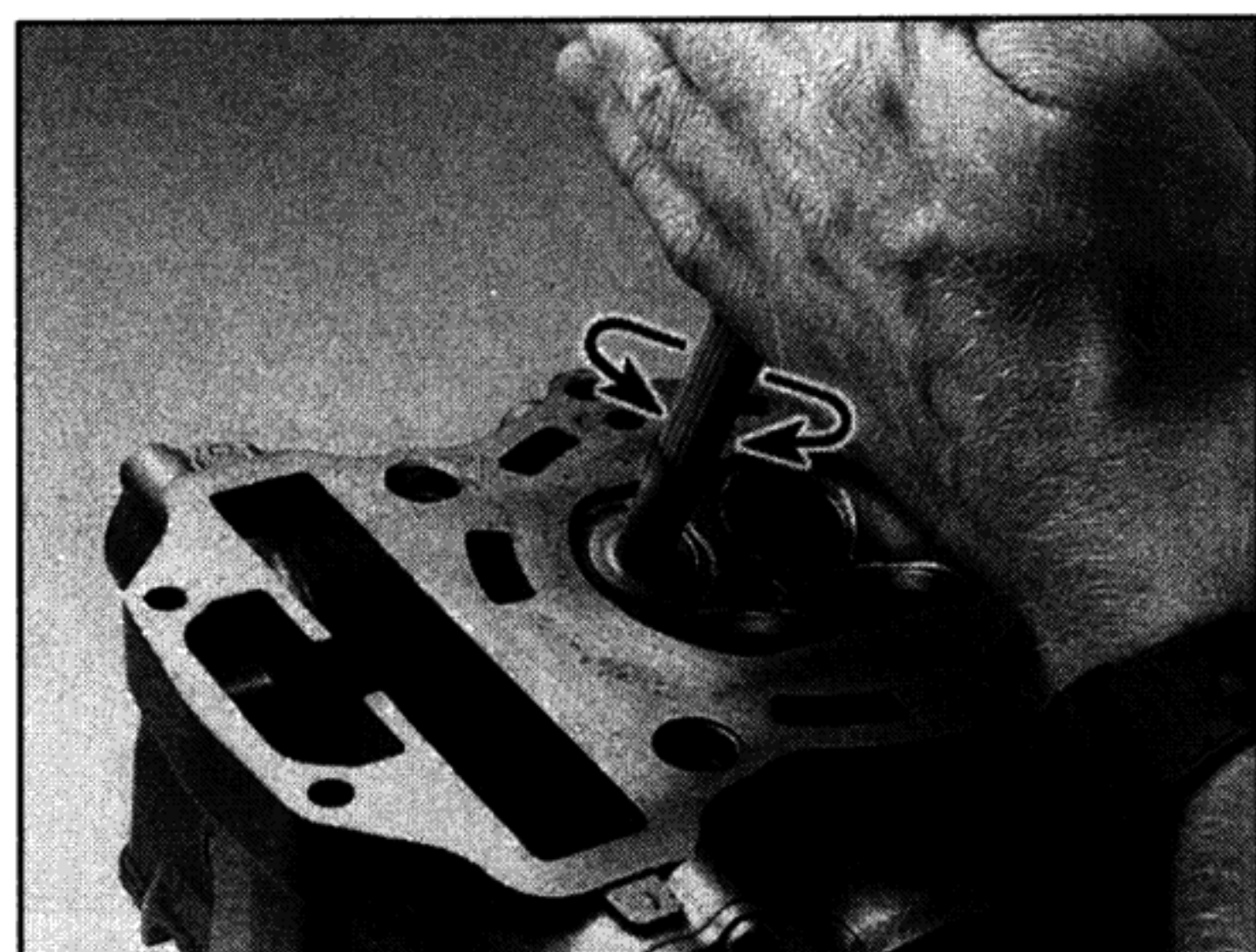
12.22a Rotate the valve grinding tool back and forth between the palms of your hands
