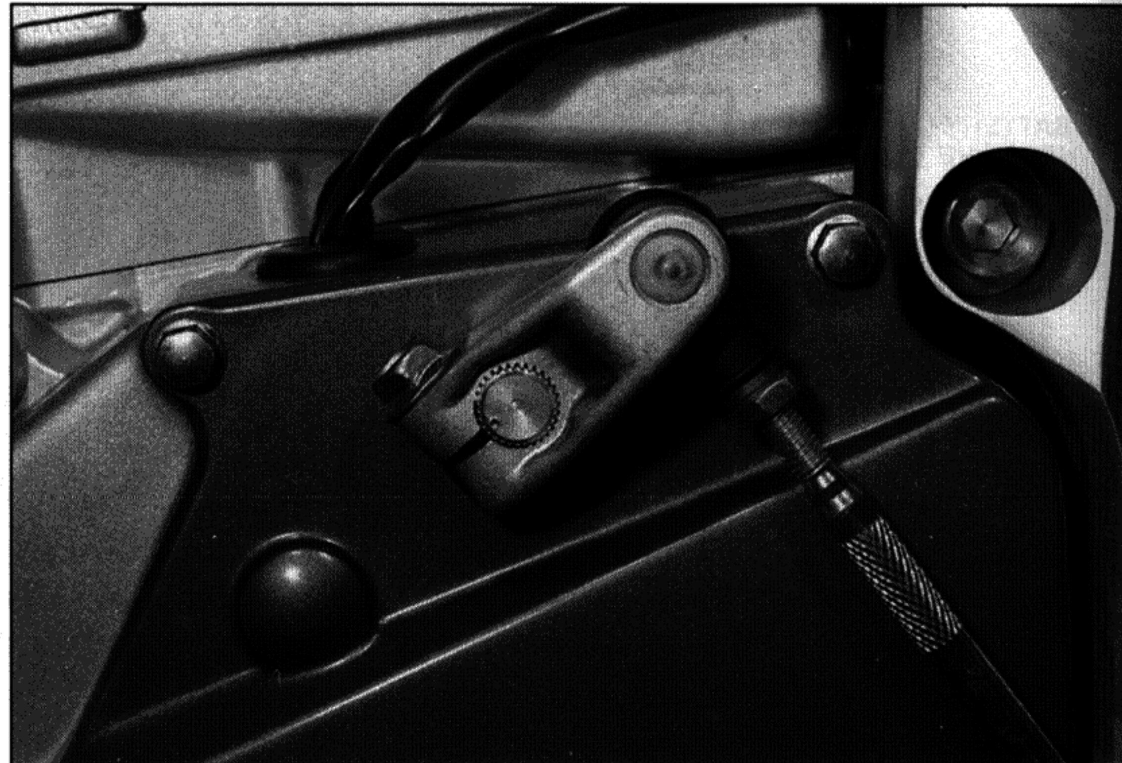
32.7 Gearchange arm/shaft alignment – TRX models
