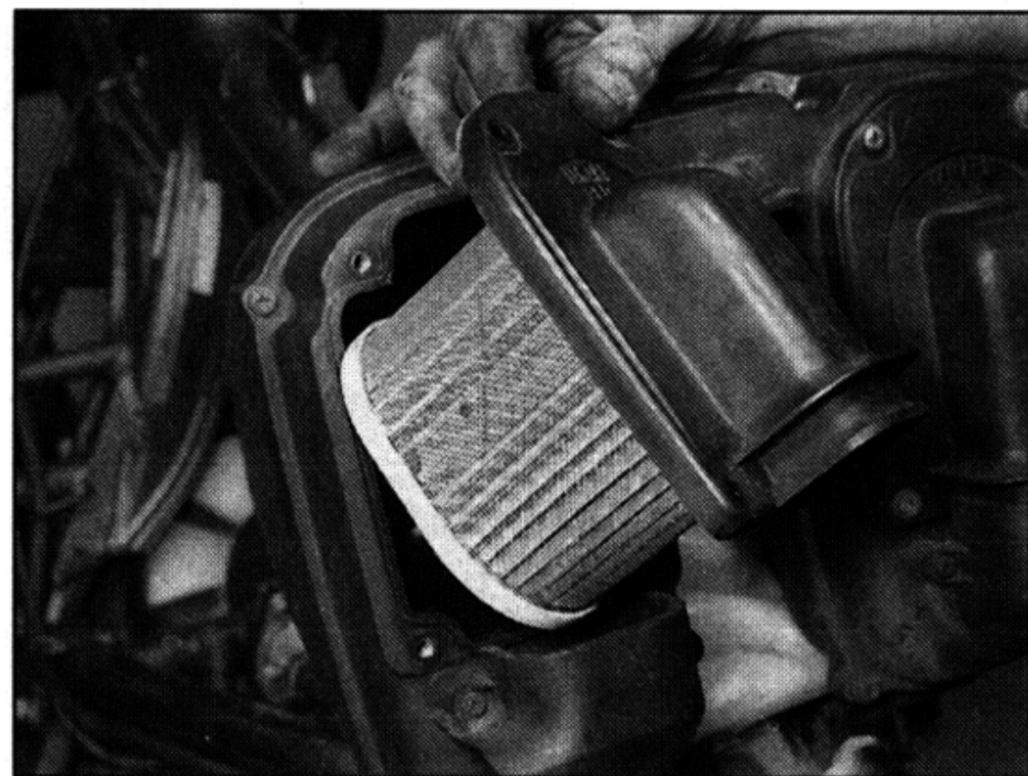
5.3b ... and remove the cover and element together
