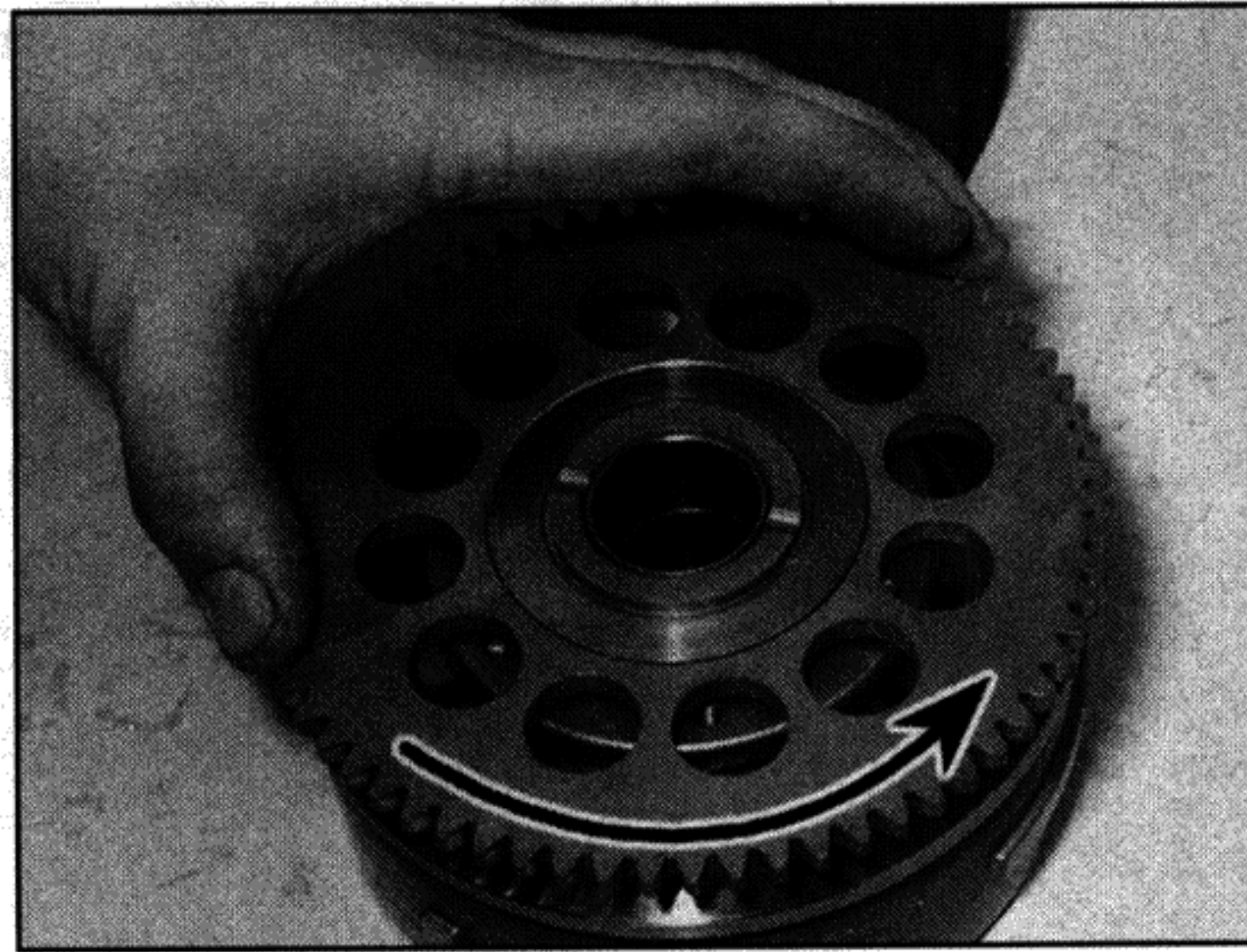
18.2 The gear should rotate freely in the direction shown
