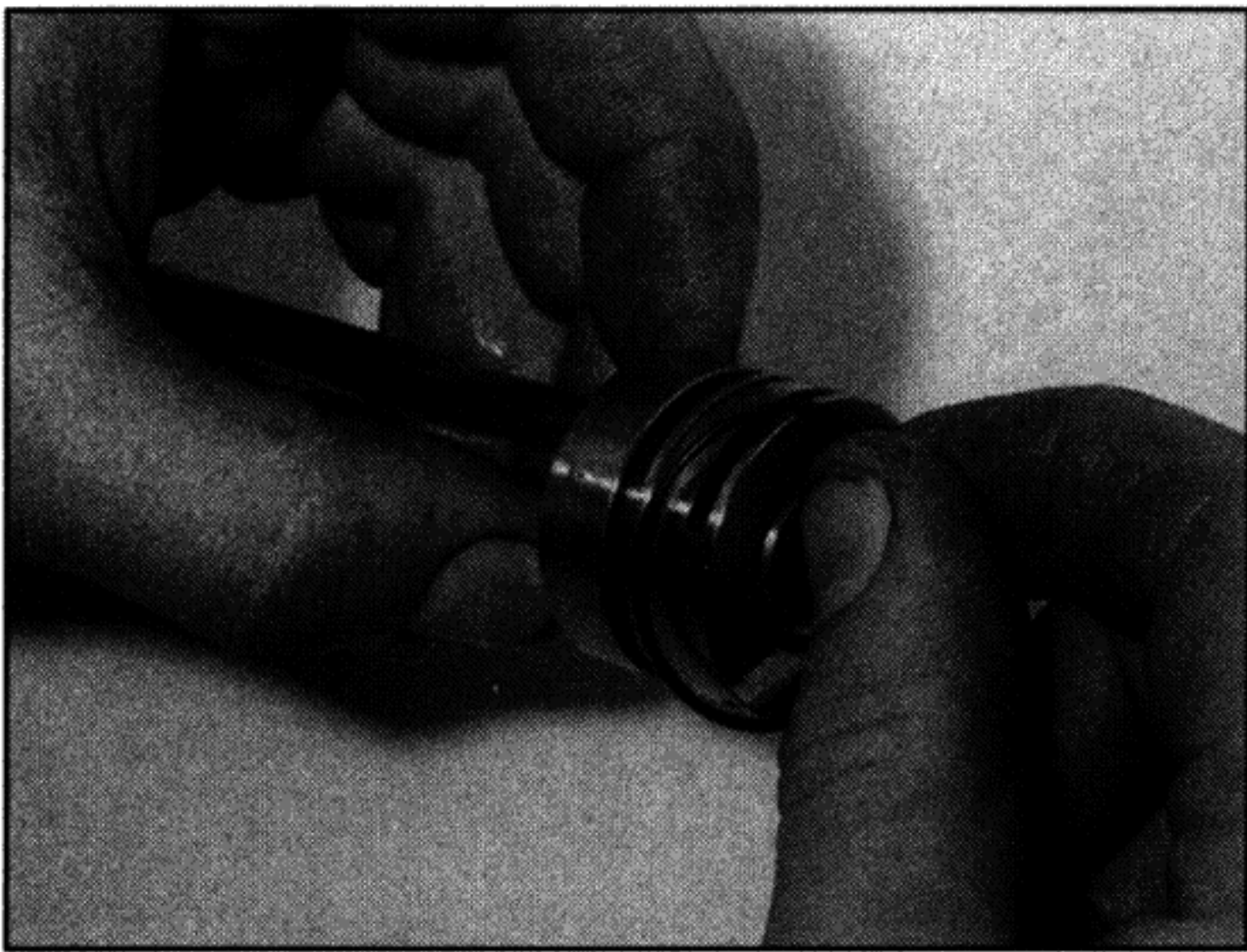
23.13a Fit a new O-ring into the narrow groove
