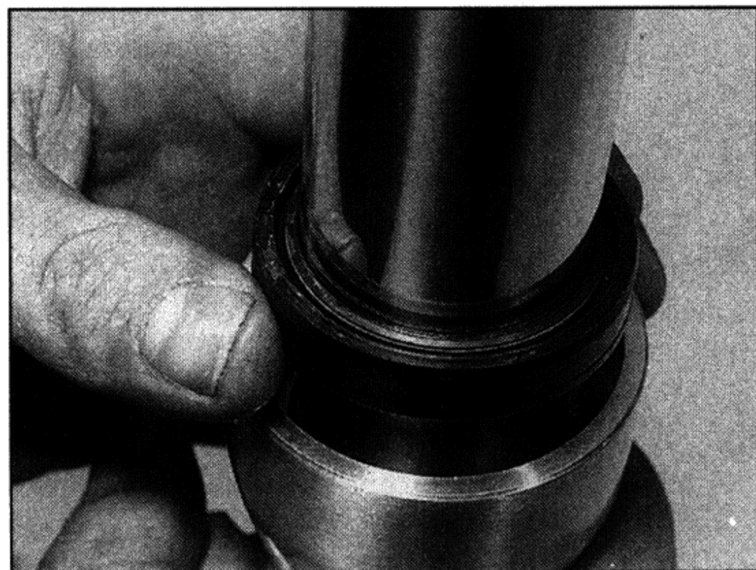
7.23 Make sure the oil seal is the correct way up
