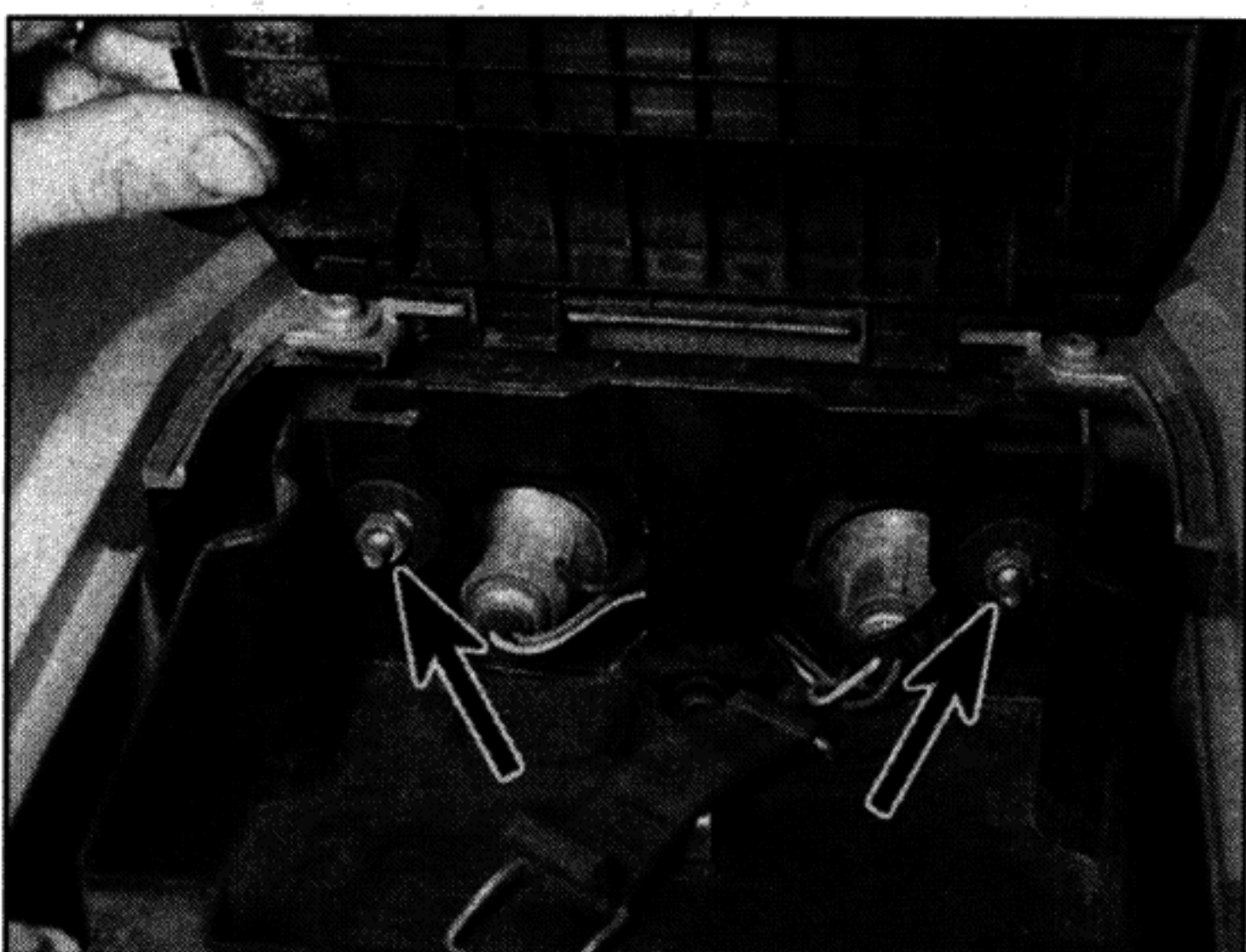
10.3b Tail light assembly nuts (arrowed) – XTZ models
