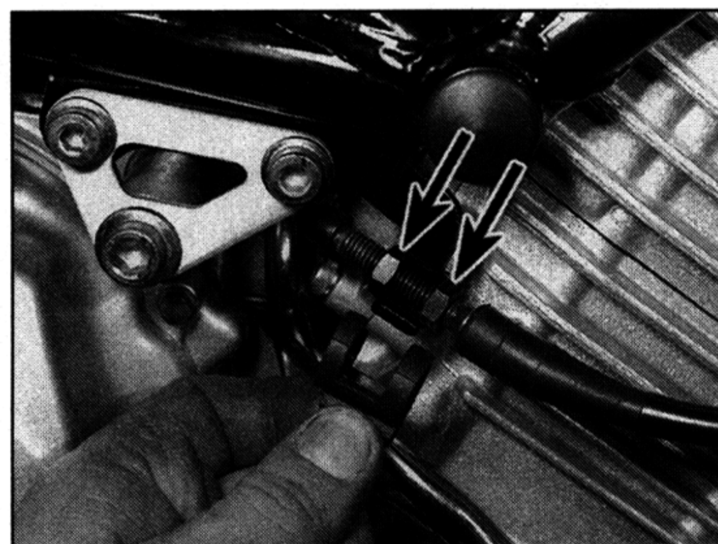
10.5a On TRX models, remove the cover and adjust the cable as described using the nuts (arrowed)
