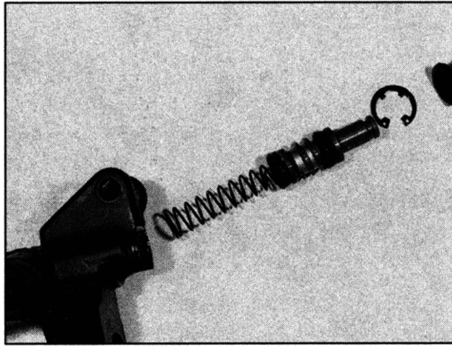
5.13b Lay out the internal parts as shown, even if new parts are being used, to avoid confusion on reassembly
