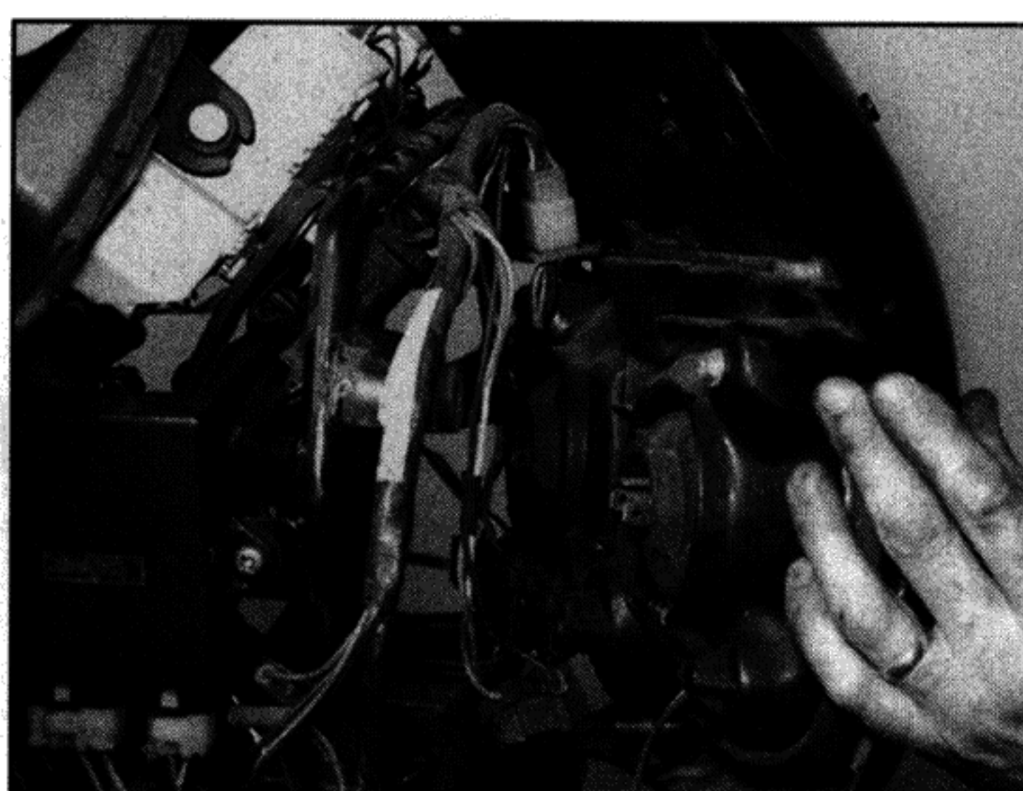
5.16 The headlight comes away with the fairing
