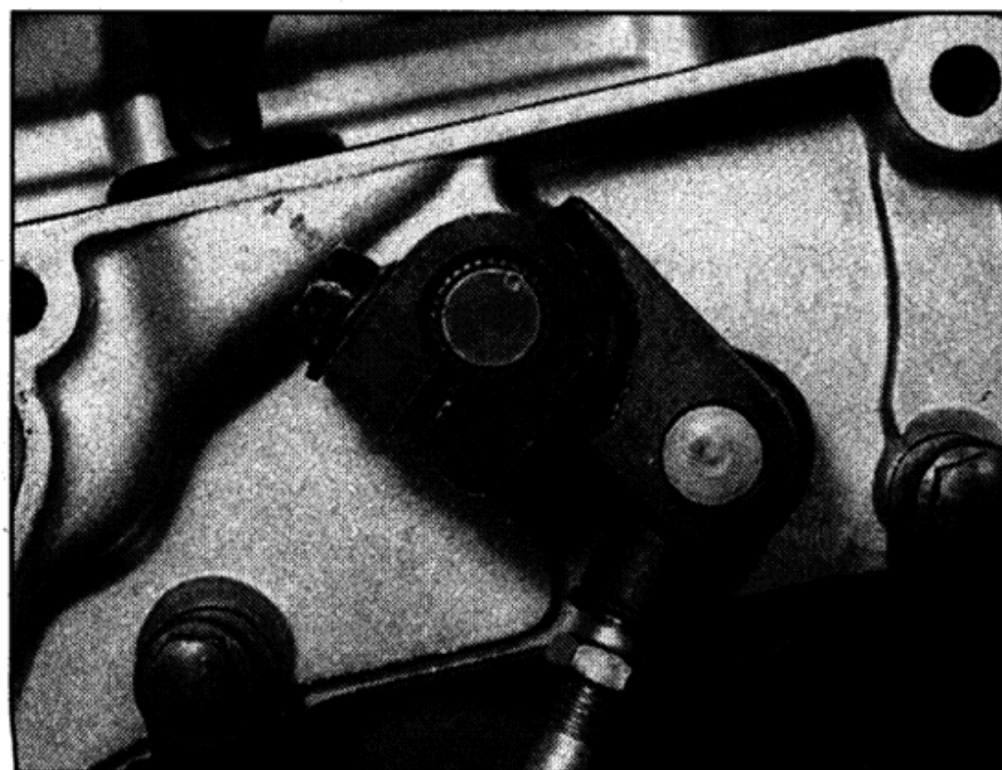
15.2b Linkage arm/shaft alignment – TDM models
