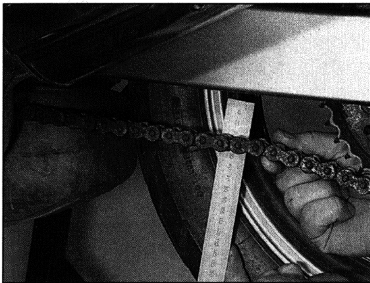
1.3 Push up on the chain and measure the slack
