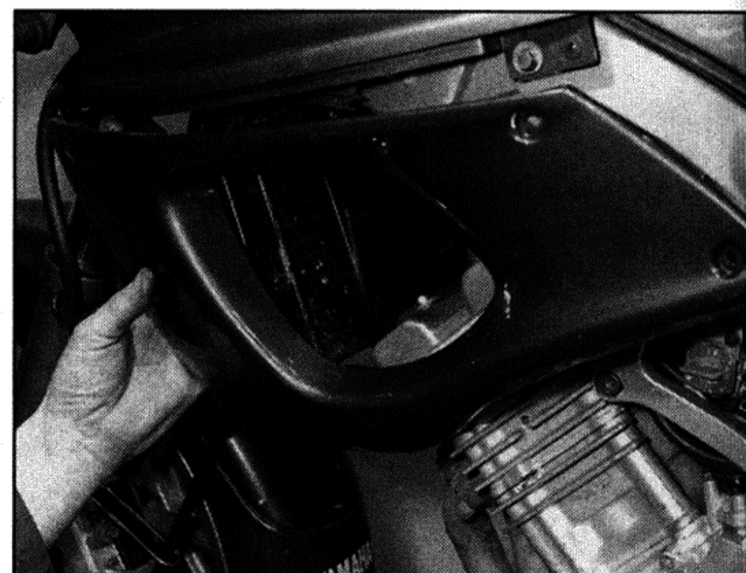
4.1b ... and remove the panel
