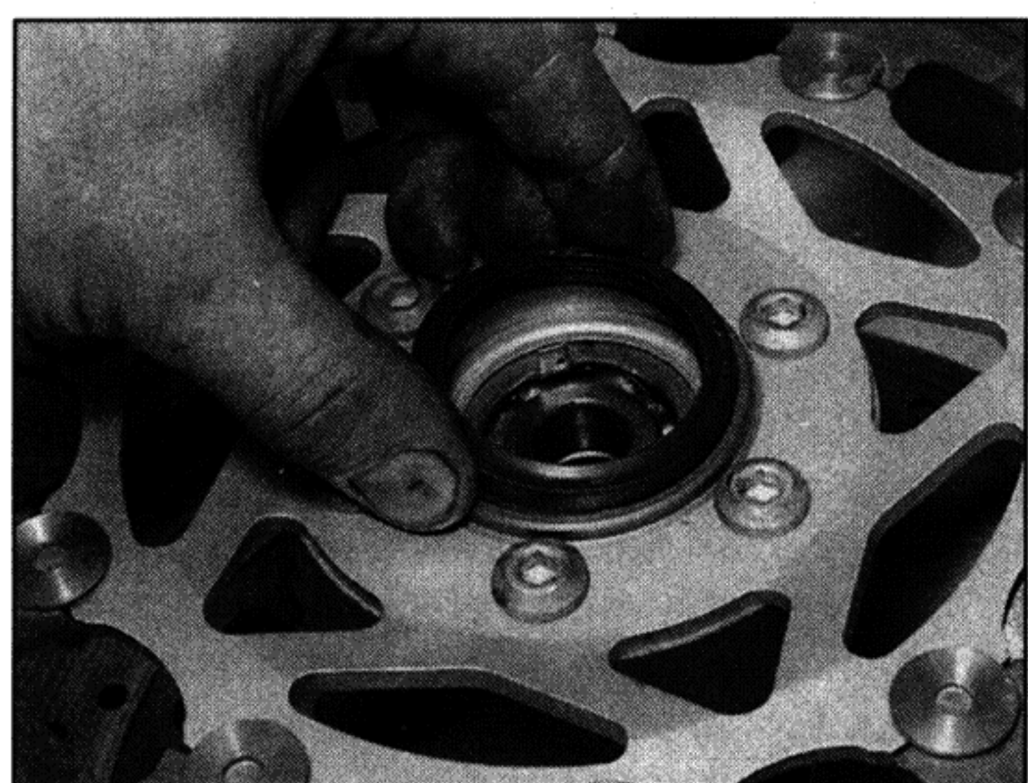
13.13 Press the grease seal into place
