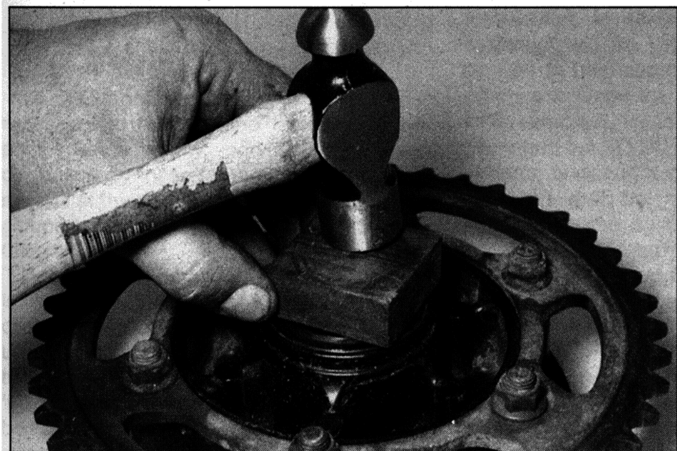
13.30a Fit the grease seal . . .
