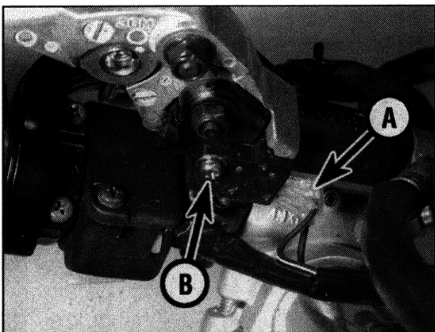
14.7b Front brake switch wiring connectors (A), mounting screw (B) – TRX models
