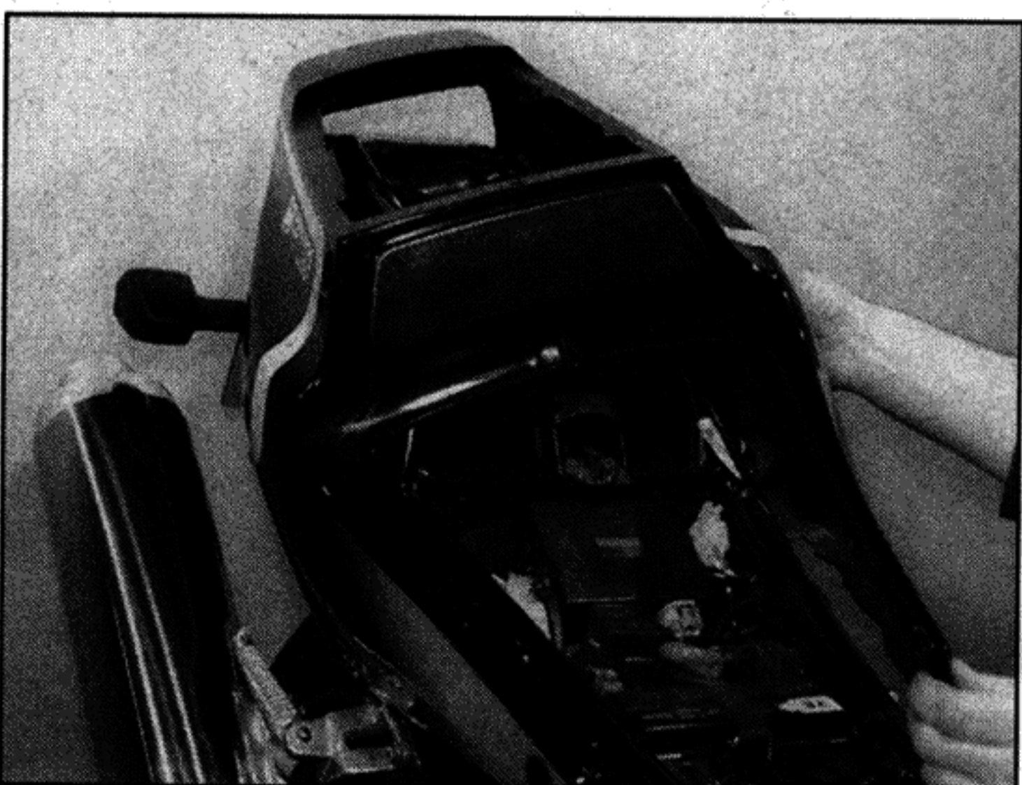
3.5b ... and remove the side cover assembly
