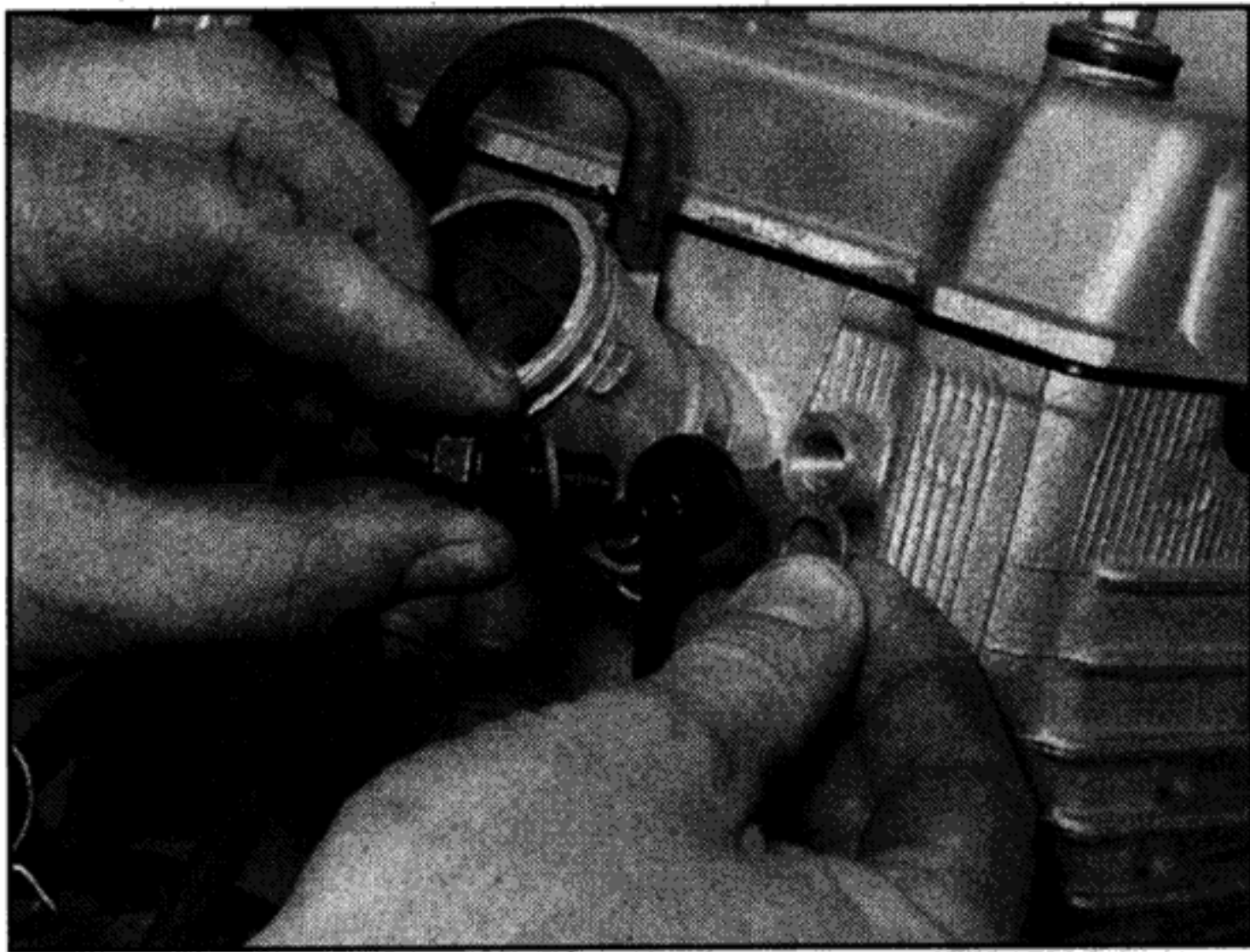
10.18a Use new sealing washers on each side of the union . . .
