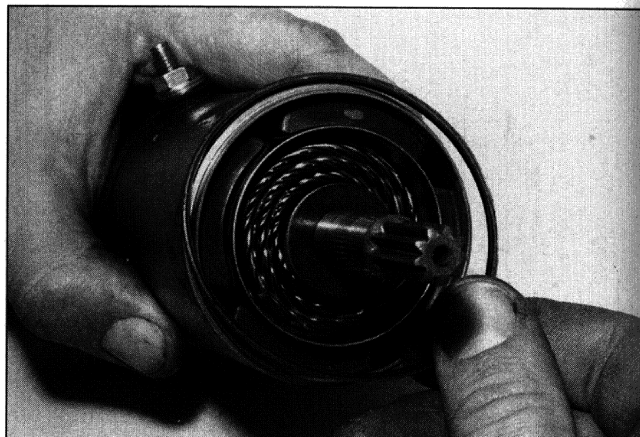
29.20a Fit a new O-ring onto the front of the housing . . .
