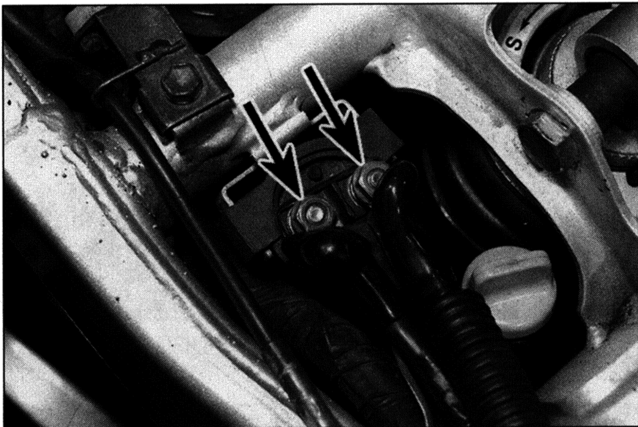
27.7 Pull back the covers to access the terminal nuts
