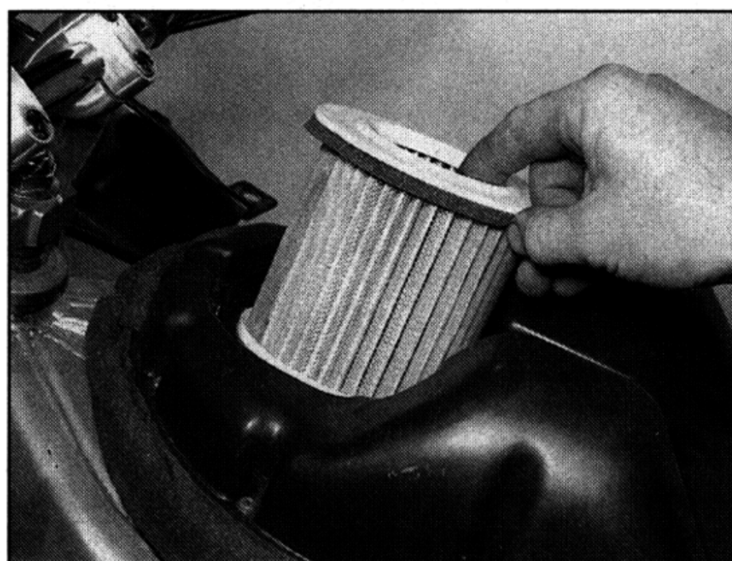
5.2b . . . then withdraw the element (TDM shown)
