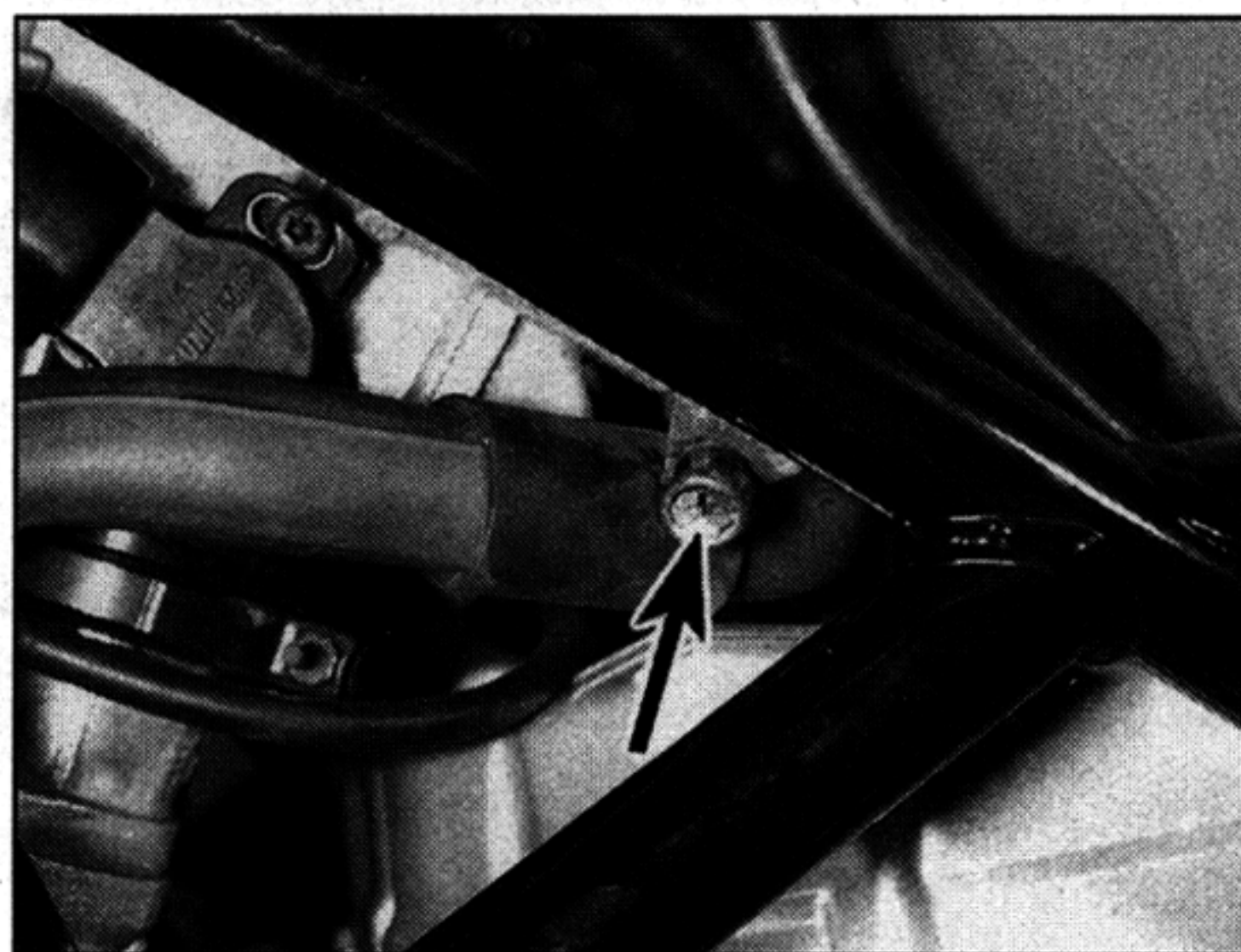
3.3b Idle speed adjuster screw (arrowed) – TRX models
