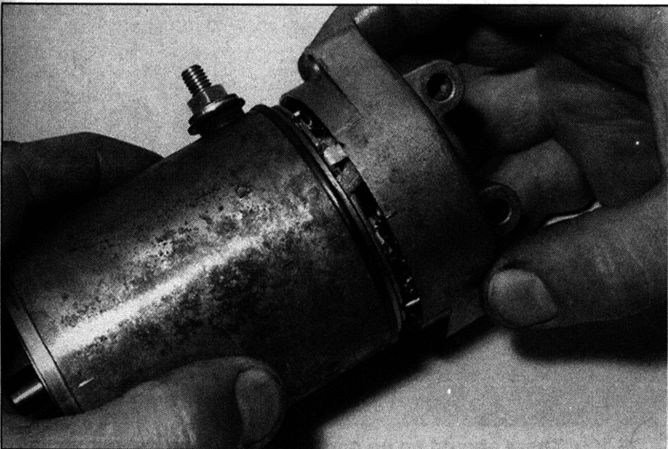
29.5a Remove the rear cover . . .
