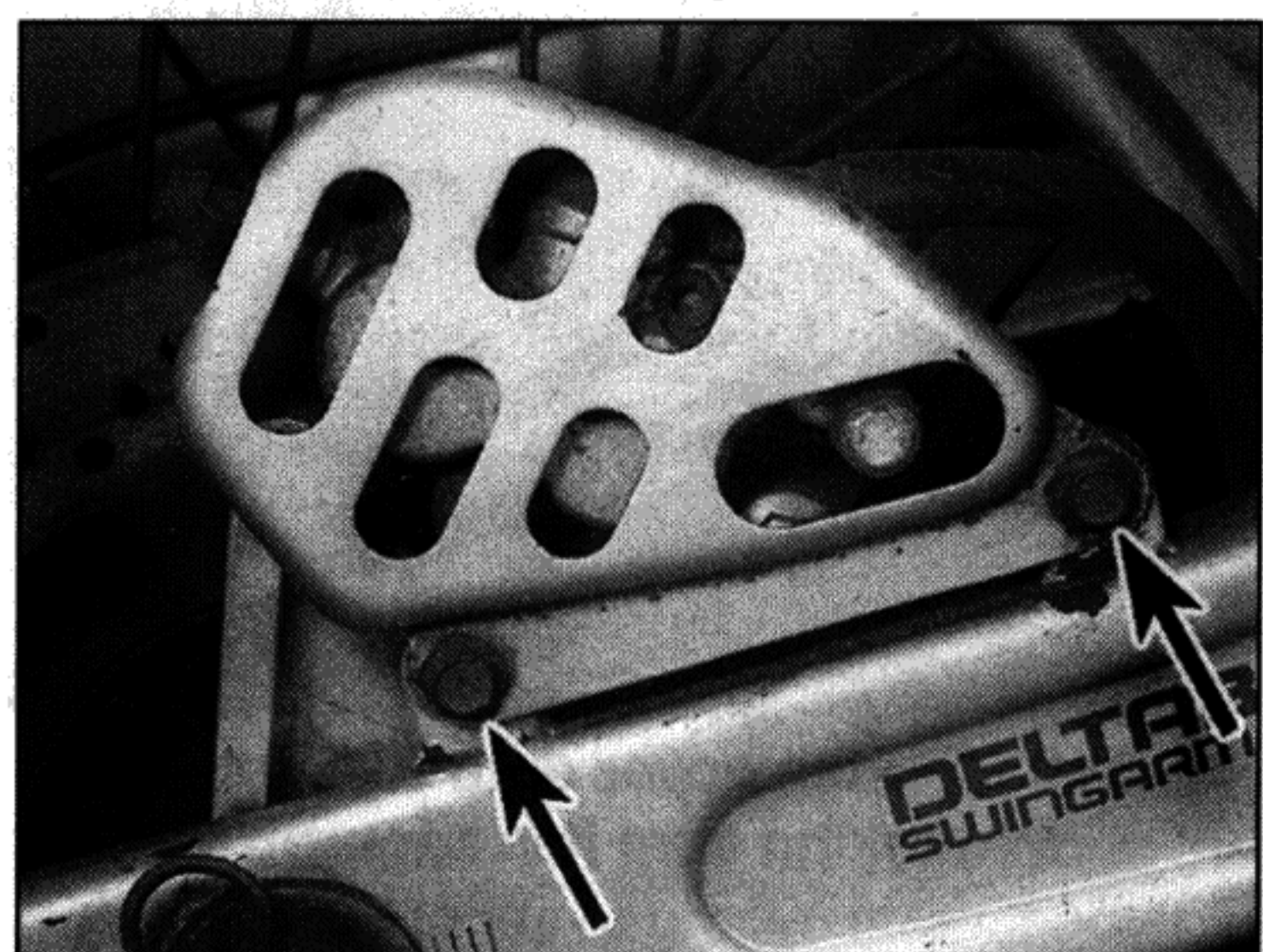
3.1 Unscrew the bolts (arrowed) and remove the shield
