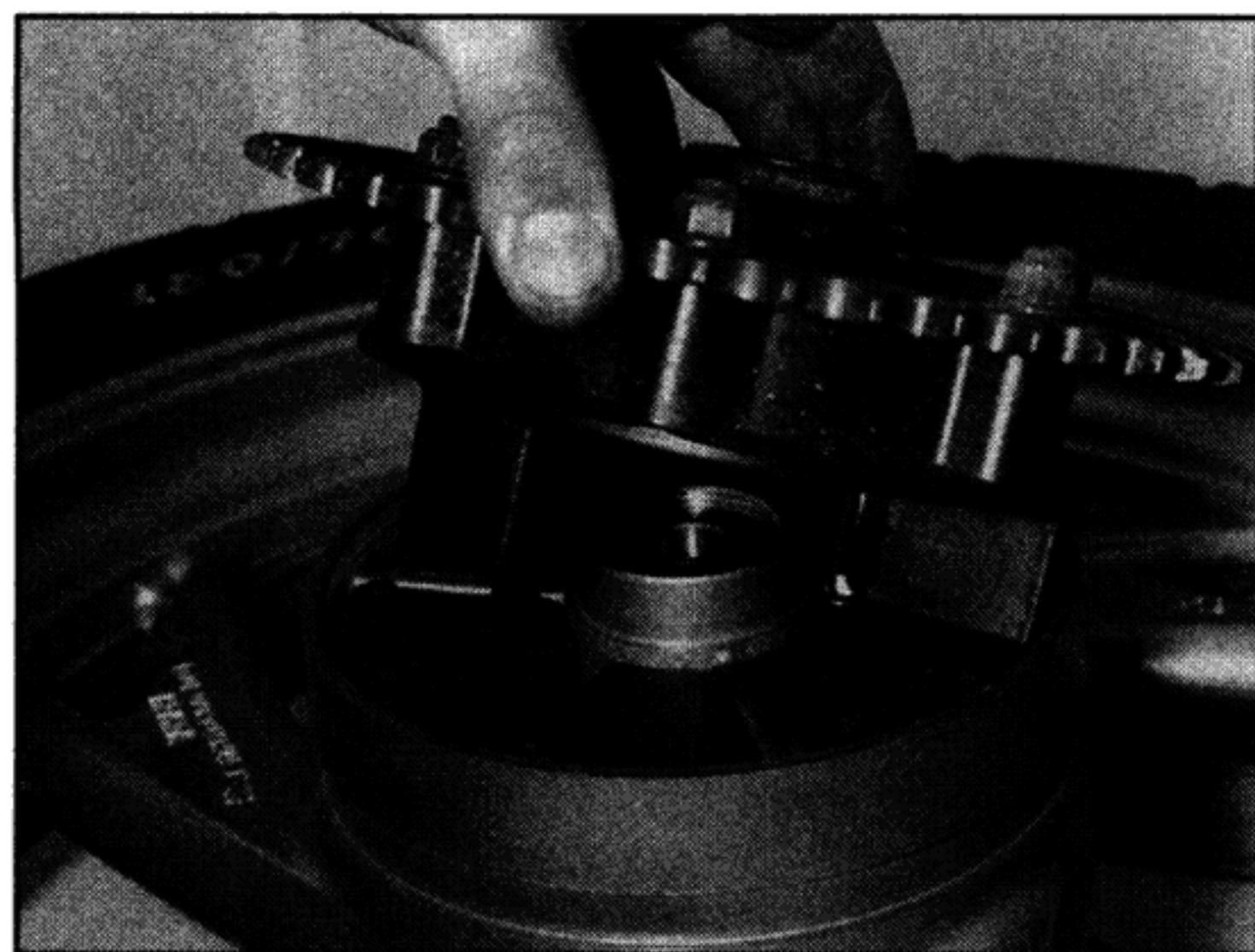
17.2 Lift the sprocket coupling out of the wheel . . .
