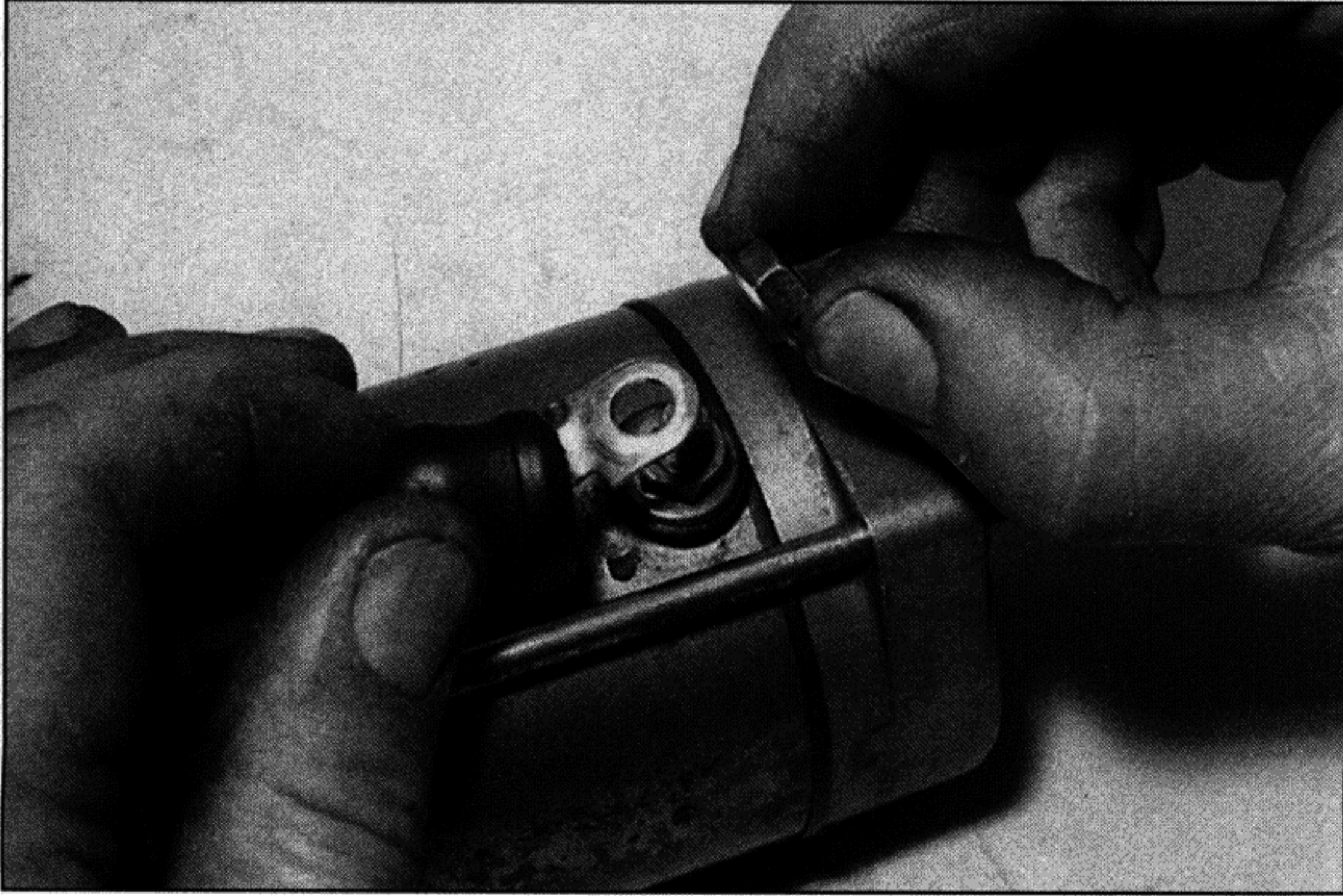
29.1 Unscrew the terminal nut and detach the lead
