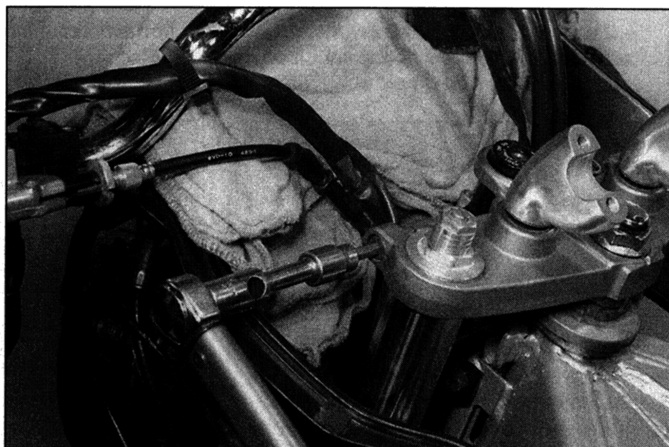
6.8 Tighten the various clamp bolts to their specified torque settings
