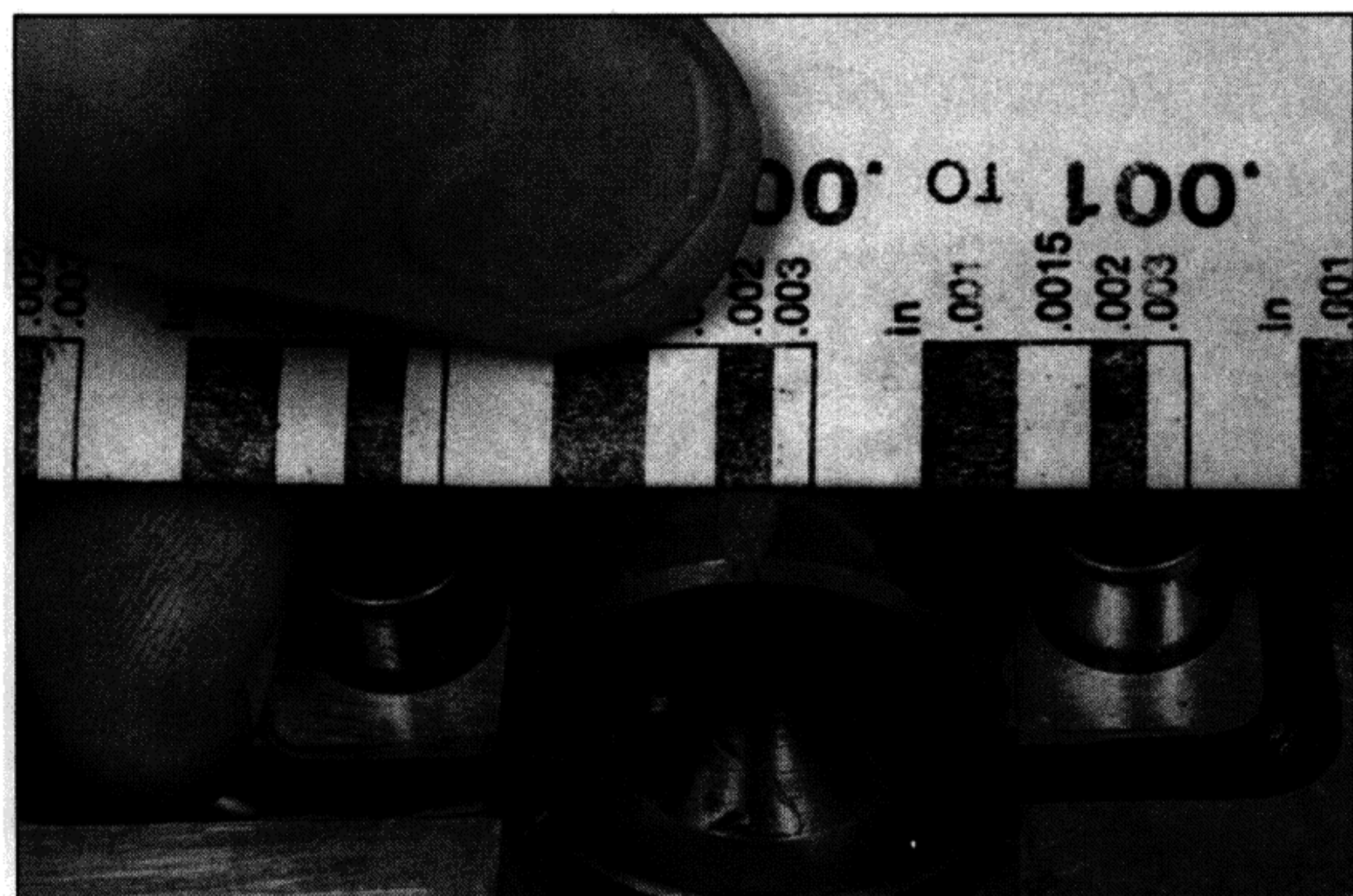
8.17a Compare the width of the crushed Plastigauge to the scale printed on the Plastigauge container
