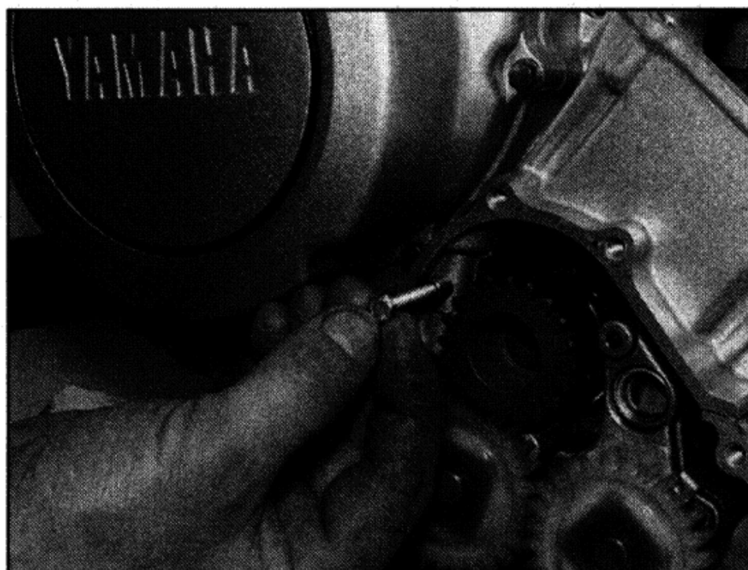
24.5b . . . then thread a 5 mm bolt into the head of the pivot pin . . .
