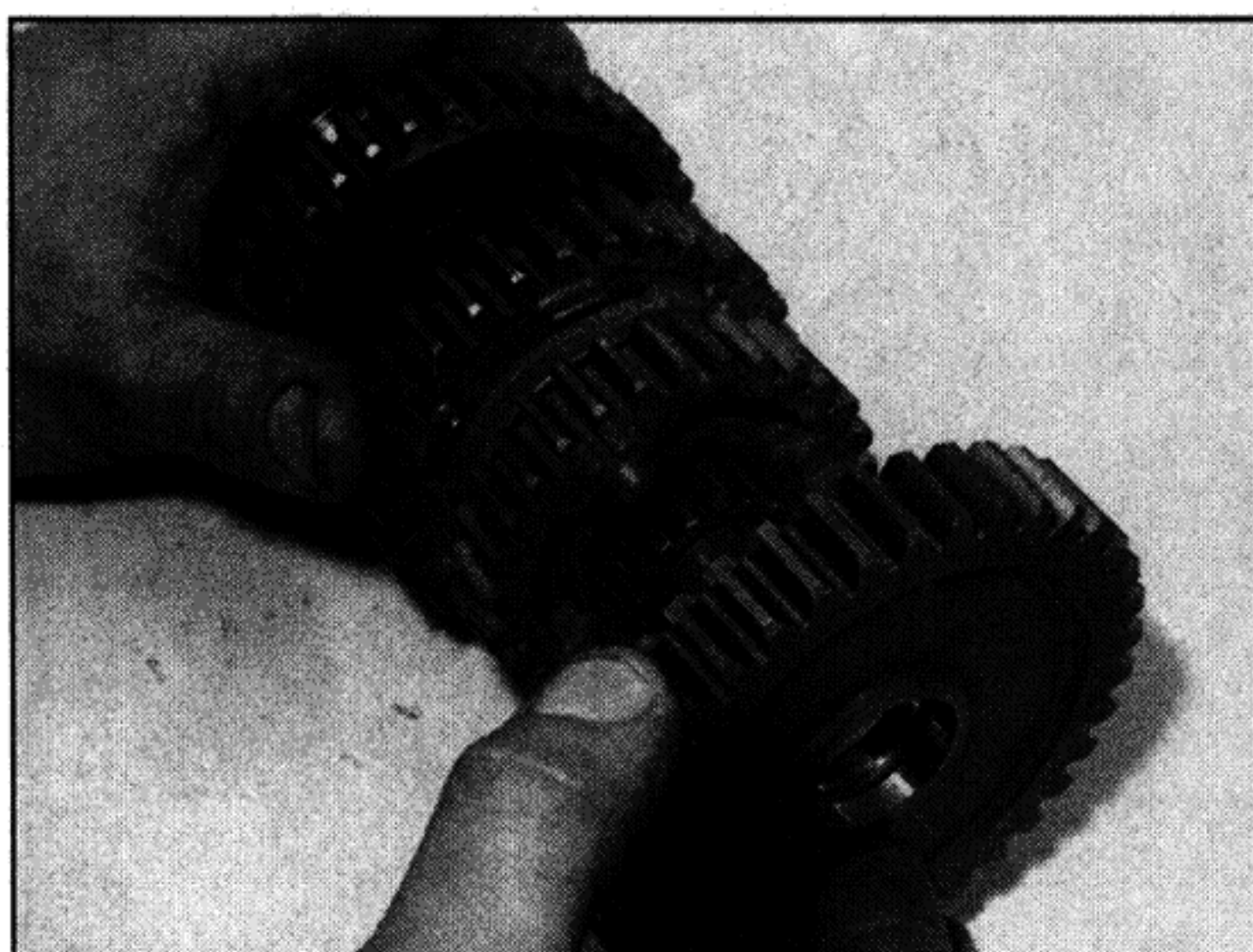
31.40b ... followed by the 1st gear pinion ...
