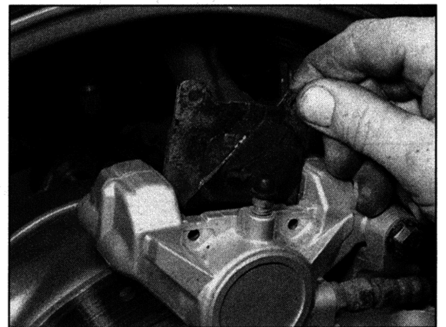
2.1e ... and lift out the pads
